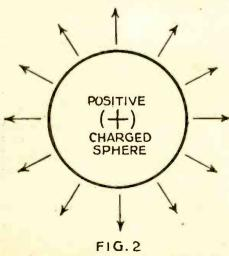
In the case of a charged sphere, the electric field extends equally in all directions.
