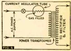
Current regulator used to stabilize power supply input voltage.
