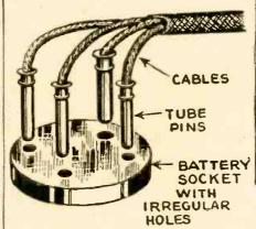
tube base as shown in the diagram. By removing the prongs and soldering the cable wires to them, you will have a flexible plug that will fit the irregular holes in a 1.4-volt battery pack.
