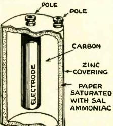
All you have to do is to secure one or two 1½ volt dry cells, large size (see drawing).
