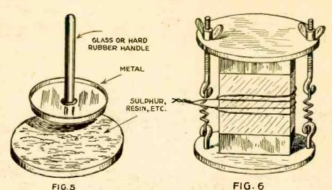
Fig. 5 shows the simple elements of an electrophorus, and the nature of the distributed charges. Fig. 6 shows a crystal of Rochelle Salts placed between clamps. As the winged nuts are tightened, even slightly, the charge set up in the crystals increases.
