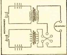
The wiring diagram for the sum-and-difference method of listening is simple and the mechanism is easily operated.
