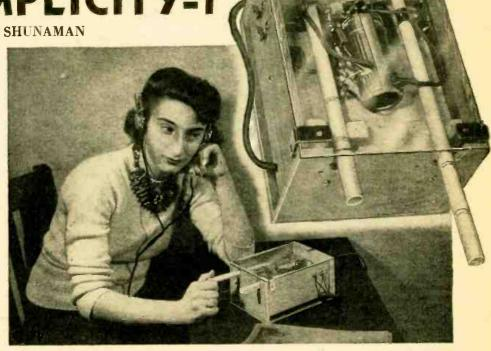
Tuning-up the all-electric model. The control being adjusted is the antenna tuner; the other one is the R.F. plate unit. Ventilation slots at the bottom of the receiver are easily discerned. Note glass cover on receiver.
