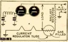
Current regulator tube stabilizes heater potential when A.C. supply fluctuates.
