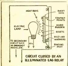
When the lamp is turned on it will be a matter of seconds before the heat from the lamp causes the strip of sheet iron to bend from its expansion. This causes the two contact points to touch and thus complete the secondary circuit. Its application is shown in the diagrams.—L. B. ROBBINS
