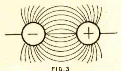
When oppositely charged spheres are brought together, the lines of force in the electric field created take the form shown.
