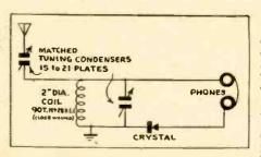
Simple crystal set. Two condensers tune both aerial and crystal circuits, thus permitting better separation of stations.
