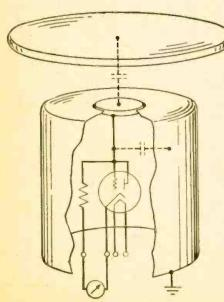
View showing tube acting as the large capacitance.
