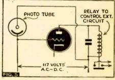
Phototube controls a relay circuit.
