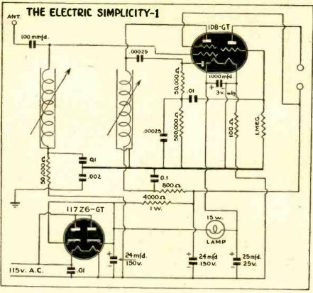
Schematic of the all-electric model. With proper ballast resistors, tubes such as the 25Z5 may be used instead of the 117Z6—GT. Note than an outside ground is used on this set, contrary to the usual A.C.-D.C. practice.
