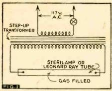
Basic circuit of the Sterilamp, the widely used
