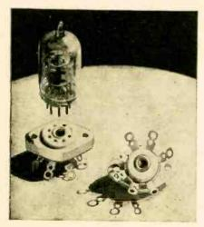
type, so they receive the tiny tube prongs without danger of fracturing the glass base of the tube.
