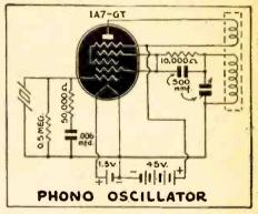
coil may be a broadcast coil from an old T.R.F. receiver, and the condenser should have a maximum capacity of from .00035 to .0005 mfd.
