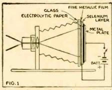
Sectional diagrammatic view of the camera which uses electrons to "get" the picture, and thus do away with "developing." The picture is ready just as soon as it is taken. Note the similarity of the components of the focal plane to the salenium photoelectric cell, but still a battery is required, which makes for some difference. Undoubtedly this device is the vanguard of similar developments which will take place in the next few years.
