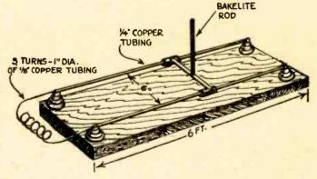
holding the rod to the copper shorting bar. The system should be kept in the clear and as far distant from surrounding stray fields and metal as is practicable under ordinary circumstances. The distances between nodes will represent half a wavelength.
