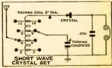
This circuit uses taps for aerial tuning and both taps and condenser in the crystal circuit.
