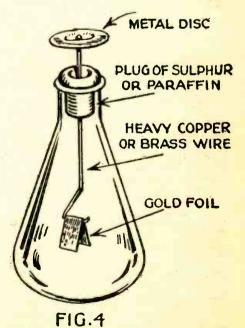
The constructional details of a home-made electroscope.
