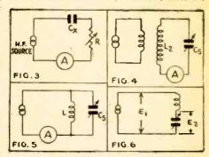
small diameter makes skin-effect changes negligible as frequency is varied, and for the same reason series inductance also varies only by a minute amount. The primary standard is a thermo-couple R.F. meter. Knowing the resistance of the wire (which is practically constant with frequency), and the current in it, the voltage s simply IR. A special separate heater type thermocouple is used. The inductive reactance of the wire is only 1-ohm at 100
