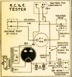
be calibrated in this way. Get several good resistors and find out their reading on the meter and fill in the rest by mathematics. meter and fill in the rest by mathematics. My power transformer was  $2\frac{1}{2}$  by 4 inches. The neon bulb is of the 2-watt type as all others will burn out.
