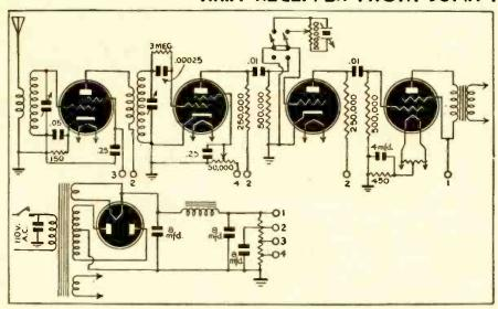
The circuit diagram shows a four-tube T.R.F. set for operation on A.C. only, which I built from salvage parts obtained from about four or five old sets.
