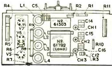
receptacle is provided for the dynamic reproducer; but magnetic reproducers connect instead to tip-jacks. The "B" voltages, which are disturbed when the dynamic reproducer field coil is removed from the circuit are equalized by load resistor R8; which is placed in shunt with the high voltage D.C. when the "link" is connected to the two binding posts shown at the upper right of the
