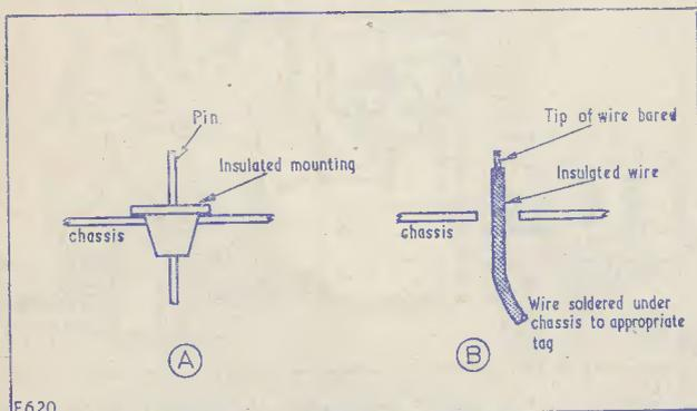
Fig. 76. Two typical test points
