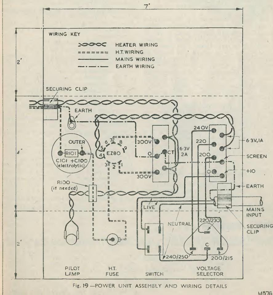
Fig. 19—POWER UNIT ASSEMBLY AND WIRING DETAILS
