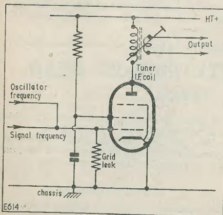
Fig. 69. The basic television tuner mixer circuit. Both signal and oscillator frequencies are fed to the common control grid
