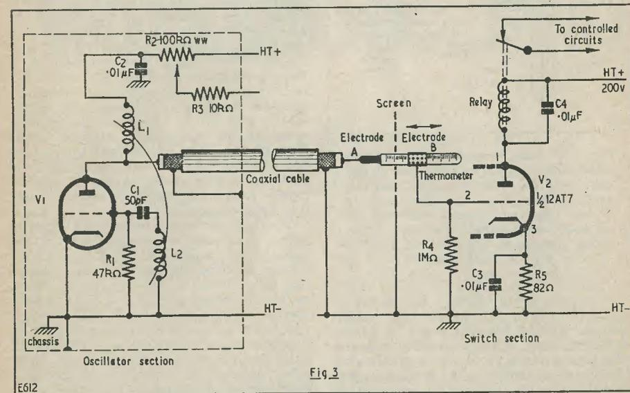
Fig. 3. A suggested circuit wherein the thermometer may operate a relay at predetermined temperatures
