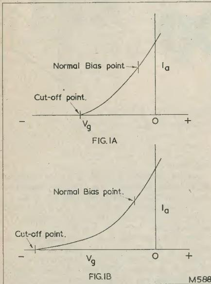
Fig. 1. Illustrating how two valves, which may behave exactly the same as amplifiers under normal biasing conditions, can have quite dissimilar cut-off potentials. The cut-off voltage in (b) is markedly further negative than that in (a)
