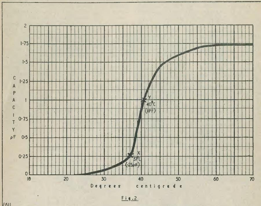
Fig. 2. Curve showing the capacity between electrodes A and B for bulb temperatures between 10 and 70° C
