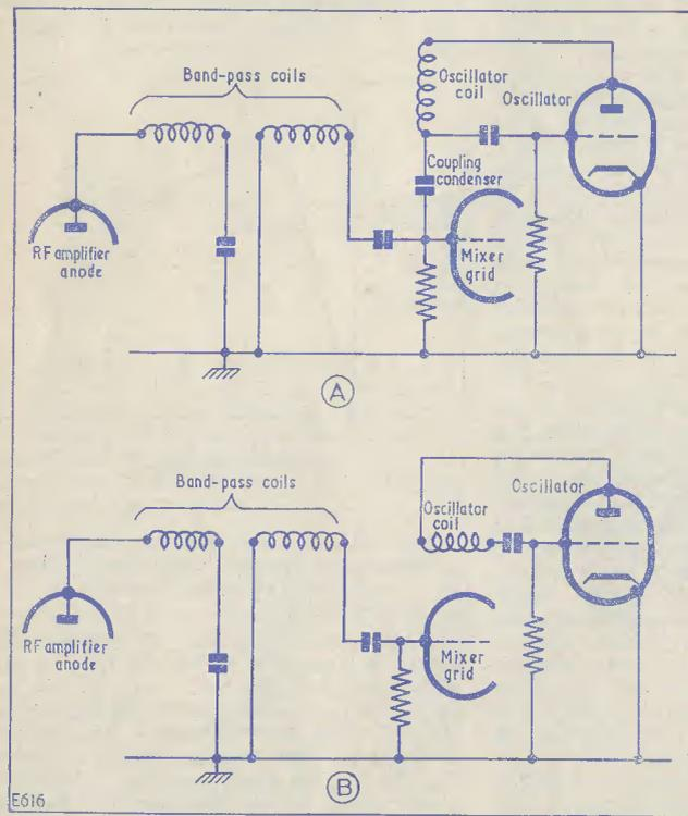
Fig. 71 (a) The oscillator voltage is frequently applied to the mixer grid via a coupling condenser, as shown here. The value of the coupling condenser usually lies between 1 and 3pF. (b) An alternative type of coupling. In this case the oscillator coil is mounted in line with the bandpass coils to obtain an inductive coupling
