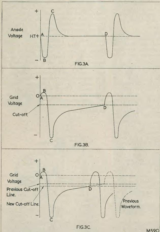
Fig. 3 (a) The anode voltage waveform of a typical blocking oscillator. (b) A blocking oscillator grid voltage waveform corresponding to the anode waveform of (a). (c) If the grid cut-off line is moved slightly, the length of the period from C to D, and hence the frequency of the oscillator, is considerably modified
