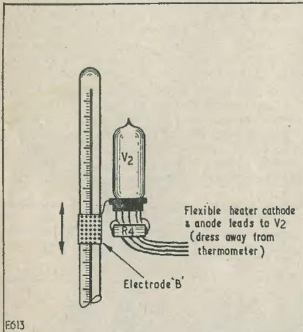
Fig. 4. In order to ensure a short connection between V<sub>2</sub> grid and electrode B, this valve may be mounted to the electrode itself, as shown here. The valve should be on the "high-temperature side" of the electrode. There should be no necessity to fit any components other than R<sub>4</sub> directly to the valveholder
