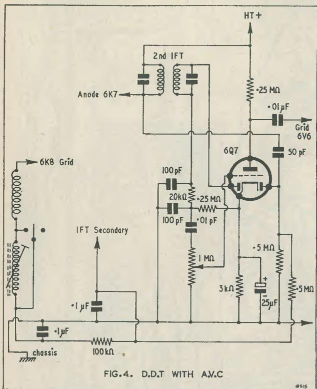
FIG. 4. D.D.T. WITH A.V.C.
