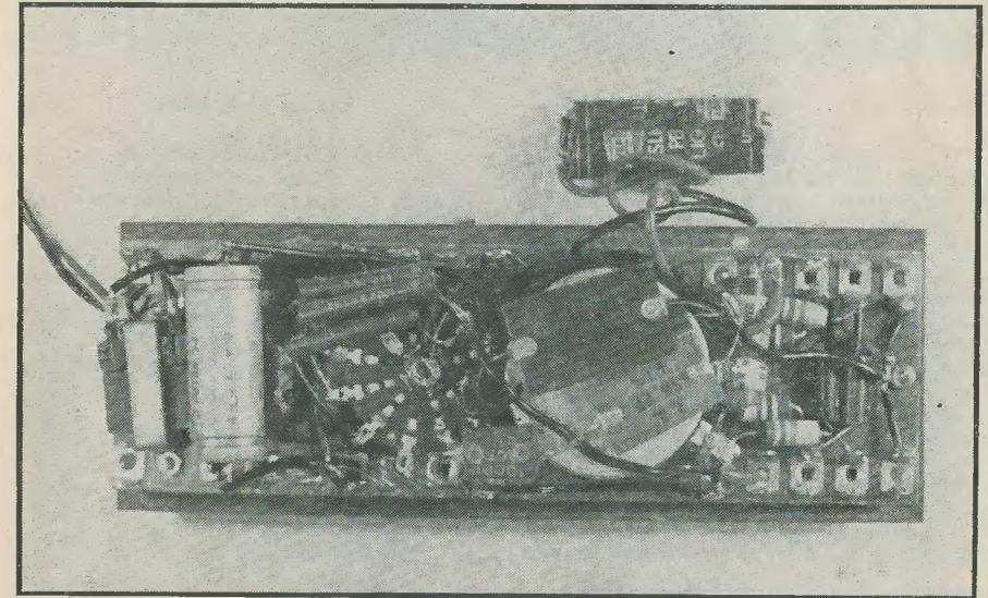
Below-chassis view of Transistor C-R bridge
