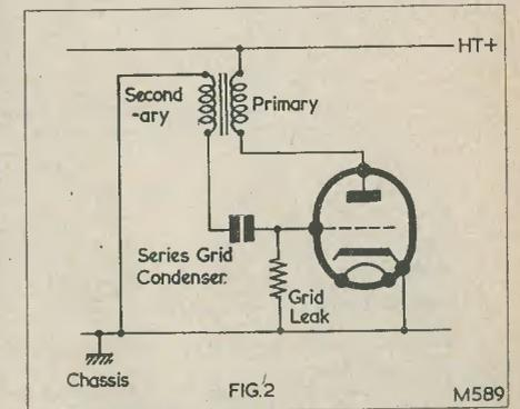
Fig. 2. A simple blocking oscillator. A control of frequency is possible by making the grid leak a variable component. Positive-going sync pulses may be applied to the grid, a possible method consisting of inserting a low value resistor between secondary and chassis, and applying the pulses to the junction of the resistor and the secondary
