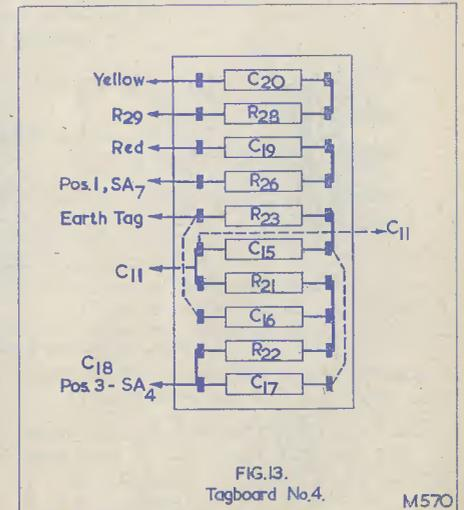
The end of  $C_{15}$  (47pF) on tagboard No. 4 nearer to the erase head socket should be connected along the path shown in Fig. 16 to the end of  $C_{11}$  (0.1 $\mu$ F) on tagboard No. 3 furthest from the  $V_3$  valveholder. The junction of  $C_{17}$  (47pF) and  $R_{22}$  (56k $\Omega$ ) on tagboard No. 4 should be connected to position 3 of switch section  $SA_4$ . From position 1 of switch section  $SA_7$  run a lead to the nearest, or free, end of  $R_{26}$  (4.7k $\Omega$ ).
