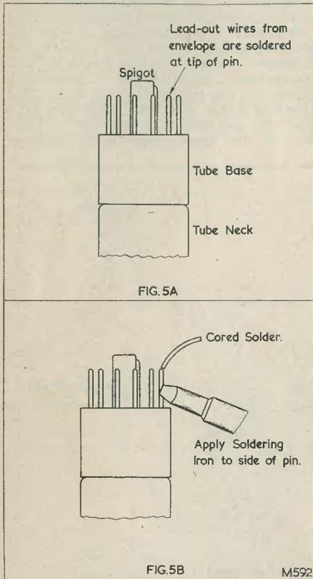
Fig. 5 (a) Open-circuit connections to cathode ray tube elements occasionally occur at the point where the lead-out wire from the envelope is soldered to the pin. (b) Where such open-circuits occur they may frequently be cleared by applying a little active, but non-corrosive, flux to the tip of the pin, carefully laying the soldering iron along its side, and allowing a little cored solder to melt and run down the inside of the pin
