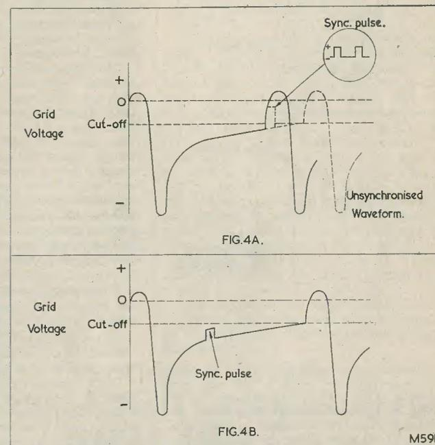
Fig. 4 (a) When a positive-going sync pulse is applied to the grid of a blocking oscillator, its leading edge causes the grid to pass the cut-off line and initiate the next cycle before its natural time. (b) If the sync pulse arrives too early, as happens here, the grid voltage does not pass the cut-off line, and the oscillator continues to run at its natural frequency
