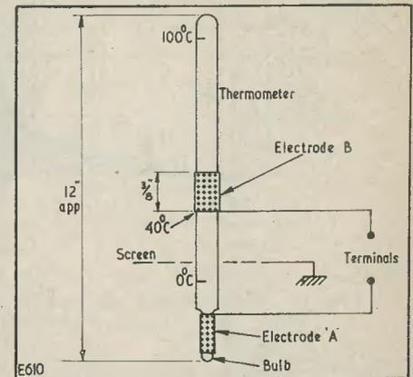
Fig. 1. The dimensions of the thermometer and electrodes used in the initial experiment
