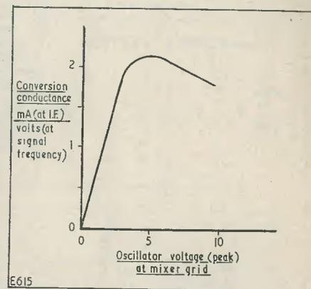
Fig. 70. A curve showing conversion conductance against oscillator voltage applied to the grid of the mixer
