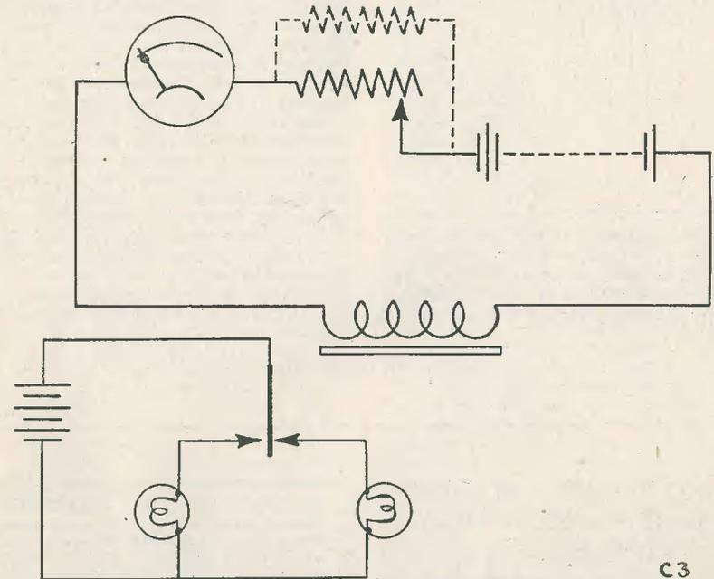
Fig. 3. Relay test circuit; the resistor shown in pecked line may be inserted to improve sensitivity (see text)
