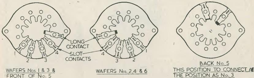
ALL SWITCH CENTRES IDENTICAL EXCEPT 5 WHICH HAS A WIPER ON THE BACK
