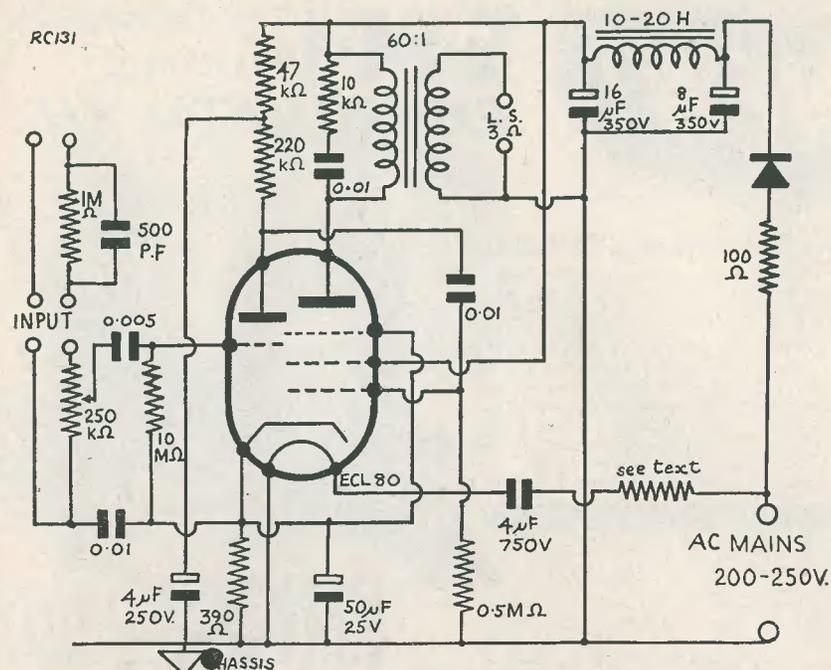
FIG. 1 CIRCUIT OF SIMPLE VALVE AMPLIFIER
