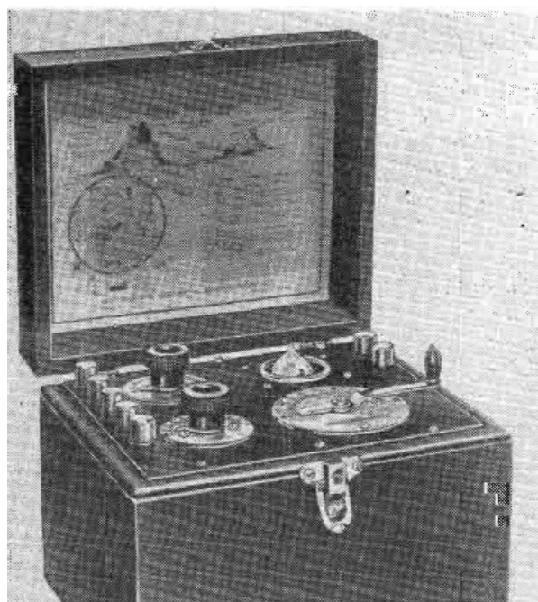
The Aeriola Senior, Westinghouse's one-tube set using the WD-11 tube, went on the market in the early twenties. It ended the reign of the crystal receiver.
