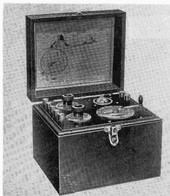
Radio took a man's size step forward in the early twenties when the Aeriola Senior, a one tube set using the WD-11 tube, was placed on the market. This receiver ended the reign of the crystal receiver.
