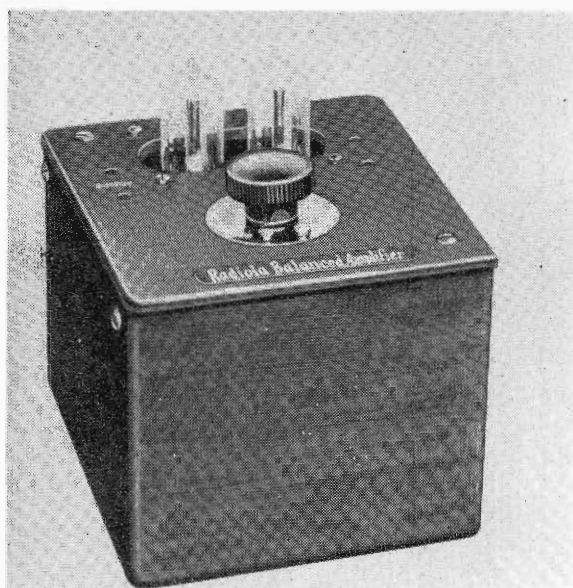
Development of this battery-operated two-tube amplifier in the early twenties made it possible to add a loudspeaker to the tuner so that the entire family could enjoy programs without headphones.
