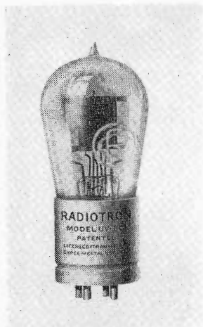
Almost all early radio sets using tubes relied on the UV-201 Radiotron for reception of the few stations operating in the early twenties.
