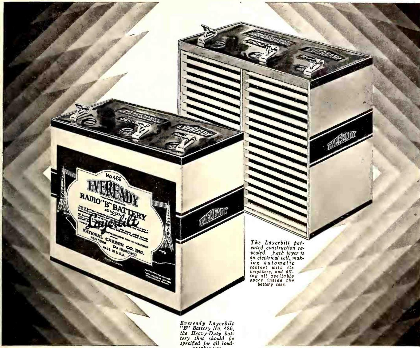
The Layerbilt patented construction revealed. Each layer is an electrical cell, making automatic contact with its neighbors, and filling all available space inside the battery case.
