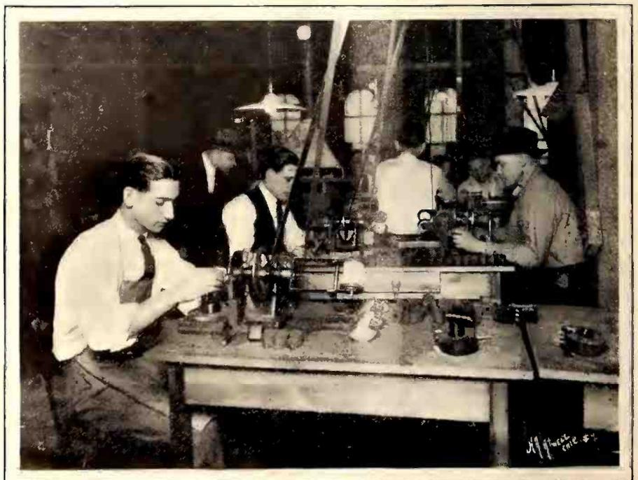
In the foreground is one of the machines used in winding primaries and interiors of torostyle coils. Finished primaries are seen under the spool of wire, while to the right are a few of the finished coils. Special machinery had to be developed for winding this type of coil, as explained in the article
