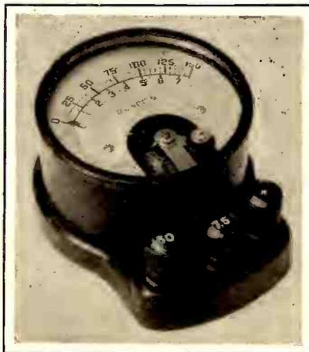
**A** DIRECT-CURRENT voltmeter, a portable instrument designed especially for use with radio receiving sets and known as type DO-3, shown above, has been introduced by the General Electric Company. The instrument has a double scale, 0-7.5 and 0-150 volts, which combinations are most suited for measuring filament and plate voltages ("A" and "B" batteries).
