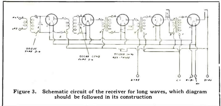
Figure 3. Schematic circuit of the receiver for long waves, which diagram should be followed in its construction
