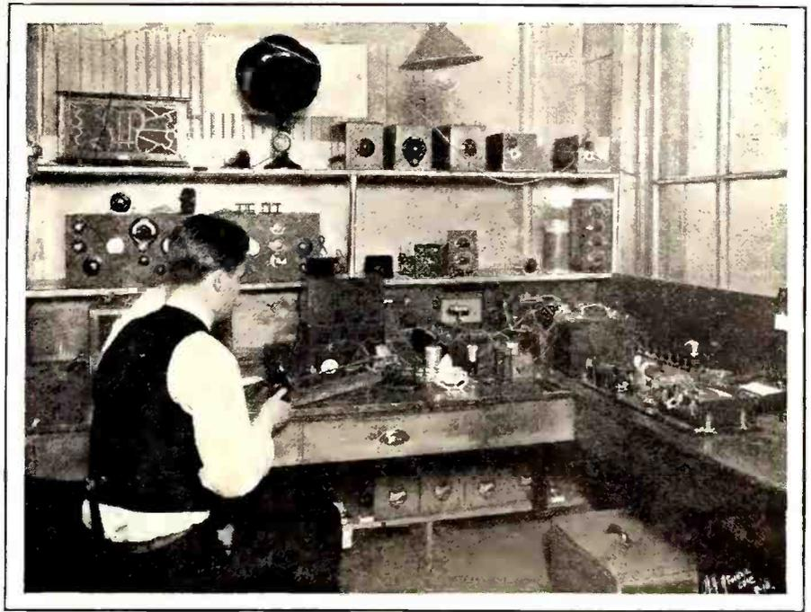
Here is a corner of the experimental laboratory where measurements on condensers and inductances are made. It is also here where preliminary tests are run on all apparatus before the company commits itself to the manufacture of a new article
