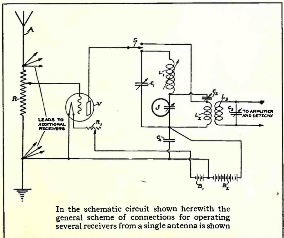
In the schematic circuit shown herewith the general scheme of connections for operating several receivers from a single antenna is shown
