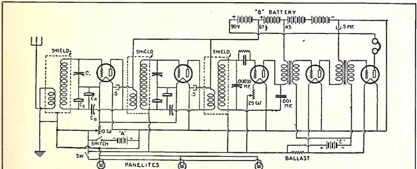
Fig. 2. Here is the isofarad circuit employing an all-capacity bridge to balance out the capacity coupling between the tube elements, and the "canned coils" which have all the power of the solenoids combined with the non-spraying qualities of the toroids.
