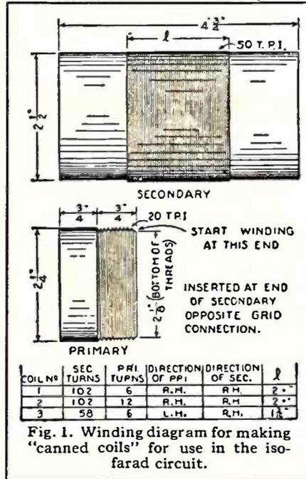
Fig. 1. Winding diagram for making "canned coils" for use in the isofarad circuit.
