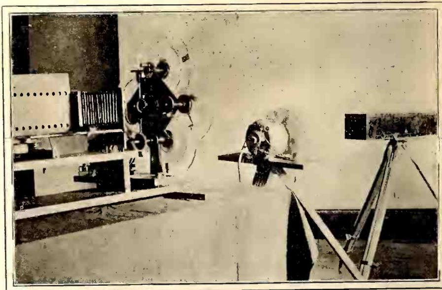
Radio Photo sending machine, lamp house to the left (for illuminating the picture); (2) four Prismatic Rings for moving the picture over the (3) light sensitive cell in the box at the right; time for each picture three minutes; distance limited only by power of the broadcasting station
