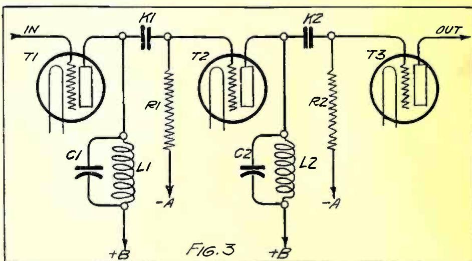
the leaks to the grid from the negative pole of the "A" battery, and the required amount can be obtained by adjusting the leaks until the proper bias is found by experiment. It should be noted that the leaks are an indispensable proposition in this sort of circuit and that they must be carefully fitted to the tubes for maximum results. The stopping condensers (K1) and (K2) are not critical.
