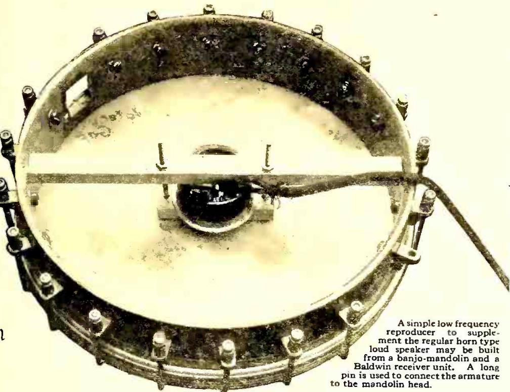
A simple low frequency reproducer to supplement the regular horn type loud speaker may be built from a banjo-mandolin and a Baldwin receiver unit. A long pin is used to connect the armature to the mandolin head.
