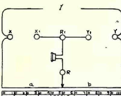
SCHEMATIC DIAGRAM OF THE BRIDGE CIRCUIT.
