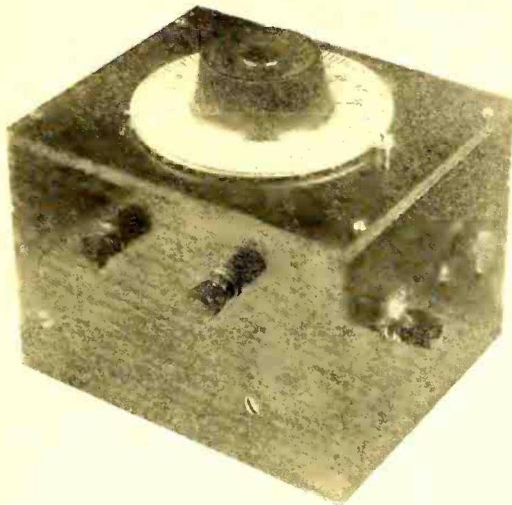
THE slide wire bridge described in the February issue of RADIO AGE has proven itself so popular and of such an asset to set builders and experimenters that, in answer to numerous requests, the writer has completed an improved model of this instrument, wherein the construction has been so simplified as to bring it within reach of the most inexperienced novice and yet retain the accuracy and ease of operation so necessary in an instrument of this kind.
