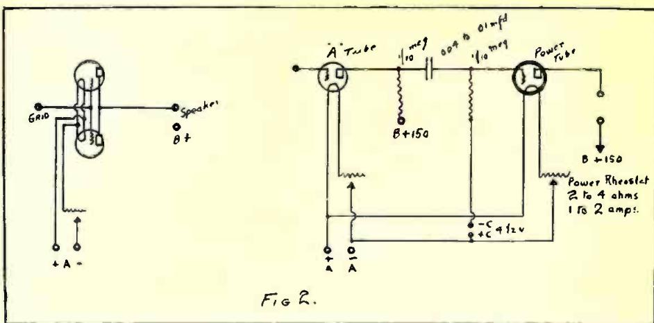
Fig. 2.—To prevent overloading of the last audio tube, a heavy power tube may be employed, or as an alternative nearly as good, two tubes may be operated in parallel.
