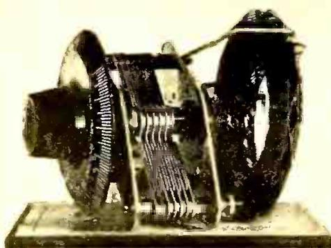
A rear view of the tuner for Mr. Hopkins' portable set, showing the method of mounting the coils on the back of the condenser.
