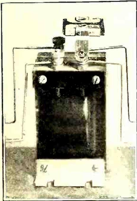
If you're annoyed by squeals in your set, maybe it's the fault of your amplifier. If so, here's a sure cure. If the second step of your audio amplifier causes a high pitched squeal that doesn't seem logical, eliminate it by placing a .00025 fixed condenser across the secondary of the transformer. This should not only eliminate the squeal, but should improve the quality of your reception as well. The photo shows how to place the condenser on the A. F. transformer.
