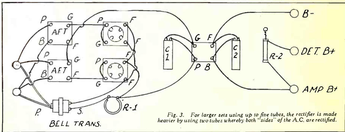
Fig. 3. For larger sets using up to five tubes, the rectifier is made heavier by using two tubes whereby both "sides" of the A.C. are rectified.
