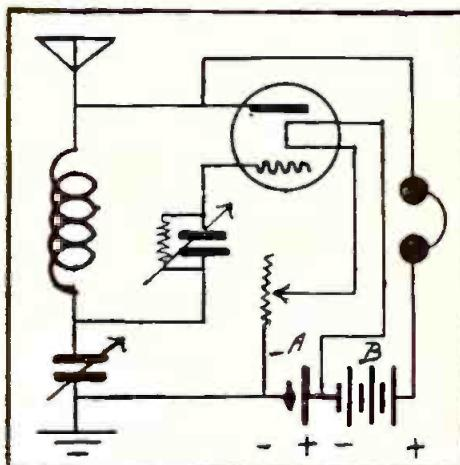
Here is another of the hookups built with the "\$1.00 circuit" by Mr. Perry. This hookup differs from the one shown on Page 7 in that only one coil is used. This arrangement insures excellent long-distance broadcast reception.
