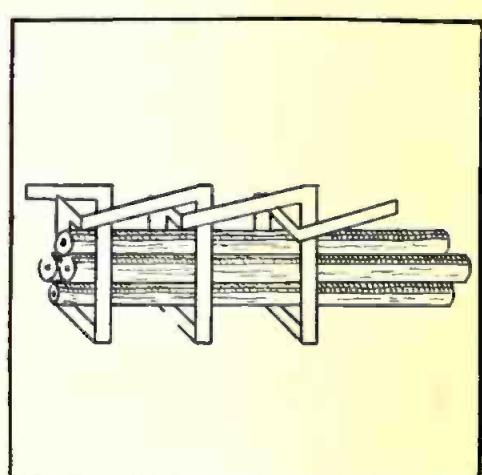
The above illustration shows the method of binding the wires in the cable together.
