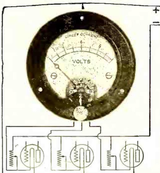
The above picture shows a voltmeter arranged to enable one to read the filament voltage on three separate groups of tubes. This is accomplished by means of the small switch located at the bottom of the meter.
