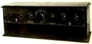
Here is the "Thermiodyne," the new six-tube wonder set manufactured by the Shepard-Potter Company of Plattsburg, N. Y. The feature of the Thermiodyne is its simplicity of control, all tuning on the entire six tubes being manipulated by the one control in the center. Great demand for the Thermiodyne is reported by the manufacturer.
