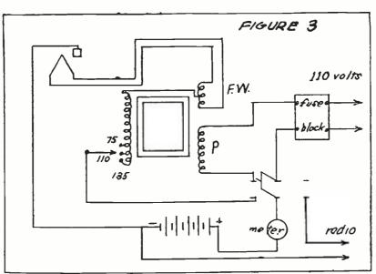
Figure 3. The wiring diagram of the home-built rectifier. ted to the plate and a fashion, it is only necessary to throw the switch from side to side to have the is steady stream from fila-battery on charge or discharge. Quite simple, fans.
