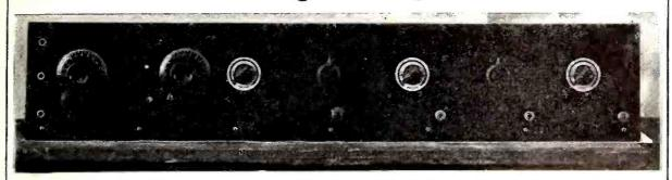
This figure shows the panel arrangement for separate control of each of the fundamental circuits. Instead of complicating matters, this control system actually makes the operation of the set much simpler.
