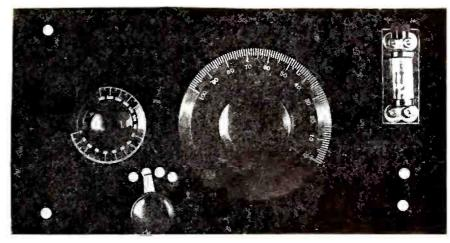
A front panel view of the beginner's crystal receiver, showing the simplicity of the panel layout.
