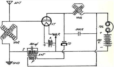
The "Bought Components Receiver" submitted by one of our British Dial Twisters. He says that he does exceptional work on this reflex circuit, which can be constructed from parts available at any radio store. The circuit is designed with the idea of not requiring any special parts.
