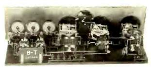
The new Bremer-Tully "Nameless" Low Loss receiver, one of the features of recent radio shows. This hookup consists of five tubes and its success is said to have given added impetus to the "low loss" craze now spreading among American and European radio fans. Note the simplicity and clear cut method of construction
