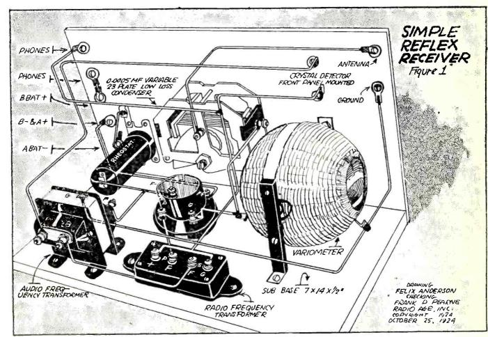
A perspective drawing of the simple single tube reflex, showing the simplicity and the lack of complication in its construction. The tube is made to do the work of both radio and audio frequency amplification, while the crystal detector gives exceptionally beautiful signal quality. The set is an ideal receiver for those "bugs" who wish to operate local stations on the loud-speaker.
