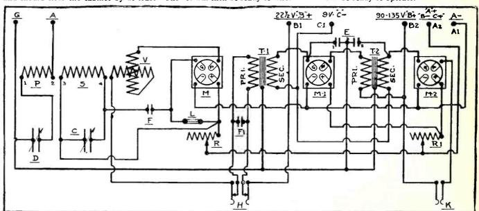
Fig. 3. A schematic circuit diagram of the three tube super-power receiver that reduces static and other outside noises to a mini-n. The construction and operation is fully described in the accompanying article.
