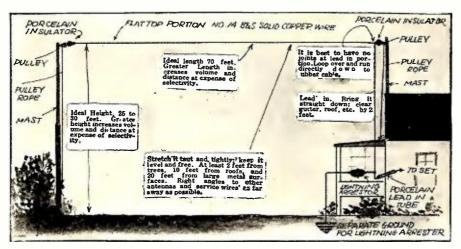
A photo-diagram showing the ideal dimensions for the antenna to be used on any average broadcast receiving set. If the instructions printed on the diagram are followed religiously, the listener can expect very good results from practically any receiver he tries out.
