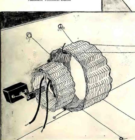
An illustration showing the assembly and mounting of the anode and feedback coils. The feedback coil is variable with respect to inductive relation to the plate will.
