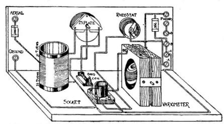
A perspective sketch and wiring diagram of the regenerative receiver contributed by turns close together, our technical editor, Mr. Frank D. Pearne. This set, with the exception of the coupler, uses standard parts, and can be easily assembled. From reports on this circuit, we are led to believe that it is exceptionally efficient.
