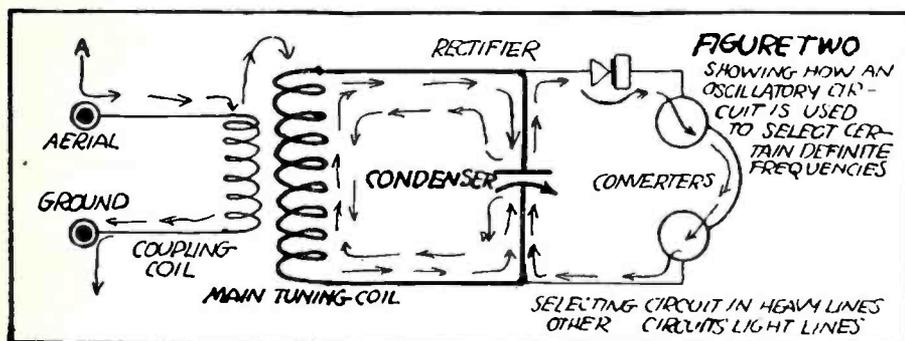
The secondary or oscillatory circuit is the part of the set which accomplishes the action of selecting the desired stations. The impulse or wave is transferred to the main tuning coil by induction and surges back and forth as indicated in the circuit shown in black. The current of a pulsating direct nature is converted by the phones to mechanical energy.
