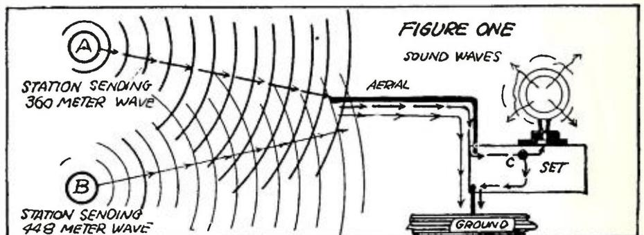
When the set as shown is tuned to Station A, the signals from that station enter the detector C and are changed to sound waves. Waves from Station B pass through the set unchanged, and go off to the ground without being converted into sound, because the set is not in resonance with that frequency.
