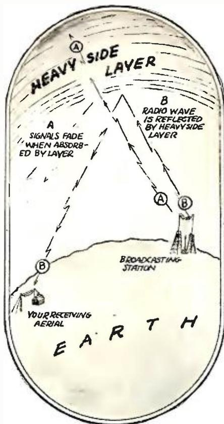
It is supposed that a "Heavy-side layer" as illustrated in the diagram above is responsible for the fading of signals, as well as their propagation along the surface of the earth. When this layer absorbs signals, we have fading.
