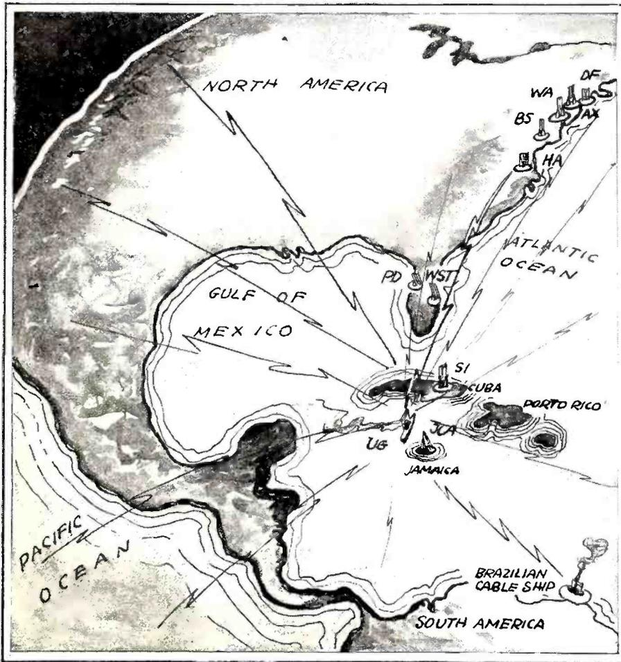
The Steamship "Schley," steaming off the coast of Jamaica, carried on communication with stations indicated by the towers in the photo-diagram above. A log of the stations: AX, Atlantic City; HA, Hatteras; UG, Schley; DF, Coney Island; PD, Tampa; WST, Miami; SI, Guantanamo, Cuba; JCA, Jamaica; WA, Waldorf Astoria; BS, Philadelphia.
