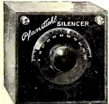
P-500. A new wave-trap efficiency secured with special double Pfanstiehl inductance. \$8.00
