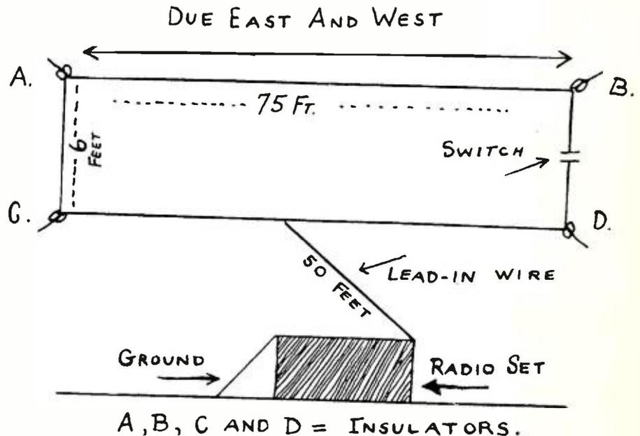
open when radio telegraph messages are being received. The lead-in wire is fifty feet in length and is the same size as the aerial wire.
