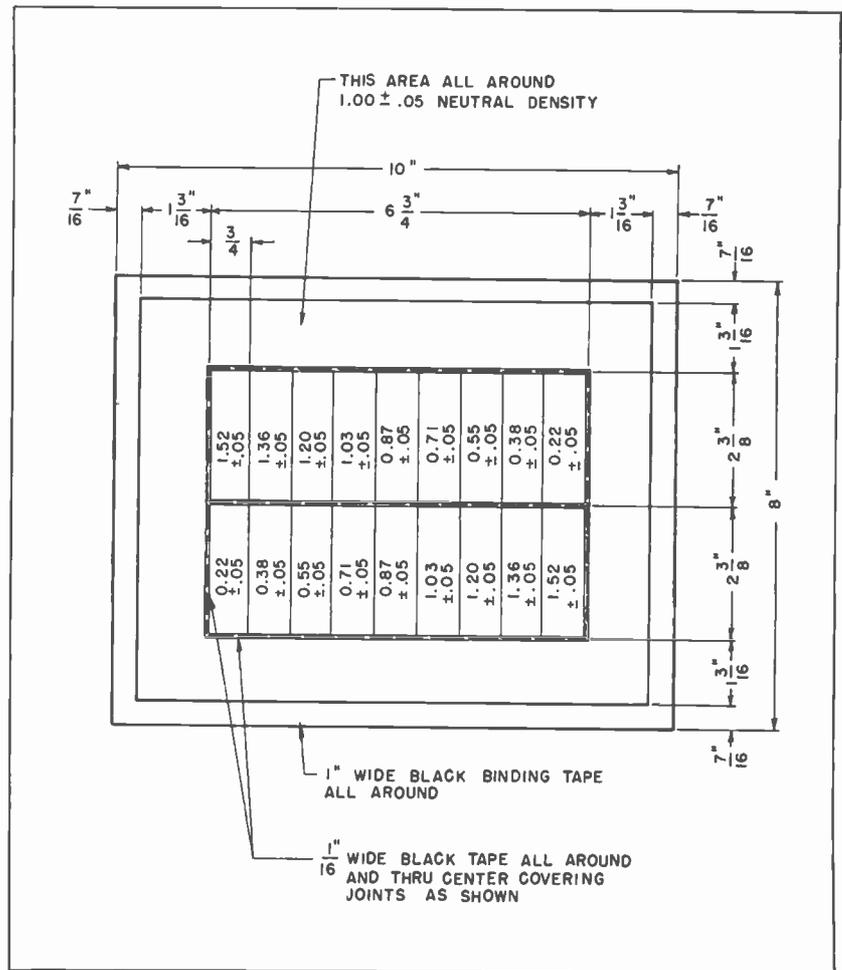
FIG. 4. Proposed RETMA 8 by 10 inch Logarithmic Transmission Transparency.
