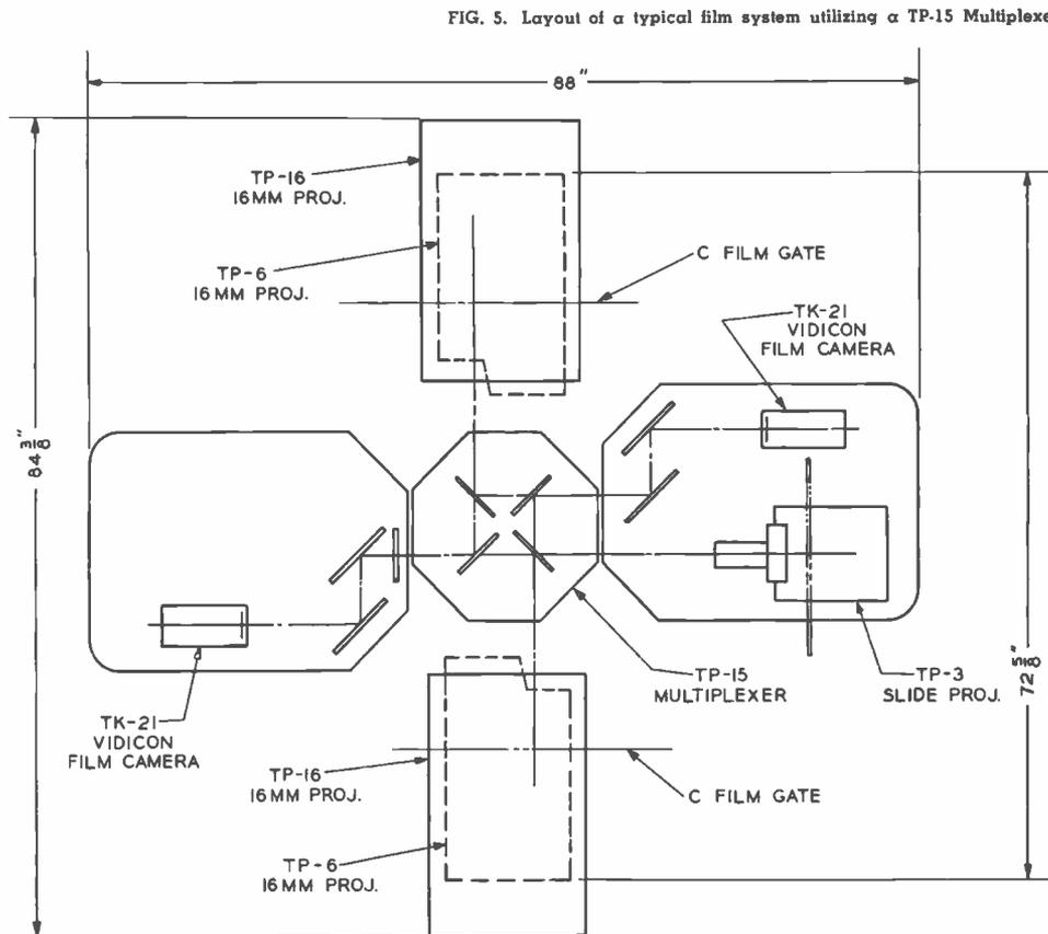
FIG. 5. Layout of a typical film system utilizing a TP-15 Multiplexer.
