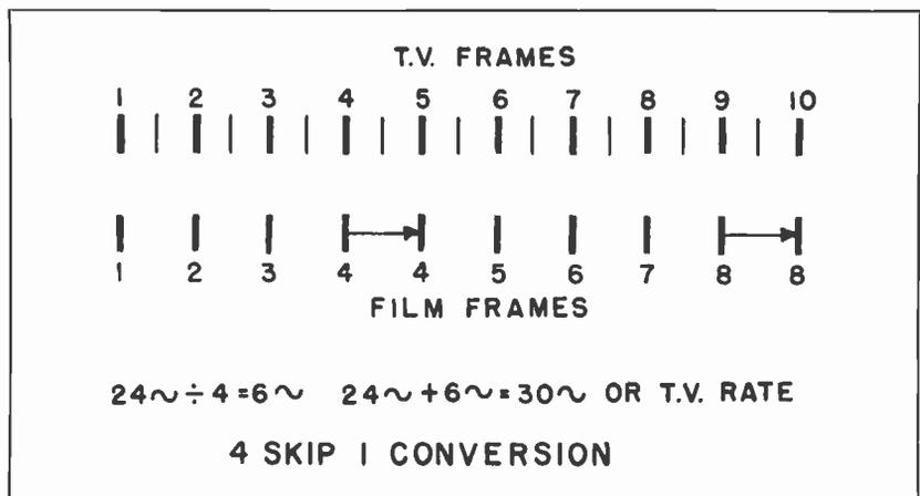
wheel one-half cycle later and advances the film to frame 3. Pin 2 advances the film to frame 4, and is withdrawn. Pin 1, now again extended, advances the film to frame 5 which is the beginning of a new sequence. Four frames of film have served for five frames of television information.
