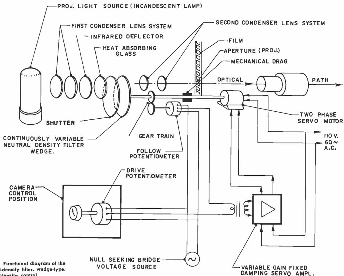
FIG. 1. Functional diagram of the neutral-density filter, wedge-type, light intensity control.
