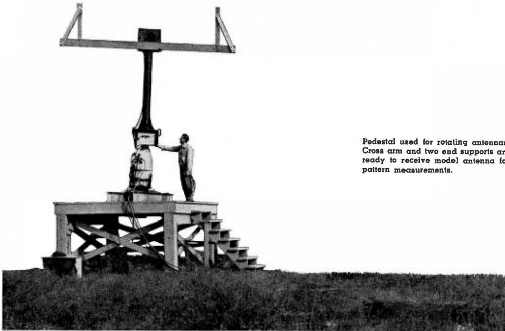
Pedestal used for rotating antennas. Cross arm and two end supports are ready to receive model antenna for pattern measurements.
