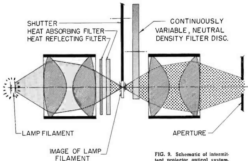
FIG. 9. Schematic of intermittent projector optical system.
