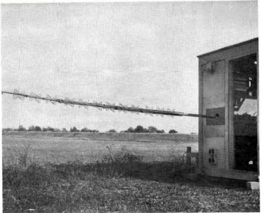
TF-6BM scale model on pattern test set-up.
