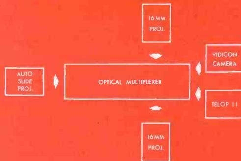
An RCA Multiplexer, Type TP-II allows a single Vidicon Camera to accept up to four film picture sources—two 16mm or 35mm film projectors, a TP-3B, 35mm automatic slide projector, and a Telop II slide and opaque projector. The multiplexer is pictured above in a multi-input film system using two RCA TP-6A professional film projectors.
