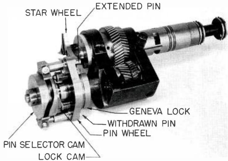
FIG. 6. Overall view of complete intermittent.
