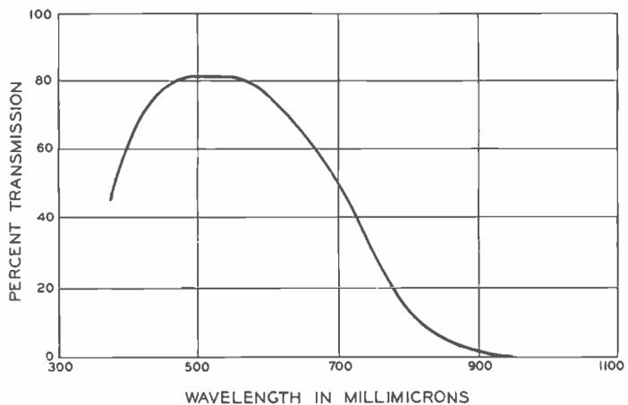
FIG. 6. Transmission characteristics of infrared filter combination.
