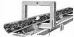
RCA Metal Detector finds metal particles (magnetic and non-magnetic) in rock products, foods, plastics, textiles and other belt-conveyed materials. Protects machinery from damage and product from foreign bodies.
