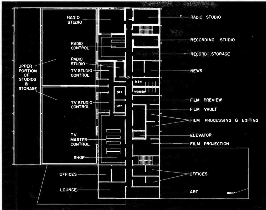
FIG. 4. Upper level plan of fully-expanded scheme.
