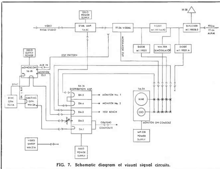
FIG. 7. Schematic diagram of visual signal circuits.
