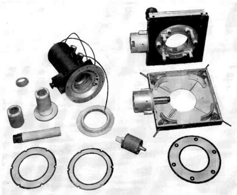
FIG. 11. PA cavity completely disassembled.
