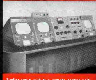
Similar setup with two camera control units (one live and one film, or two film), such as used in the RCA "Basic Buy" for TV.
