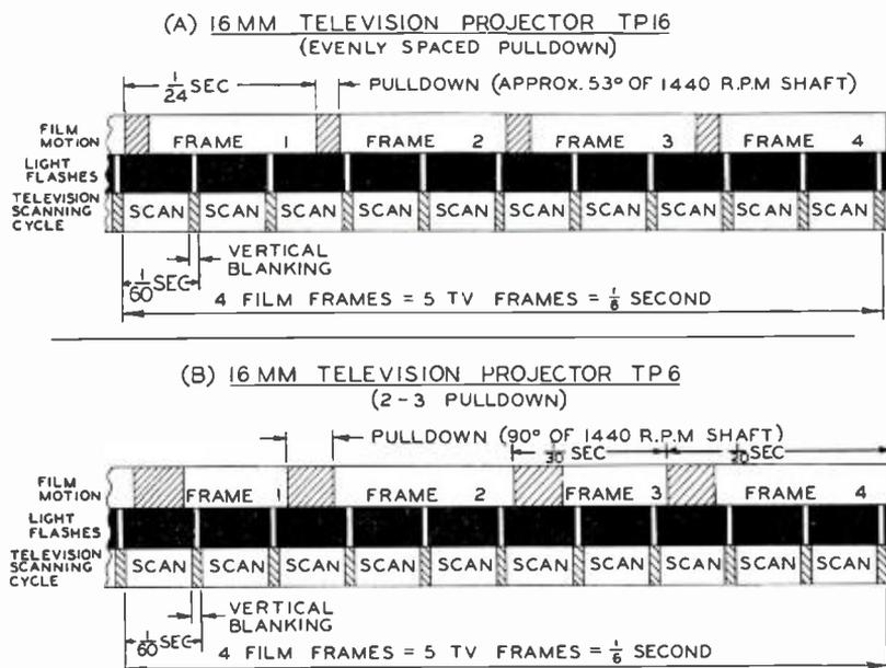
FIG. 6. Sketch showing time cycle comparison of TP-6A Professional Projector with that of the TP-16 Projector.
