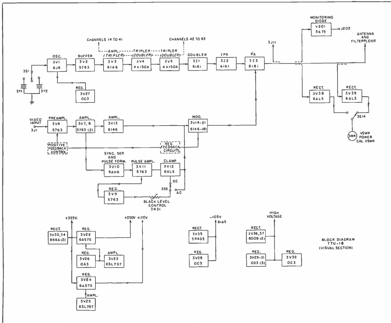
FIG. 5. Block diagram of TTU-1B visual transmitter.
