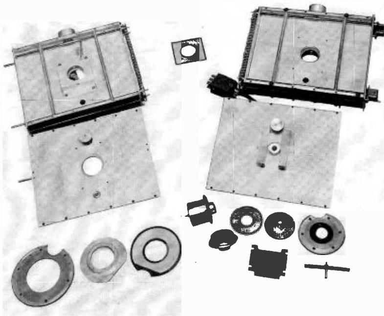
FIG. 9. Rectangular cavity for 6161 disassembled.
