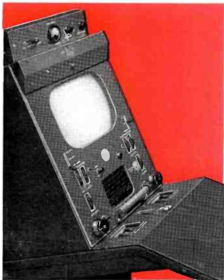
Iconscope beam current control, with indicator. A new arrangement that takes the guesswork out of day-to-day adjustments—provides a standard of comparison to help the operator adjust for optimum picture quality. The panel mounts on the housing of the film camera console, or in the remote control console.
