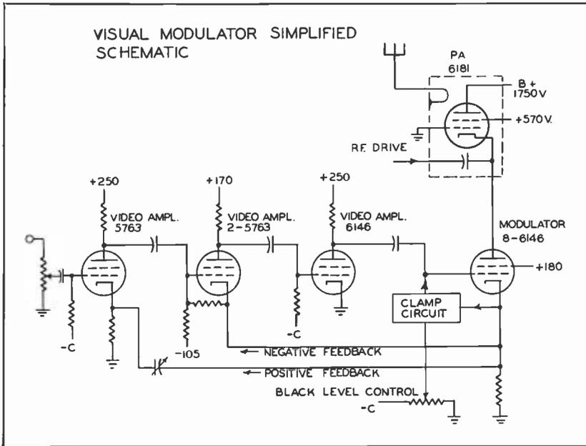
FIG. 7. Visual modulator simplified schematic.
