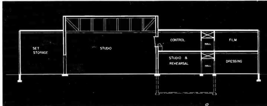
FIG. 5. Cross-sectional drawing which shows vertical relationships among various sections of building.
