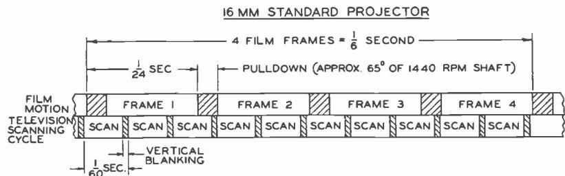
FIG. 5. Time cycling of a standard 16mm projector.
