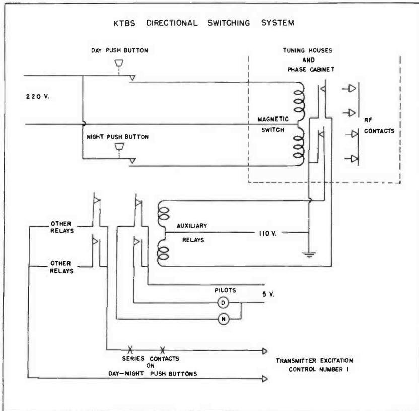
FIG. 12 (left). Simplified schematic of the KTBS directional switching system. Push buttons on the phasing cabinet operate contactors in the phasing cabinet and in the six antenna tuning houses. Back contacts operate signal lights in the transmitter room and prevent excitation from being applied until all contactors have closed.
