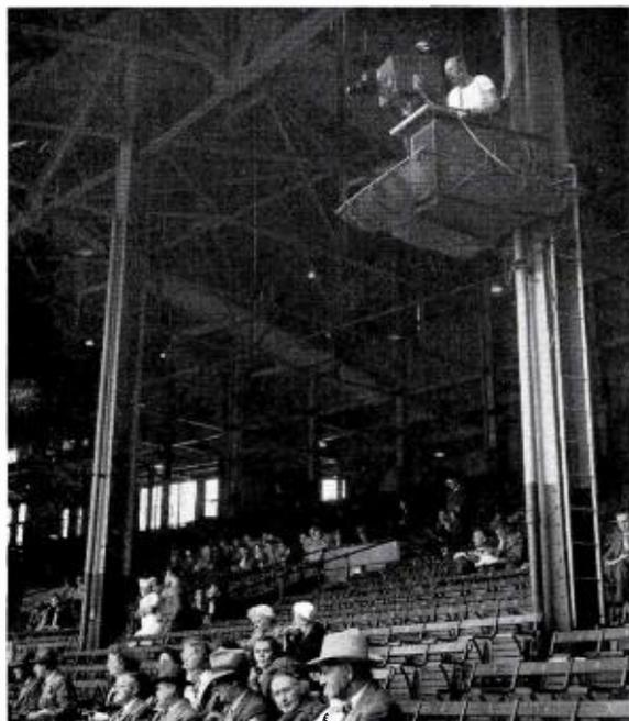
WEWS's camera setup is unusual. No. 1 Camera (shown above) is located in a "crows nest" directly behind homeplate and about 20 feet high, which gives an ideal cover shot. No. 2 is in the second tier toward 1st base. No. 3 is mounted like No. 1 in the lower stands opposite 1st base. Latter is used with 25" lens for dugout interviews—thereby saving the work of moving a camera down to the field for this purpose. WEWS telecasts have been much acclaimed by reviewers.
