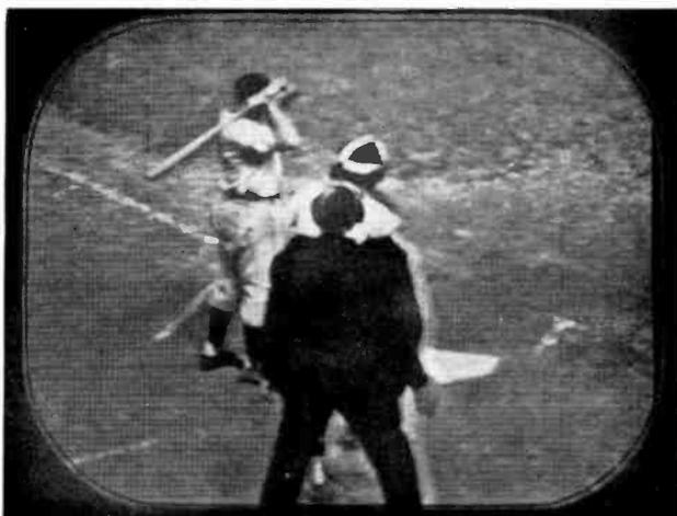
FIG. 9. WTTG NO. 2 SHOT made with an 8" lens on a camera 27 feet high, 75 feet behind (slightly to right of) homeplate.
