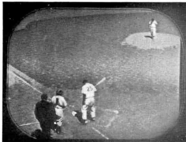
FIG. 5. WTTG COVER SHOT made with a 4" lens on a camera 27 feet high, 75 feet behind (slightly to right of) homeplate.
