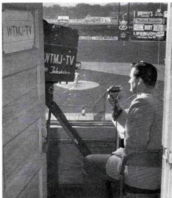
WTMJ-TV's No. 1 Camera, in the plexi-glass enclosed booth on the roof of the grandstand, uses a wide-angle lens to cover ball on infield plays, advanced runner on outfield plays. Announcer is also located in this booth.
