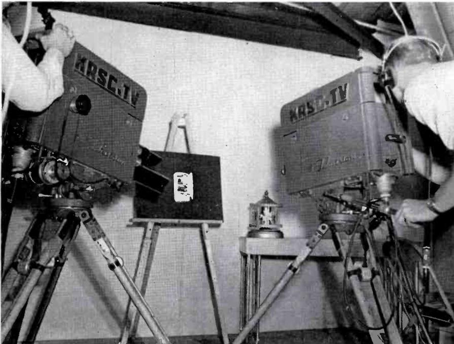
FIG. 23 (left, below). KING-TV (formerly KRSC-TV) produces commercials in the rear of its booth, as shown here—cameras simply swinging around 180° from their normal position. Note Selsyn unit, on left-hand camera, for controlling camera focus (from control position).
