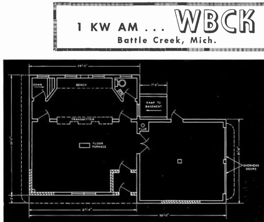
FIG. 2 (above). The floor plan illustrates how the BTA-1L is flush-mounted in one wall, with access doors provided at each side of transmitter.
