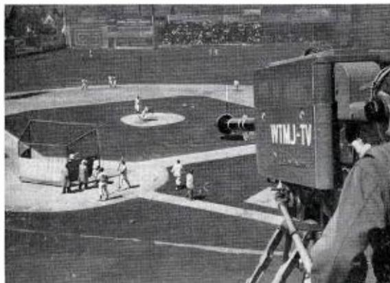
WTMJ-TV's No. 2 Camera, on roof of grandstand toward 1st base, uses a Zoomar daytimes (telephoto, night) to cover advanced runner on infield plays and to follow the ball on outfield plays.
