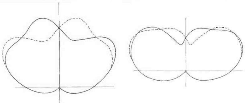
FIGS. 2, 3. Propagation patterns like those shown above are obtainable when Supergain units are connected for turnstiling. The solid and dashed lines show patterns which fit different coverage requirements.
