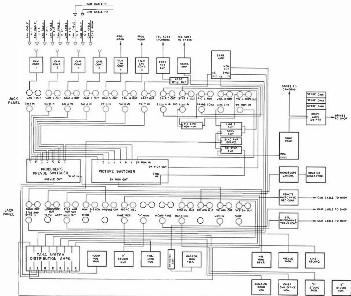
FIG. 11. Block diagram of complete TV audio and video facilities. A system of jack panels in combination with separate systems for preview and program switching affords great flexibility in programming.
