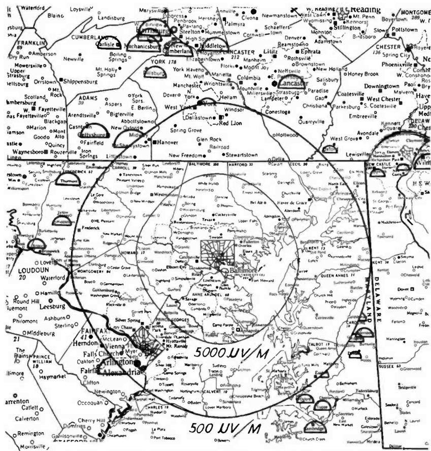
FIG. 17. 5,000 and 500 microvolt/meter contour lines of WBAL-TV. Small semicircles indicate towns outside the 500 microvolt/meter area reporting good reception.
