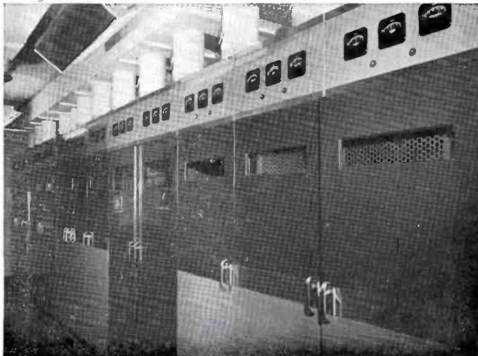
**WENR-TV.** The RCA 5-kw television transmitter Type TT-5A and RCA 10-kw FM transmitter Type BTF-10B at WENR-TV. This ABC station also includes an RCA Superturnstile antenna, field truck and field camera equipment, studio cameras, video and audio control-room equipment, film projectors, film cameras, turntables, and microphones.
