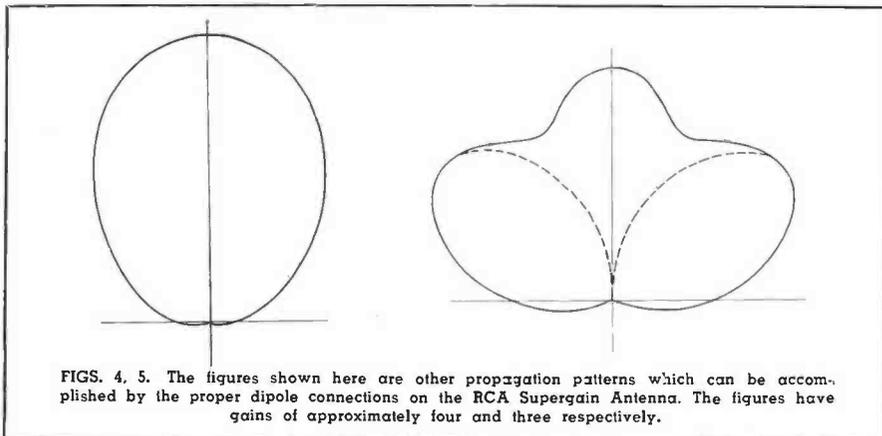
FIGS. 4, 5. The figures shown here are other propagation patterns which can be accomplished by the proper dipole connections on the RCA Supergain Antenna. The figures have gains of approximately four and three respectively.
