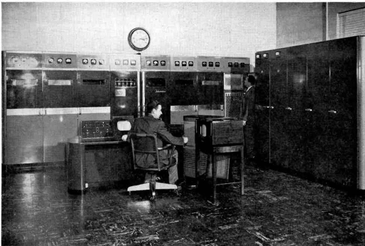
FIG. 14. TT-5A 5KW transmitter and equipment racks of WBAL-TV. Transmitter room also houses the transmitter console, an LC-1A monitoring speaker and modified RCA TV receiver for network viewing. Photo shows TV technicians Arthur Denische (seated at console) and Harrison Brooks.
