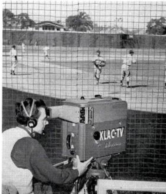
KLAC-TV's No. 1 Camera position is shown above. Here again the location is very low—only 5 feet off the ground. This has the disadvantage that players occasionally walk in front of it—but it gives an unusually dramatic picture of pitcher's delivery. It is even claimed that you can see the ball break on a curve. KLAC-TV's No. 2 Camera is higher—in the first tier at Hollywood, and in the second tier at Los Angeles. This is used for outfield shots.
