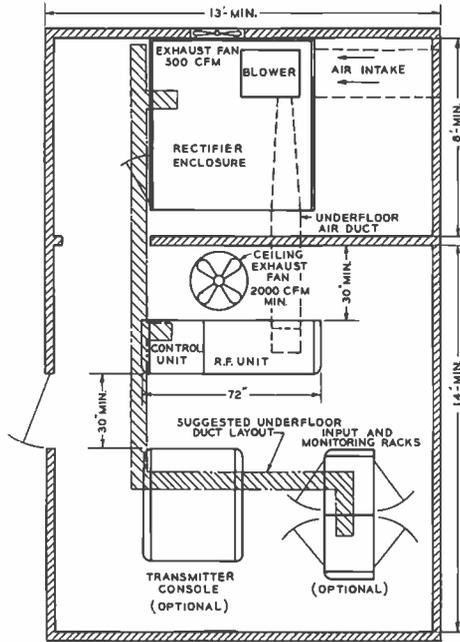
FIG. 4. Various possibilities in which the rectifier enclosure of the TT-2BH transmitter may be installed.
