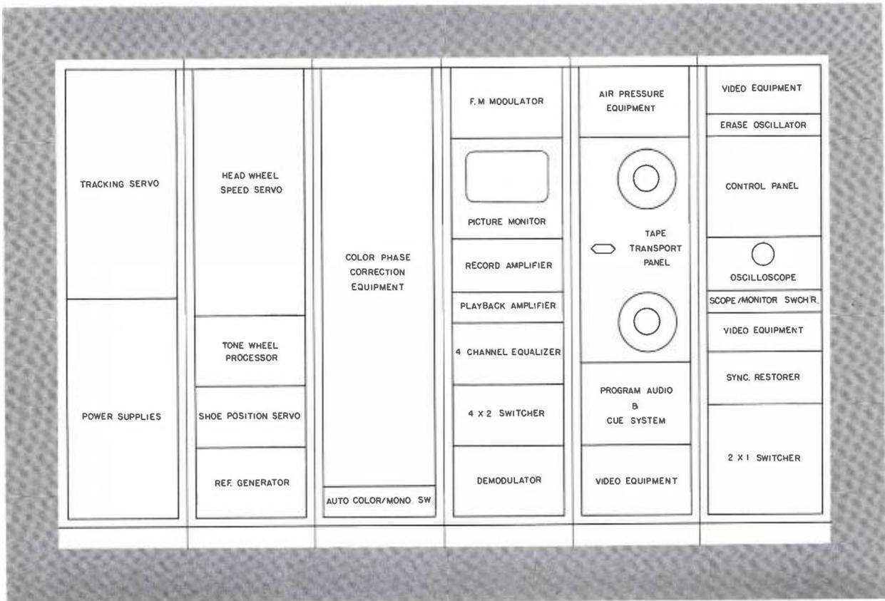
FIG. 6. Rack layout of RCA Color Video Tape Recorder. The three racks at the right form the operating position. The other three racks may be remotely located.
