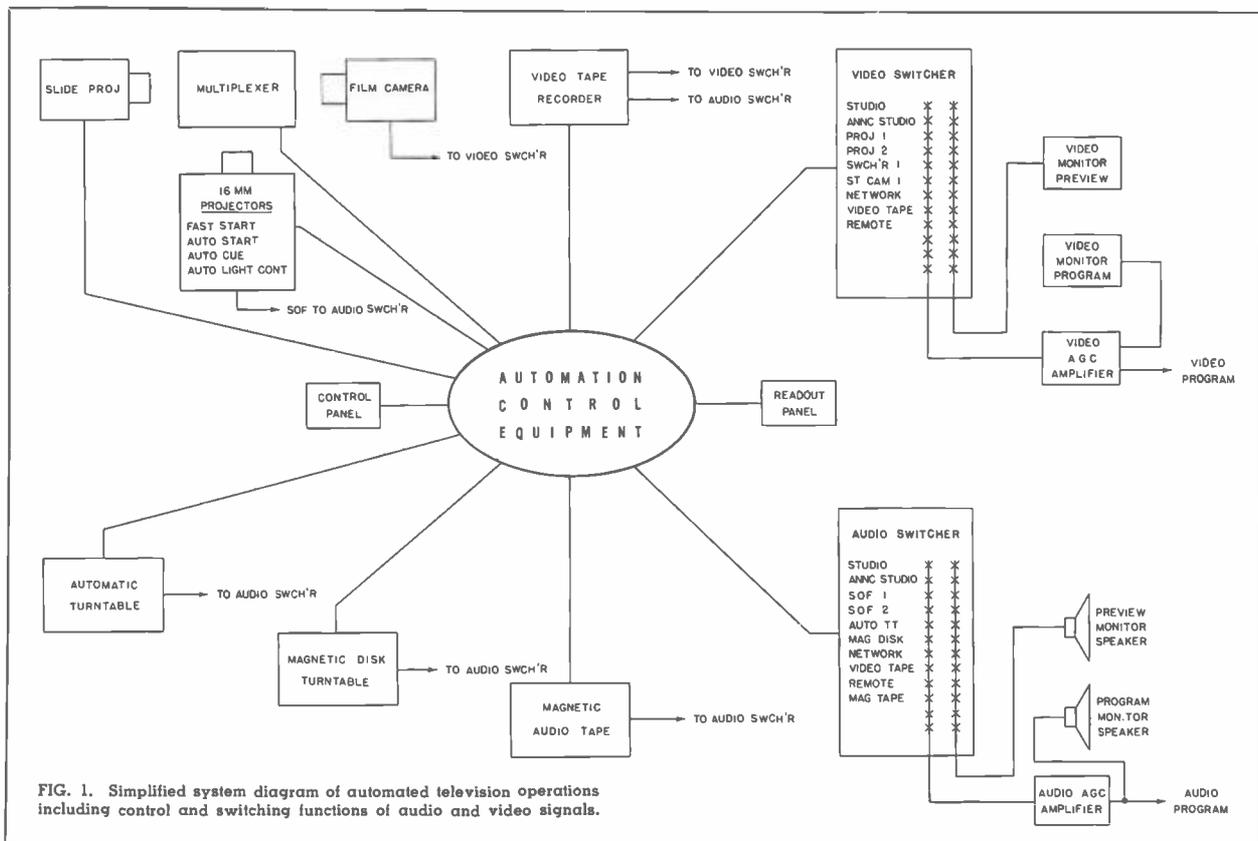
FIG. 1. Simplified system diagram of automated television operations including control and switching functions of audio and video signals.
