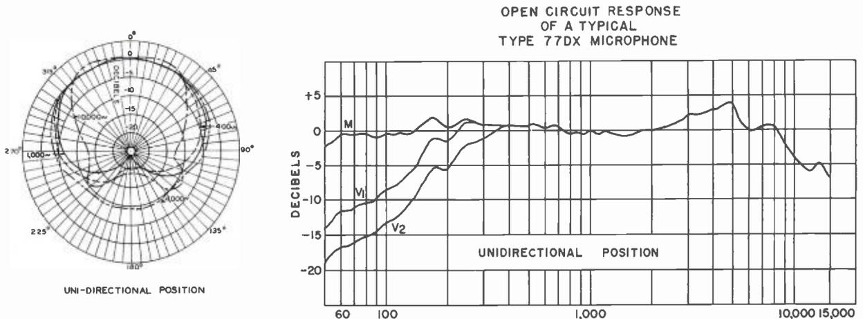
FIG. 7. This is the unidirectional response curve for the RCA Type 77-DX Microphone. A good microphone is necessary for combination control rooms.
