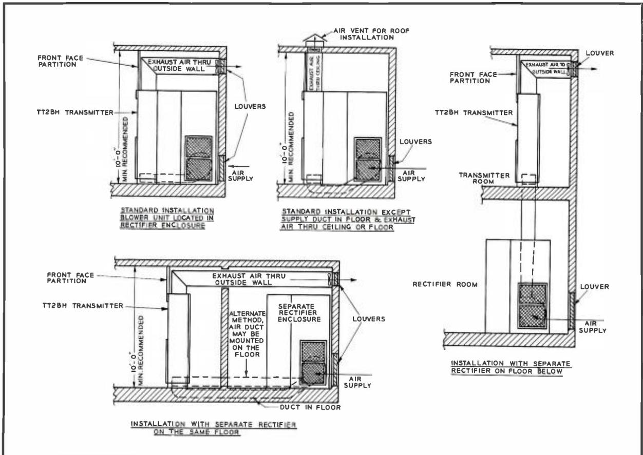
ment is shown in Fig. 3. Variations in the rectifier enclosure installation are shown in Fig. 4. The blower can also be mounted in the basement, by itself, if provisions are made for filtering the intake air.
