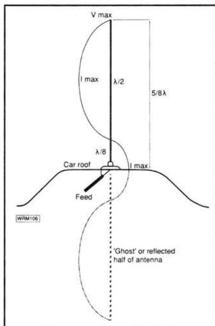
**Fig. 2: Evolution of the 5λ/8 v.h.f. mobile antenna**
