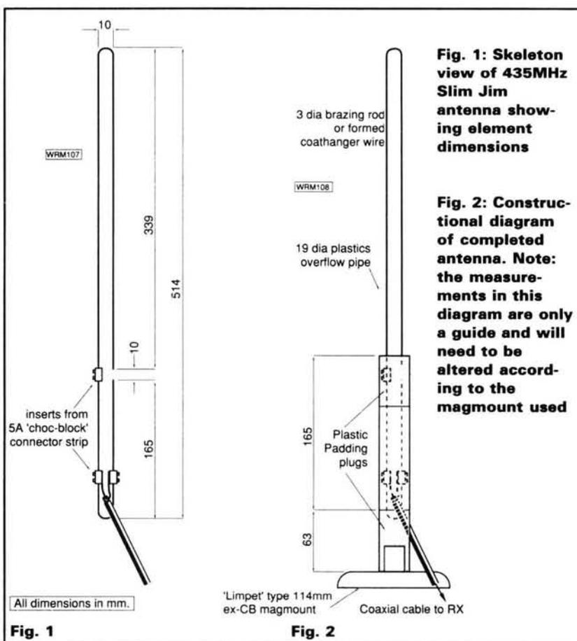
Fig. 1: Skeleton view of 435MHz Slim Jim antenna showing element dimensions
