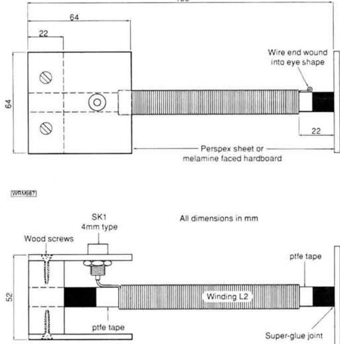
**Fig. 4: Constructional diagram of the "Fe-One" antenna**
