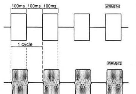
Fig. 10.6: The shaped envelope for Morse dots
