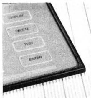
artificial bleepers or lights. The metal dome provides the actual electrical contact of the switch so there is no possibility of a "click" occurring without electrical contact being made. Being metal also means that the switch can handle larger currents than conventional flexible membranes and offer greater reliability.
