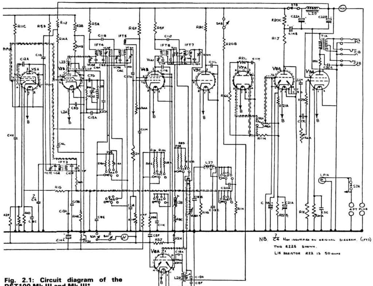
Fig. 2.1: Circuit diagram of the DST100 Mk III and Mk III\*
