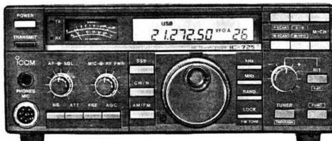
range, automatic gain control, noise blanker, 10dB receiver pre-amplifiers, 20dB receiver attenuator and r.i.t. There are three modes of scanning available:
