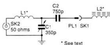
Fig. 3: The "Fe-ONE" experimental compact antenna
