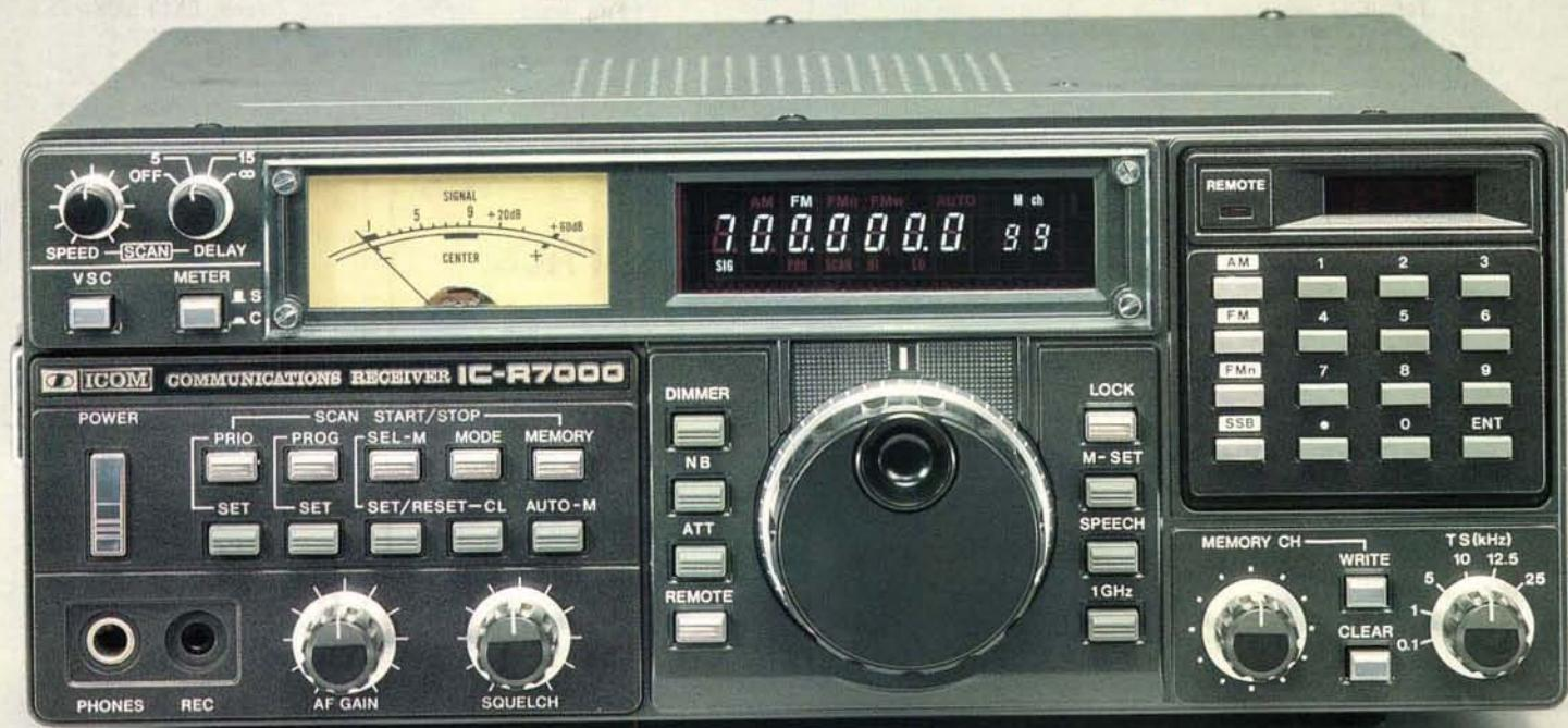
With 99 programmable memories the IC-R7000 covers aircraft, Marine, FM Broadcast, Amateur Radio, television and weather satellite bands. For simplified operation and quick tuning the IC-R7000 features direct keyboard entry. Precise frequencies can be selected by pushing the digit keys in sequence of the frequency or by turning the main tuning knob. FM wide/FM narrow/AM upper and lower SSB modes with six tuning speeds: 0.1, 1.0, 5, 10, 12.5, 25KHz.
