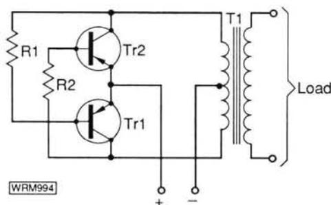
Fig. 1: Basic asynchronous d.c. to a.c. converter circuit
