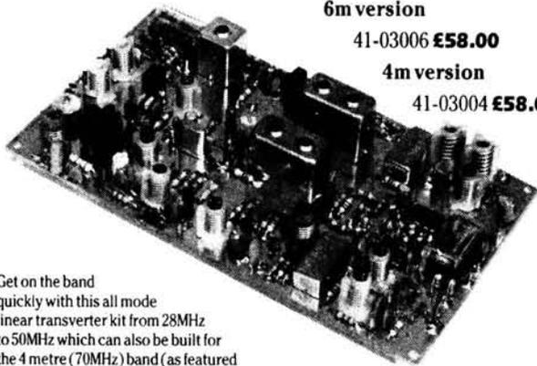
Get on the band quickly with this all mode linear transverter kit from 28MHz to 50MHz which can also be built for the 4 metre (70MHz) band (as featured in the January issue of Ham Radio Today).
