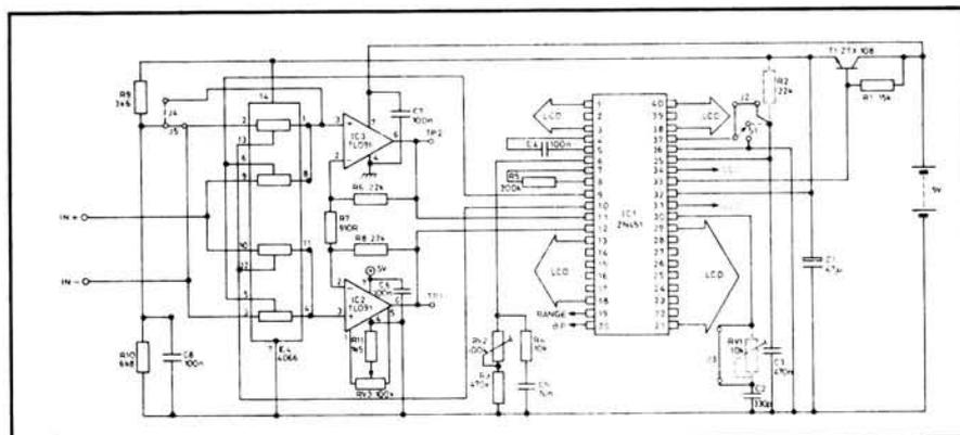
vide the required +5V at pin 32, in conjunction with the internal voltage regulator in the i.c.
