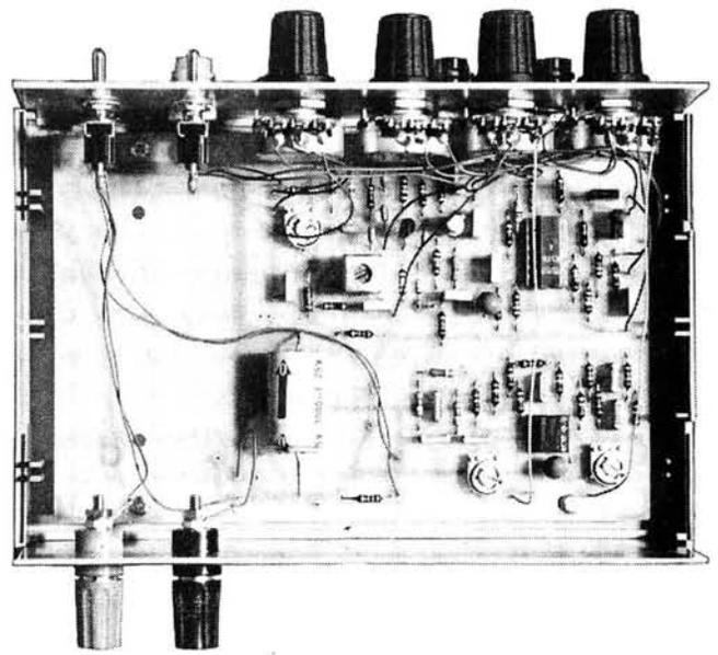
Photograph of the author's prototype showing the general layout of components
