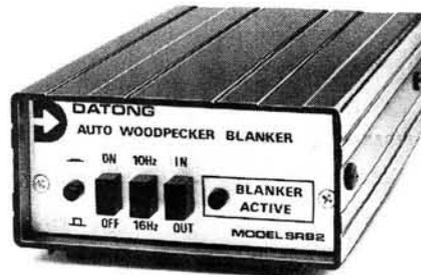
signals even with the severest of Woodpecker interference. When no Woodpecker interference is present, no blanking occurs, and the receiver or transceiver operates exactly as normal.
