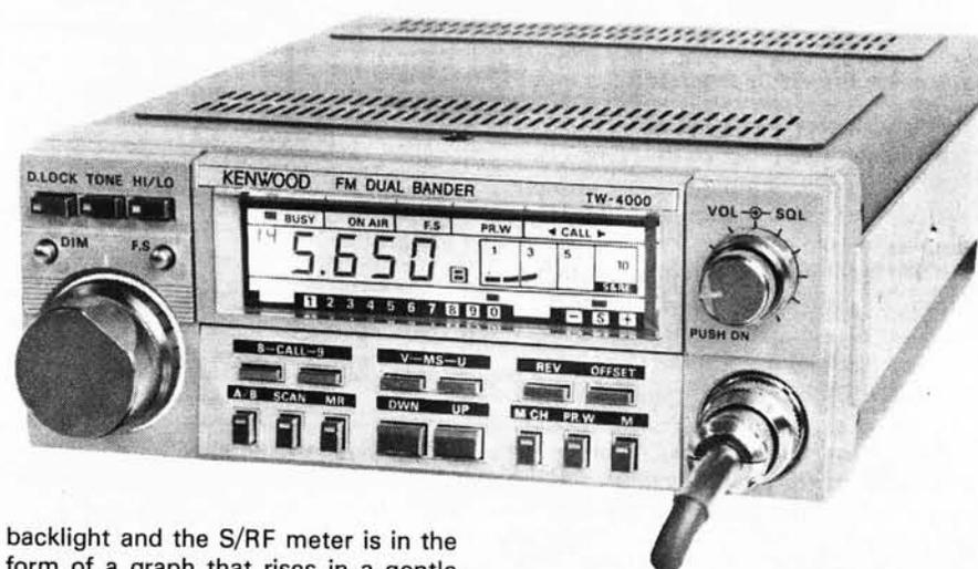
backlight and the S/Rf meter is in the form of a graph that rises in a gentle curve as the signal strength increases.
