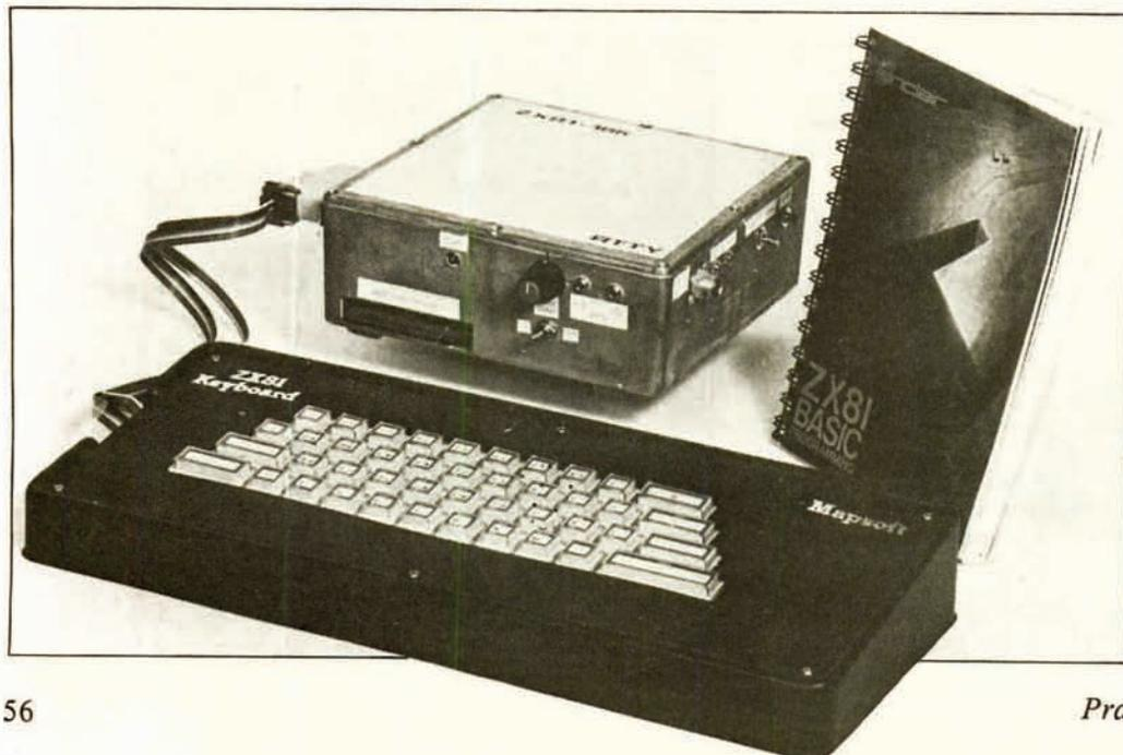
The re-housed ZX81 with the Maplin keyboard. The diecast box houses the mains power supply, mains filter, ZX81, Ground Control 16K RAM board, Scarab interface board together with the various input and output sockets. The Maplin keyboard is a great improvement over the original ZX81 pressure-sensitive one
