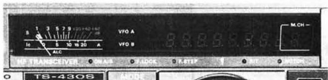
**Trio's attractive new styling incorporates "S" meter, frequency and memory channel indicators within a single window**
