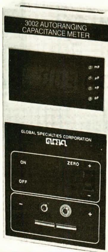
and the instrument automatically selects the most appropriate of the eight ranges. The basic accuracy is claimed to be 0.2 per cent of reading  $\pm 1$  count up to 199.9 $\mu$ F and 1 per cent of reading  $\pm 1$  count up to 19.99mF with a resolution of 0.05 per cent of full scale on all ranges and 1pF on the lowest range.
