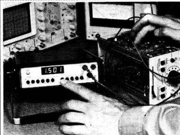
In use here is the Advance DMM7 digital multimeter, a new 3½-digit 5-function instrument.
