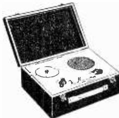
A well-tryed portable, using high efficiency ferrite rod aerial. 2 waveband. 4 valves. Build it during the dark evenings ready for the spring. Full constructional data and price list 1/6. Total building cost £7-10-0.
