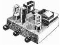
Valve line-up 6SL7, 6V6 and 6X5. FOR A.C. MAINS 200/250 VOLTS. The output Valve is of the beam type and feeds 4 watts into a specially designed output Transformer
