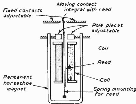
Fig. 3.—A simplified cross-sectional diagram of a high-speed polarised relay. The moving contact need not necessarily be insulated from the reed.
