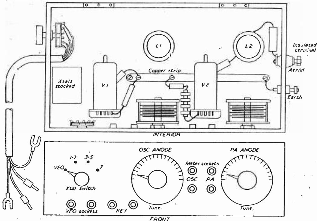
Fig. 2.—Layout and panel details.
