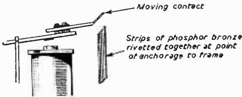
Fig. 2(b)—Another heavy current relay. In this case the contacts are, to a certain extent, self-cleaning.
