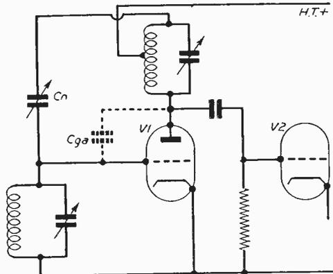
Fig. 49.—Method of neutralising grid-anode capacitance.
