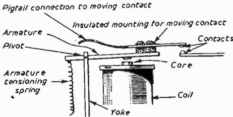
Fig. 2(a)—An alternative type of relay construction permitting the switching of heavy currents.
