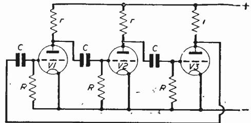
Fig. 1.—Relaxation oscillator for nearly pure sine waveform.
