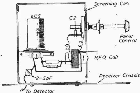
Fig. 6.—A typical B.F.O. stage layout.
