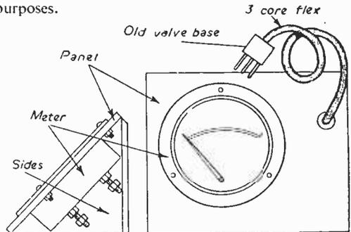
Fig. 2.—Constructional arrangement.
