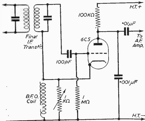
Fig. 5.—A cathode-coupled det. B.F.O. stage.
