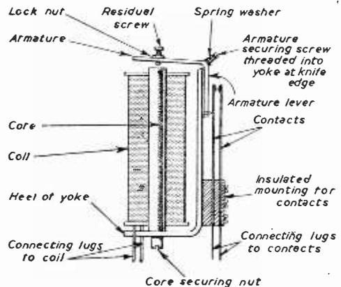
Fig. 1.—Cross-section of a typical relay. The coil lugs pass through holes in the heel of the yoke. An extension on the moving contact nearest the yoke bears against an insulated inset on the armature lever.
