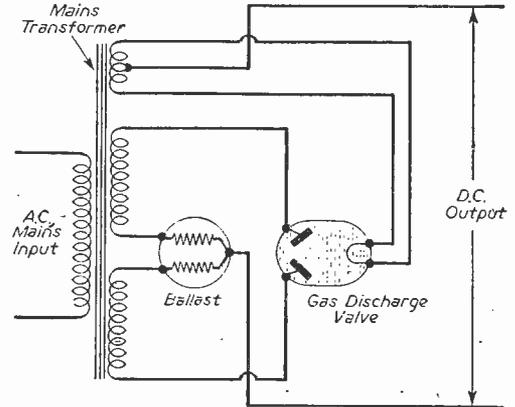
Fig. 1.—The full-wave circuit with centre-tapped filament.
