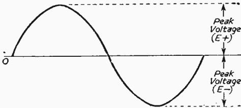
Fig. 10.—One cycle of sine-wave.
