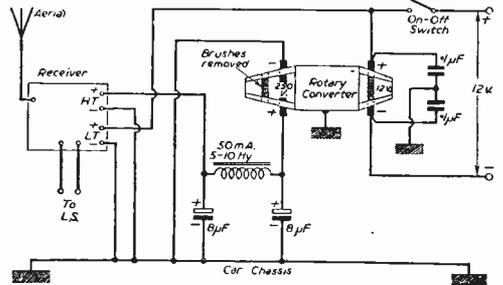
Details of a converter power supply.
