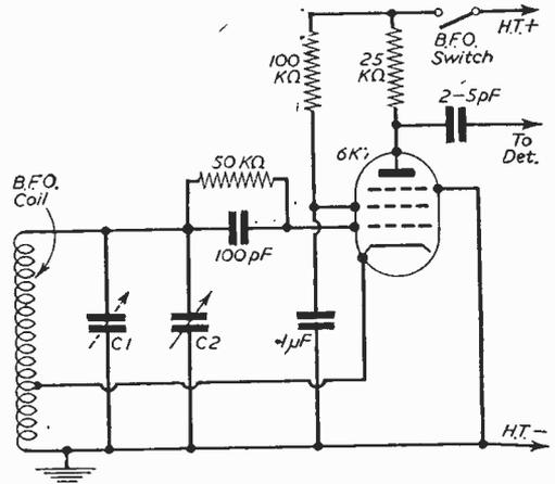
Fig. 1.—A typical B.F.O. stage.
