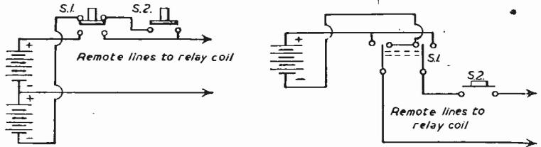
Fig. 5(a)—A remote circuit for controlling the relay of Fig. 4. S1 and S2 are push-buttons which when pressed cause the relay armature to move in the desired direction. The double-pole arrangement at S1 is included to prevent damage should both push-buttons be accidentally pressed at the same time. Fig. 5(b)—An alternative control circuit using only one battery. In this case the D.P.D.T. switch S1 selects the desired movement of the relay, push-button S2 being pressed to actuate it.
