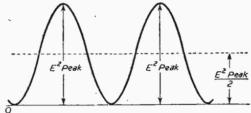
Fig. 11.—This curve is evolved by plotting against time all the squares of the instantaneous voltage values in the sine-wave at Fig. 10.
