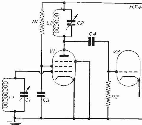
Fig. 48.—Basic R.F. amplifying circuit.
