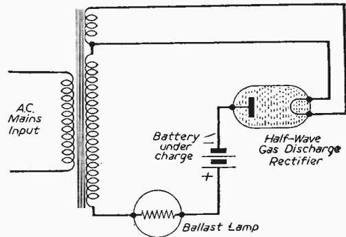
Fig. 2.—This shows a half-wave circuit.
