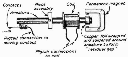
Fig. 4—A suggested design for a relay which can be easily constructed in the amateur workshop. The possible contact assemblies are not, of course, limited to the simple arrangement shown here.
