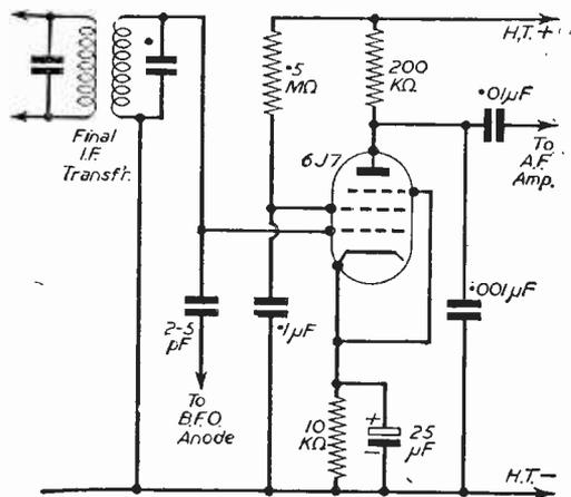
Fig. 4.—Grid detector with BFO input.
