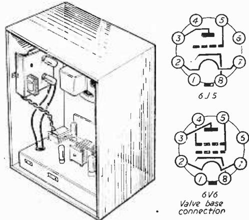
Fig. 2.—Position of amplifier in existing cabinet and valve base data.
