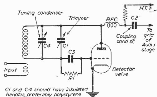
Fig. 2.—Basic self-quenched capacitive circuit
