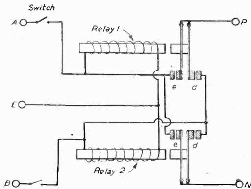
Fig. 1.—Standard circuit recommended by the author—e and d depict energised and de-energised positions respectively.
