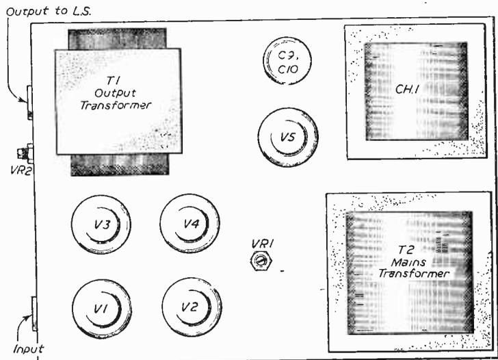
Fig. 2.—Suggested layout of the main components.
