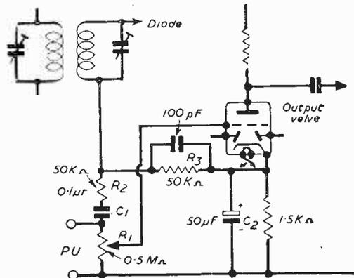
Fig. 3.—A typical pick-up input circuit of an average receiver.
