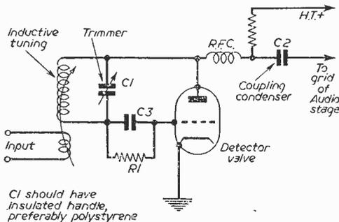
Fig. 1.—Basic self-quenched inductive circuit.
