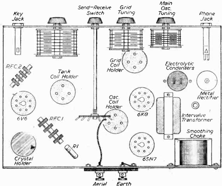
Fig. 4.—Below chassis layout.
