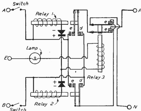
Fig. 3.—Inclusion of a third relay.
