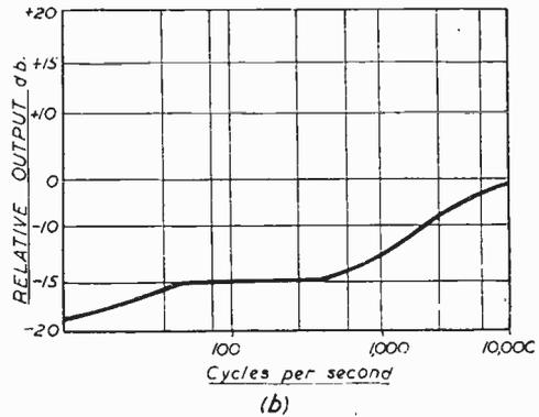
Fig. 2(a).—Approximate crystal pick-up response and (b).—Approximate magnetic pick-up response.
