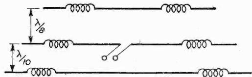
Fig. 5.—A compact close-spaced beam offers scope for experiment.
