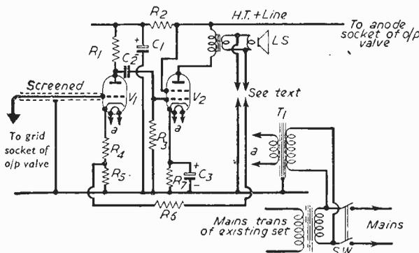
Fig. 1.—Theoretical circuit of the amplifier.
