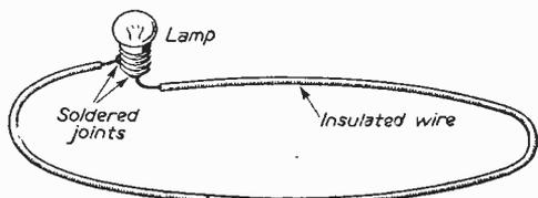
Fig. 2.—Simple oscillation tester.
