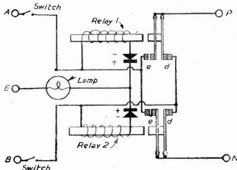
Fig. 2.—Modification for use with low-current relays.
