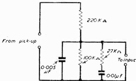
Fig. 4.—A bass-boost circuit for a magnetic long-playing pick-up.
