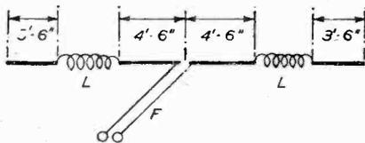
Fig. 4.—End-loading enables an efficient radiating system to be accommodated in a small space. The above aerial is some 16ft. in length, yet radiates effectively on 14 Mc/s.
