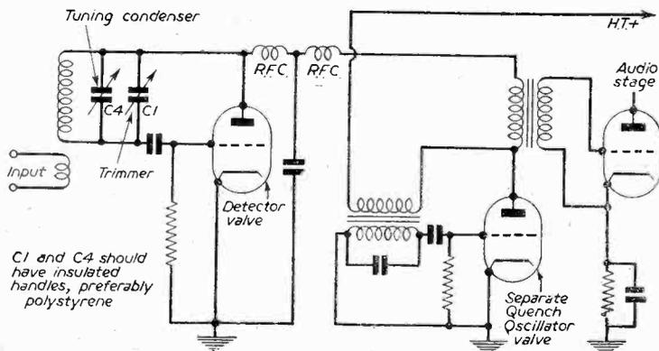
Fig. 3.—Basic externally quenched (capacitive) circuit.
