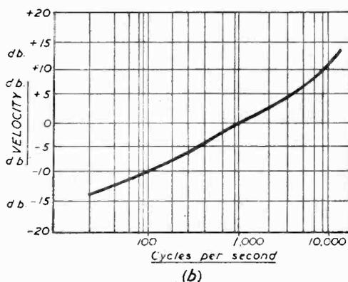
Fig. 1(a).—78 R.P.M. recording characteristic and (b).—Microgroove recording characteristic.
