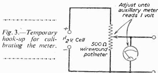
Fig. 3.—Temporary hook-up for calibrating the meter.
