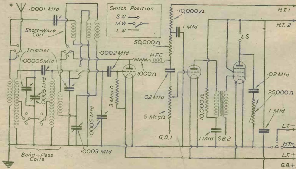
Fig. 1.—Theoretical circuit of the All-wave Three.
