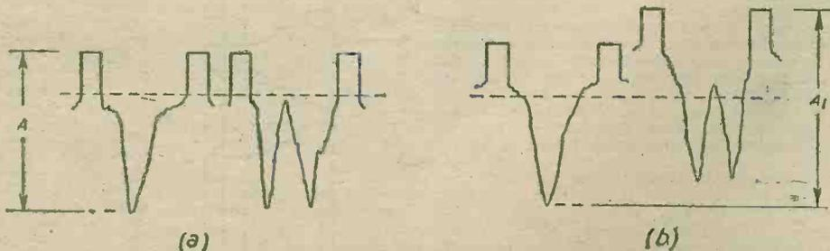
Fig. 17.—Vision signals with the D.C. component retained at (a) do not constitute such an uneconomical grid swing as those with the D.C. component removed as at (b).
