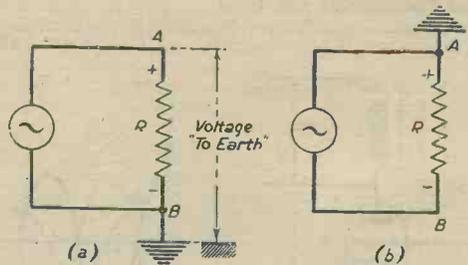
Fig. 4.—A simple "earthed" A.C. circuit to illustrate "phase-reversal"—of the insulated end relative to earth. Compare with Fig. 1 and Fig. 3.
