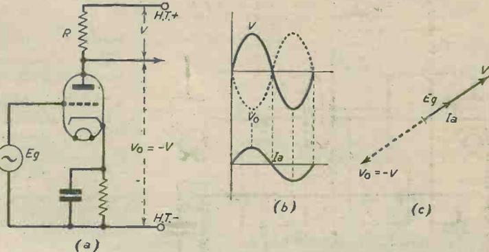
Fig. 1.—Phase relations in a simple stage with resistance load  $R$ :  $E_g$  and  $I_a$  are in phase.  $I_a$  develops a "supply-voltage"  $V$  across  $R$ , but the output voltage  $V_o$  is at 180 deg. to  $V$ , i.e., phase-reversed to the load voltage, and to  $E_g$ .
