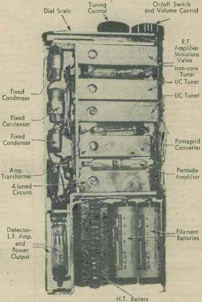
Interior of the new Belmont Pocket Radio Receiver. This measures 3in. wide, 6½in. high, and is only ¼in. thick. It weighs 10 ounces with batteries. The complete set may be seen on page 443.
