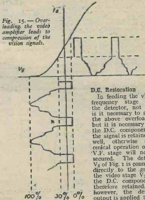
Fig. 15.—Overloading the video amplifier leads to compression of the vision signals.
