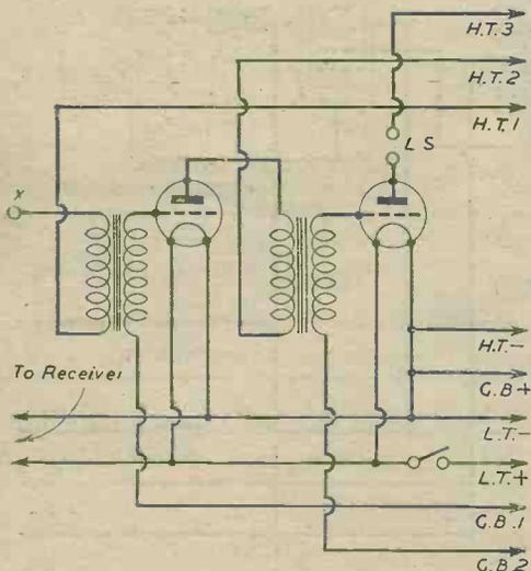
Fig. 4.—A two-transformer coupled amplifier, without decoupling.
