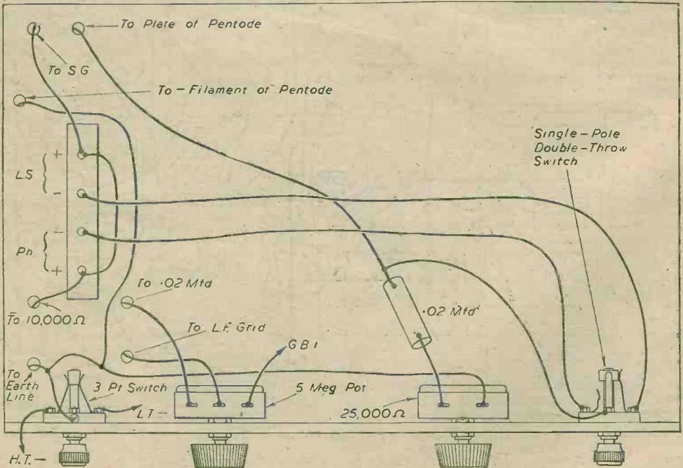
Fig. 3.—Under-chassis wiring of the receiver described above.
