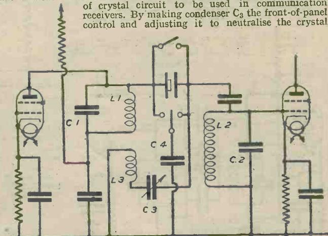
Fig. 2.—A simple single neutralised I.F. Crystal Stage circuit.
