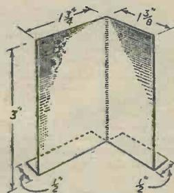
Fig. 5.—Details of the battery compartment.
