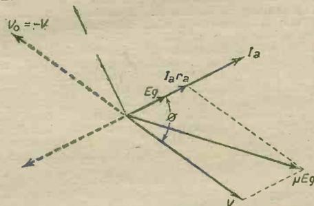
Fig. 7.—Vector diagram for load having resistance and capacitive reactance.
