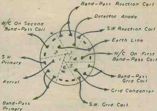
Fig. 4.—Details of the switch wiring.
