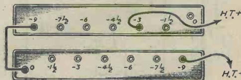
Fig. 6.—Connections for the two grid-bias batteries.
