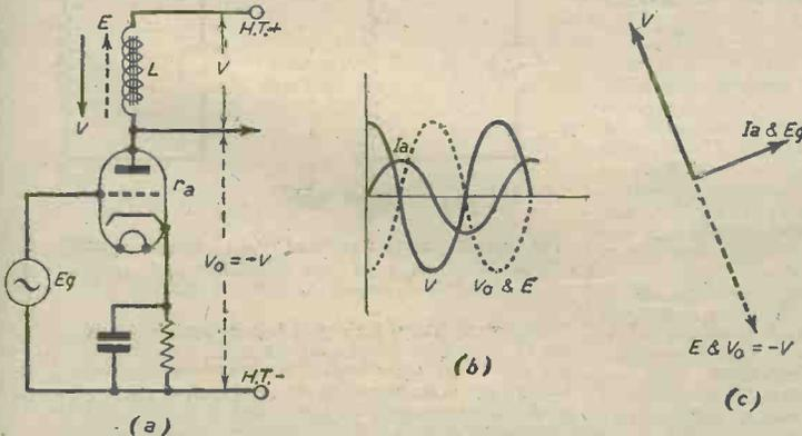
Fig. 2.—With a pure inductance  $L$  in the anode circuit, there is a back E.M.F.,  $E_s$ , which requires a "supply" component  $V$  equal and opposite to it. The anode-to-cathode valve voltage,  $V_o$ , has the same phase as  $E_s$ , i.e., both have a negative sign, relative to  $V$ .
