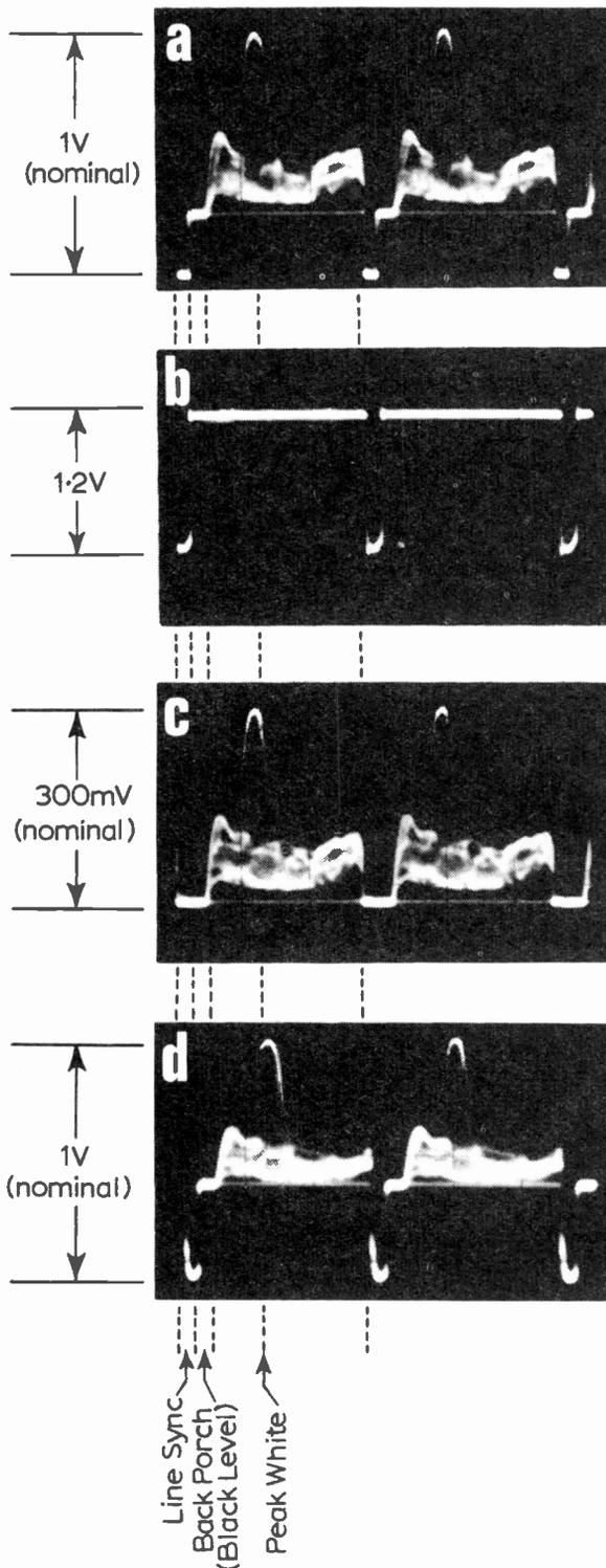
Fig. 3 (left): Waveforms. (a) Input from camera (250mV/cm vertical deflection). (b) Sync pulses at Tr2 collector, extracted from the composite input signal (500mV/cm vertical deflection). (c) Video signal at Tr4 emitter, with sync pulses removed (500mV/cm vertical deflection). (d) Mixed and processed video signal recombined at the mixer output (junction C8/R26) with the sync pulses (250mV/cm vertical deflection). The video and sync ratios are controlled by the values of R6, R12 and R20.
