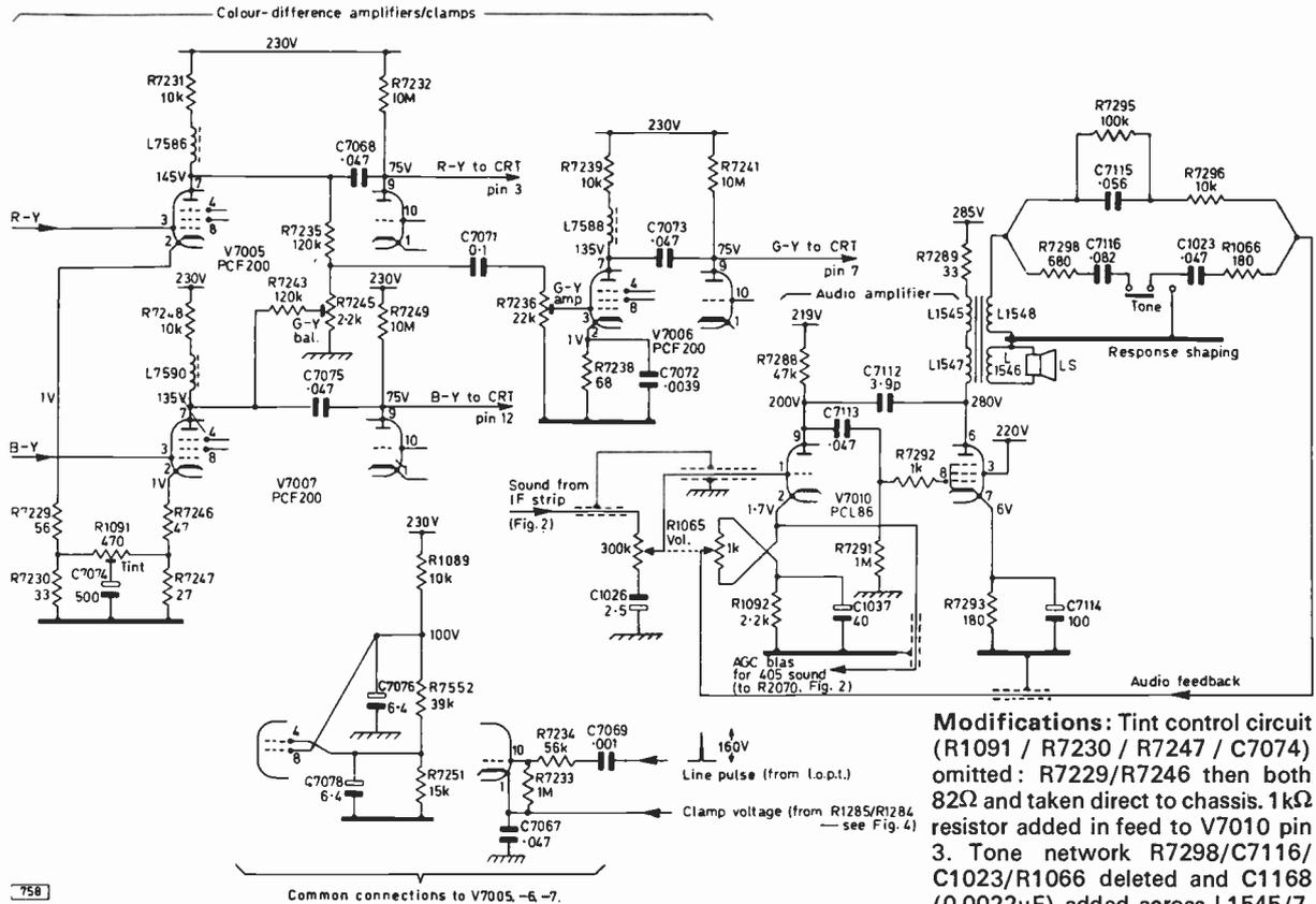
**Modifications:** Tint control circuit (R1091 / R7230 / R7247 / C7074) omitted: R7229/R7246 then both 82Ω and taken direct to chassis. 1kΩ resistor added in feed to V7010 pin 3. Tone network R7298/C7116/C1023/R1066 deleted and C1168 (0.0022μF) added across L1545/7.
