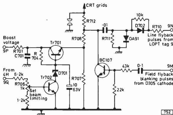
Fig. 2: Beam limiting and flyback blanking circuit used by L. Cook.
