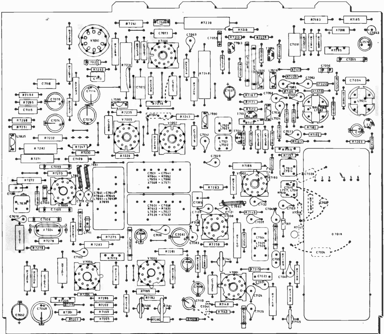
Fig. 10: Layout of the decoder panel. The author advises cutting out R7209 (if present) at lower left. On some panels the sound output transformer is mounted above left. Corrections: C7504 should read R7504 and L7505, L7506 (can with L7509); C7076 should read C7096 (left-hand side beneath L7638).
