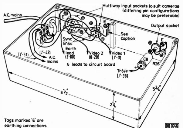
Fig. 2: Wiring to the case. The board and the controls are mounted on the lid of the diecast box. The resistor (say 100Ω) shown terminating the sync link at the camera 1 socket may be necessary to match sync lines.
