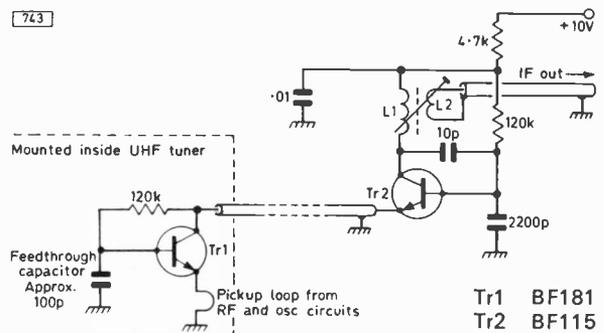
Fig. 3: Cascode mixer-amplifier circuit.
