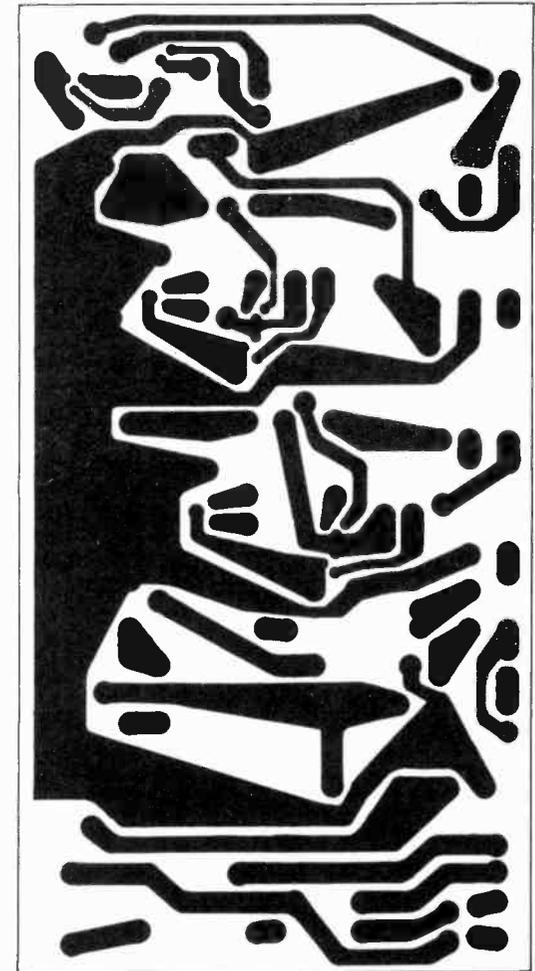
Fig. 7 (right): Printed panel pattern (copper side), shown half scale.
