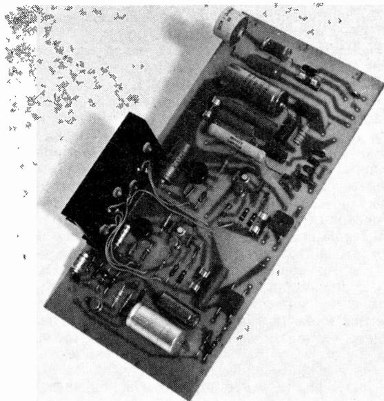
*E. Erven's power supply unit. Four large can electrolytics are separately mounted using suitable clips.*
