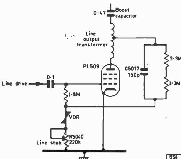
Fig. 1: Line output valve grid circuit of the Philips G6 chassis (single-standard version). The complaint was occasional erratic width reduction.
