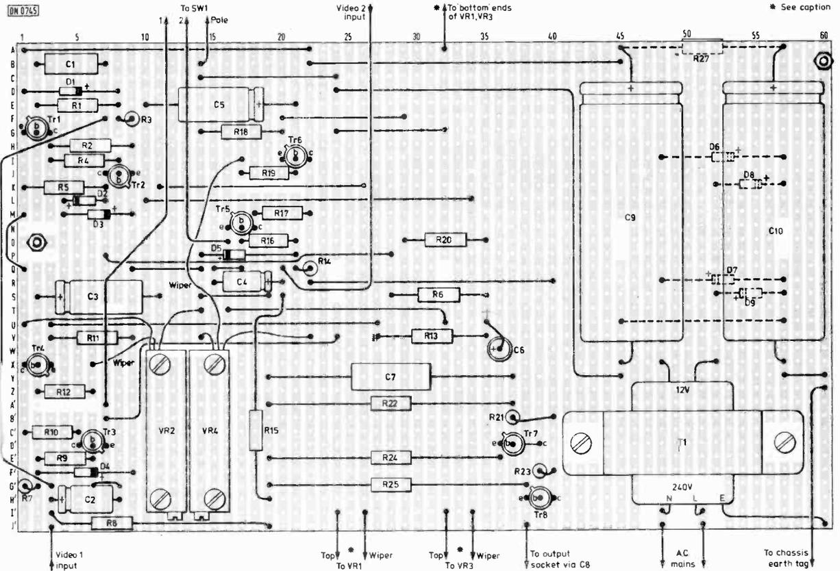
Fig. 4: Veroboard layout, viewed from the component side (0.1 in. Veroboard used). R27 and D6-9 are mounted on the copper side. Connections to VR1 and VR3 can be made via flying leads or if sliding potentiometers are used (as in the prototype) these can be soldered directly to the copper side. Ensure that the mains connections are well insulated from the rest of the circuit board.
