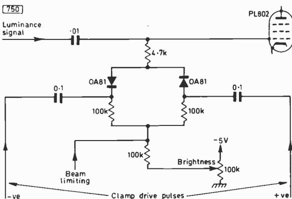
Fig. 2: Double-diode driven clamp used in the RBM dual-standard colour chassis.
