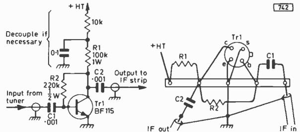
Fig. 1 (left): Simple untuned transistor i.f. stage.
