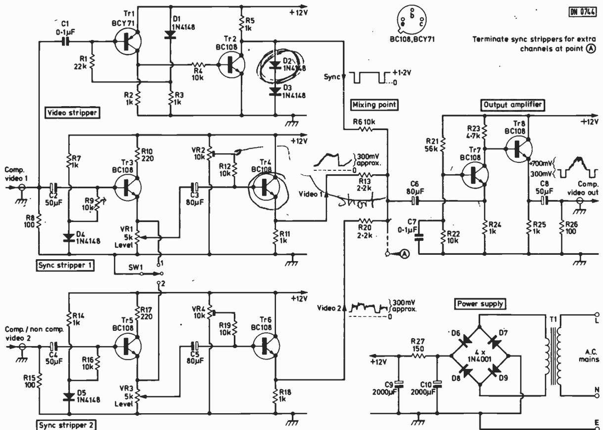
Fig. 1: Circuit diagram of the video mixer—two-channel version.
