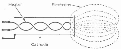
Fig. 1—When heated by the heater the specially coated cathode produces electrons which fall back to the cathode if not attracted by a positively charged anode.
