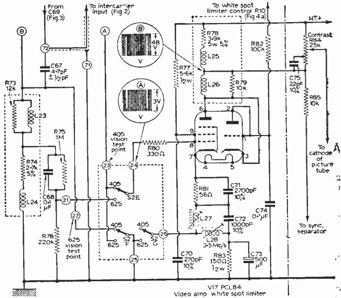
Now in the “625” position the “earth” is removed from point “B” and applied instead to point “A”. The detector load then comprises R74 (Fig. 5) and, after filtering by L23 and L25, the video signal is applied in reversed sense to the control grid of the video amplifier valve via S2E—which is now in position “b”.
