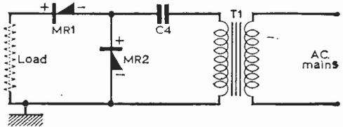
shown unless arrangements are made to feed such a heater from a separate l.t. winding. The capacitors C2, 3, 4 must be adequately rated and a panel lamp and associated warning lens are desirable inclusions.
