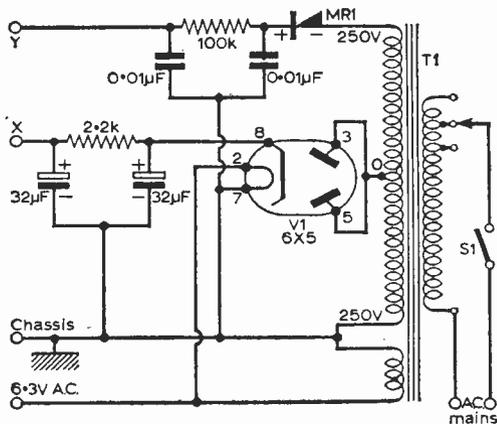
Fig. 1—Simple arrangement of two separate half-wave circuits.
