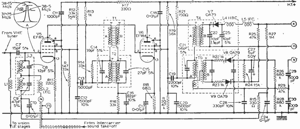
amplifier V5, from whence it is fed to V6 and to the f.m. ratio detector. S2 now selects the f.m.-derived audio and passes it to the sound amplifier and output stage, the latter driving the loudspeaker as before.
