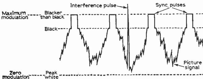
Fig. 36—Showing how an interference pulse appears on a negatively-modulated television signal. Note that the pulse rises in the direction of the sync pulses.
