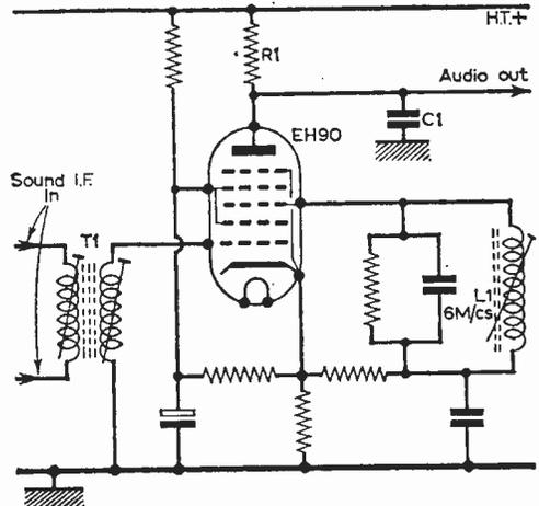
Fig. 39—Circuit of the locked-oscillator FM detector using the Mullard EH90 heptode valve.
