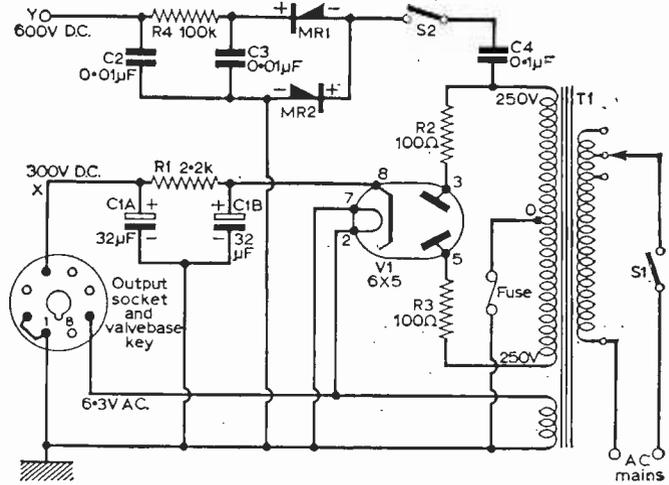
Fig. 2 (above)—An improved version of the basic arrangement, using full-wave rectification.
