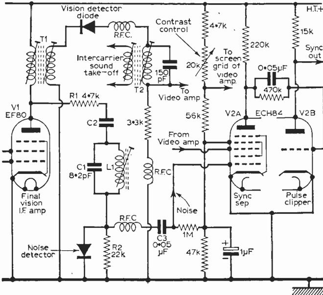
Fig. 38—An interference-cancelling sync separator circuit based on the Mullard ECH84 triode-heptode valve (see text).
