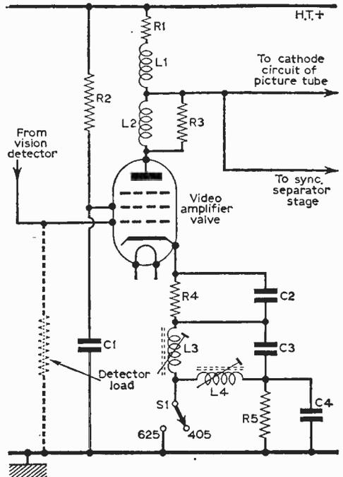
Fig. 27—Video amplifier stage used in some switchable receivers. On 405 lines the stage is biased for the positive signal drive by the voltage dropped across R4 and R5 in series, but on 625 lines the bias is reduced to cater for the negative signal drive by switch S1 short-circuiting R5.
