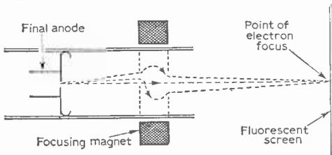
Fig. 3—The electron beam is brought to a point of focus at the fluorescent screen either by a magnetic or electrostatic field. This diagram shows the twisting effect imparted to the electrons by a magnetic focusing field.
