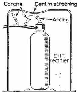
Fig. 57—Arcing from the anode of the e.h.t. rectifier can be caused by a dent in the screening can or shield, as this drawing shows. Corona produces a bluish ray from the discharge point usually to a chassis member, and is accompanied by a hissing sound. Corona may need a darkened room to display itself, while arcing is far more vigorous; it sounds like sharp, staccato cracks and is clearly visible even in daylight.
