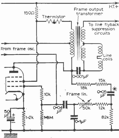
Fig. 55—The basic frame amplifier circuit of the K-B New Queen Special, Model OV30. In the event of limited picture height, the capacitor marked thus\* can be reduced from 0.05 $\mu$ F to 0.025 $\mu$ F (see text).
