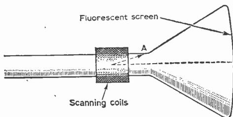
Fig. 5—Corner cutting often occurs due to the electron beam striking the neck of the tube when the scanning coils are removed from the flare of the tube—also see Fig. 6.
