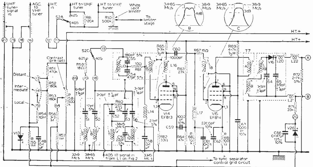
Fig. 4—The vision i.f. stages and vision detector circuit and the tuner switching arrangements. The i.f. stages are designed for the required 625-line passband and filters are switched into circuit to restrict the passband on 405 lines. The "distant", "intermediate" and "local" tappings alter the delay of diode V13.
