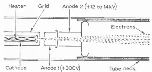
Fig. 2—This diagram illustrates the electron gun assembly of a tetrode picture tube.
