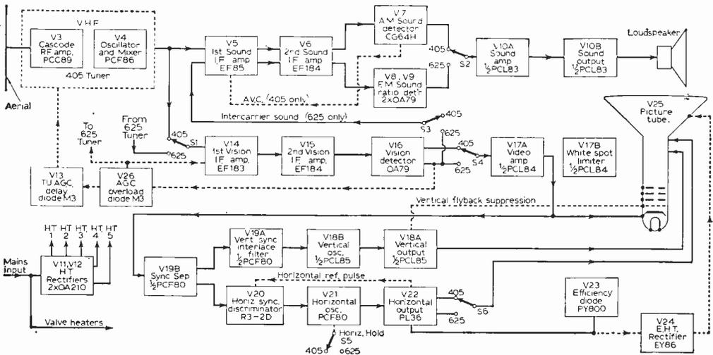
Fig. 1—Block diagram of the new Pye switchable Model V700D. Note that the stage references here correspond to those on the circuit sections.
