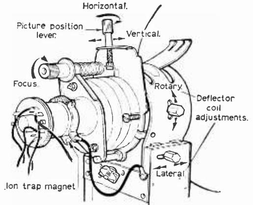
Fig. 8(b)—Picture adjustments provided on other Ferguson receivers.
