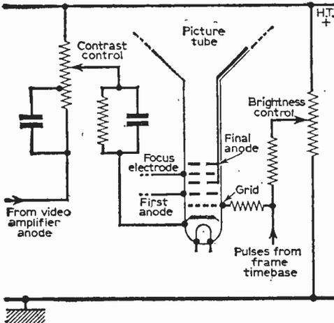
Fig. 28—The brightness and contrast controls of a switchable receiver. Note that the contrast is controlled by a “video drive” control in the cathode circuit of the picture tube. The brightness control is conventional and the flyback lines are suppressed by a signal from the frame timebase being fed into the control grid circuit.
