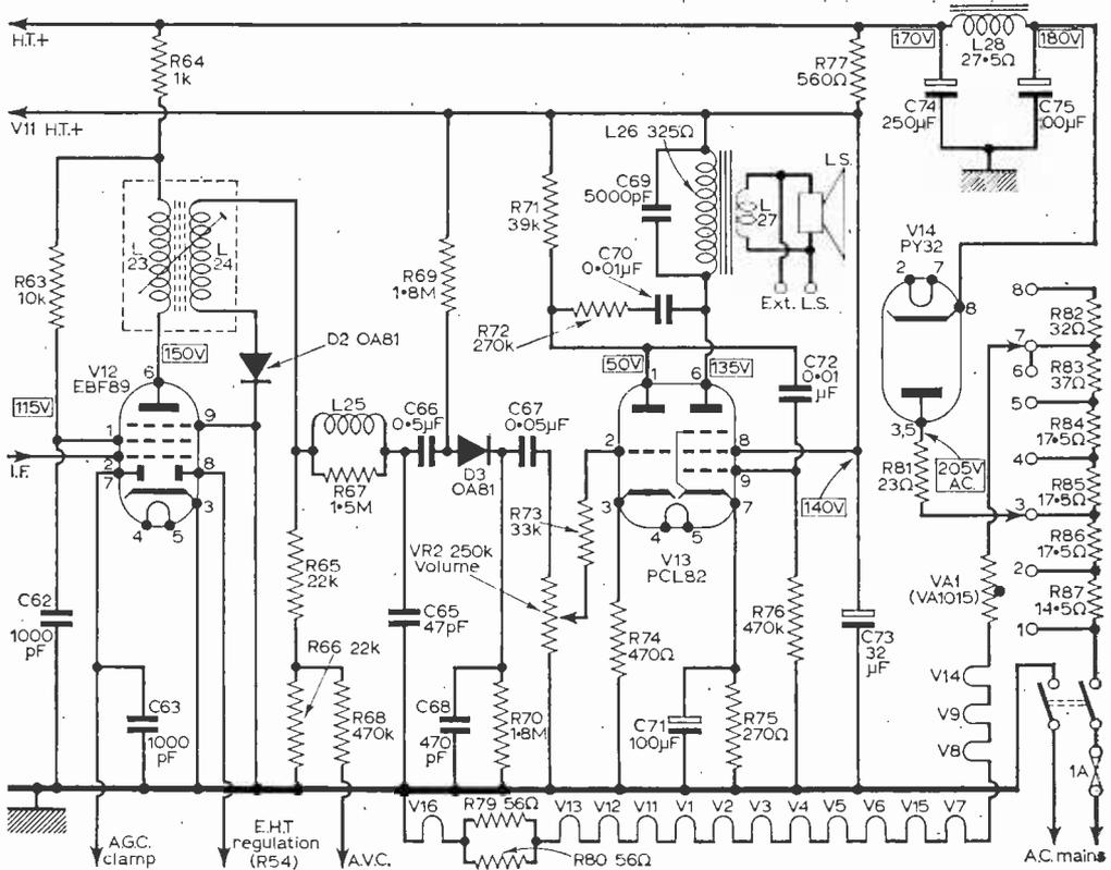
Fig. 5—The sound section and the power supply circuitry.
