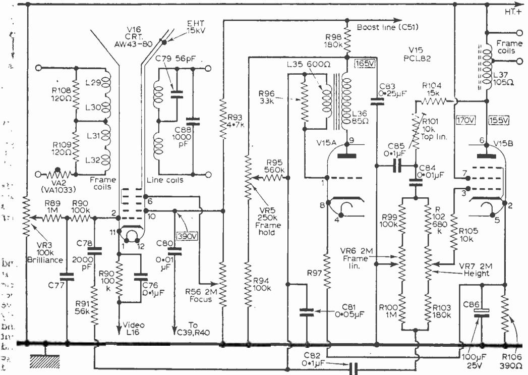
Fig. 4—The frame timebase and cathode ray tube circuits.
