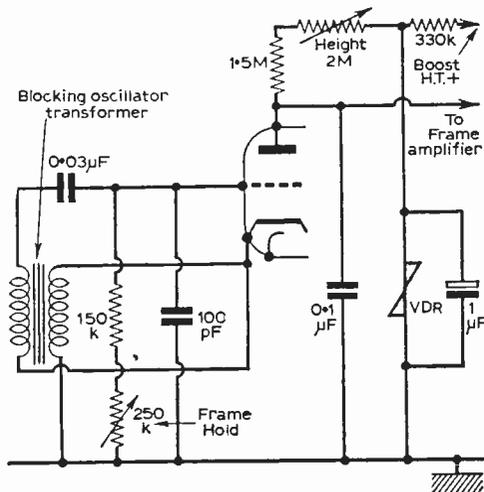
Fig. 4—In this circuit, a VDR is used to stabilise a frame blocking oscillator.
