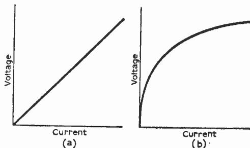
Fig. 2—The resistance of a normal resistor remains constant with variations in the voltage present across it; thus, the voltage/current characteristic is linear as shown in (a). With a voltage-dependent resistor, however, the resistance is not constant, but falls as the voltage across it increases. This gives a non-linear voltage/current characteristic shown in (b).
