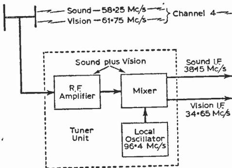
Fig. 1—A block diagram of the first two stages in a television receiver common to both sound and vision. The standard I.F.'s (e.g., sound at 38.15Mc/s and vision at 34.65Mc/s) are produced by the local oscillator operating above the signal frequencies, causing the sound I.F. to be higher than the vision I.F.
