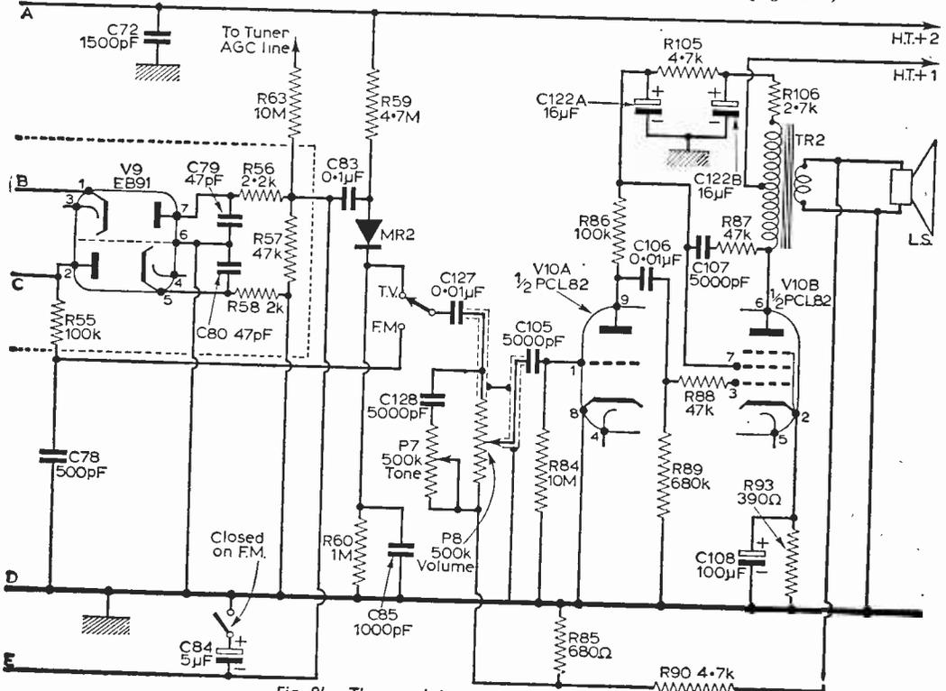
Fig. 8b—The sound detector and output stages.
