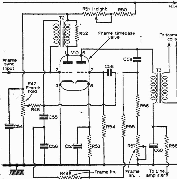
Fig. 30—Extra height can be obtained in the Masteradio series by (a) including R52— $47k$  and (b) increasing C56 from  $0.03\mu F$  by adding an extra  $0.01\mu F$  in parallel.
