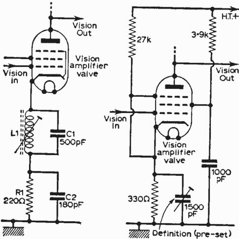
Fig. 8 (left)—The tuned circuit L1/C1 forms a dot pattern suppressor connected in the cathode circuit of the video amplifier valve.
