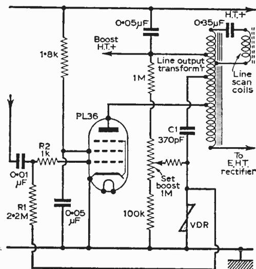
Fig. 5—Stabilisation of the line timebase is accomplished by the VDR producing a form of line output stage gain control voltage.
