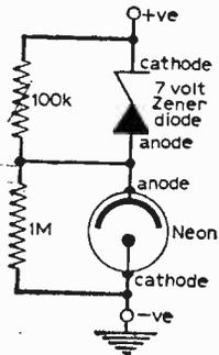
Fig. 6—To obtain variations of some 10 to 20V in the output voltage, the neon may be backed with suitable zener diodes in series.
