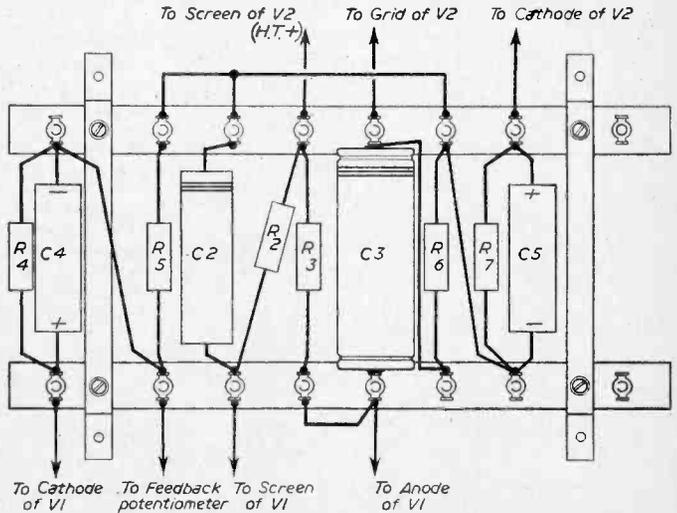
Fig. 3.— Wiring of the group board upon which the smaller parts are mounted.
