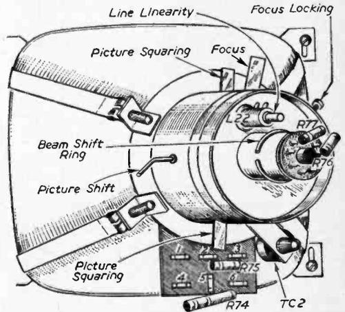
Fig. 5.—The tube unit (position of shift and L22 are different on some models).
