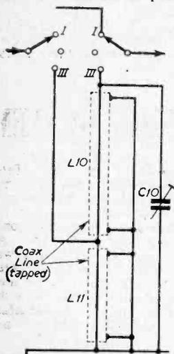
Fig. 4.—An alternative input circuit using coaxial lines with the input circuit tapped down this line for best results.
