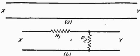
Fig. 1.—Diagram illustrating characteristic resistance of lines.
