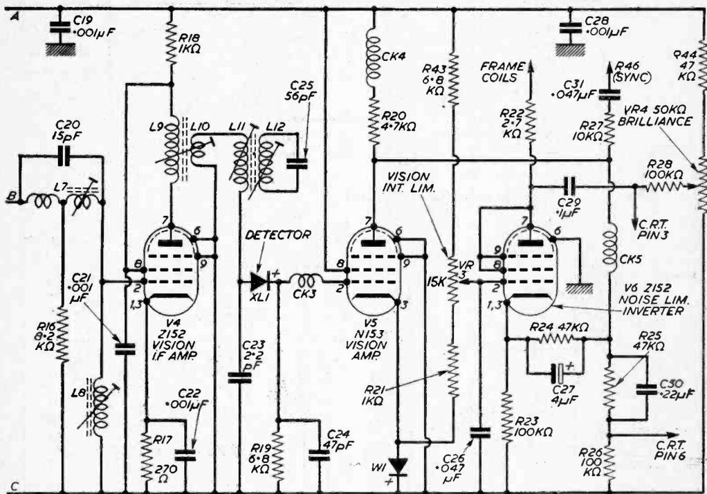
in a lack of voltage at the screen or anode and of course in the case of R13 the sound will also be almost entirely absent. These resistors often burn out as a result of a shorted 0.001 $\mu$ F decoupling capacitor or an internal short in a Z152 valve. Thus when a short is recorded at pin 8, before disconnecting the 0.001 $\mu$ F, always remove the Z152 to see if this is responsible after all.
