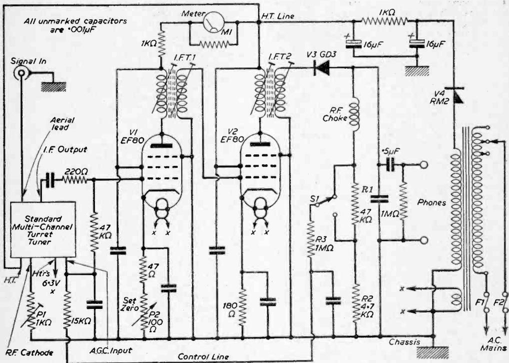
Fig. 3.—Circuit diagram of the signal strength meter for comparative tests.
