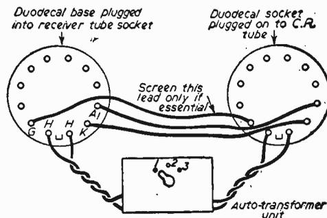
Fig. 3.—Typical arrangement of booster unit.
