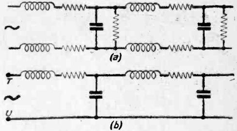
Fig. 7.—Circuits illustrating the characteristic impedance of lines.
