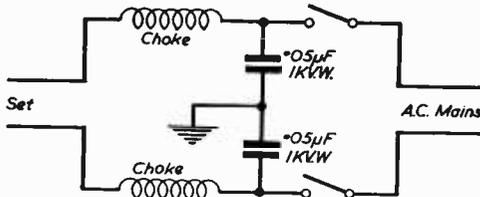
Fig. 5.—Preventing feedback to the mains by means of choke/capacitor network. This is similar to the Belling-Lee L300/3 filter unit.
