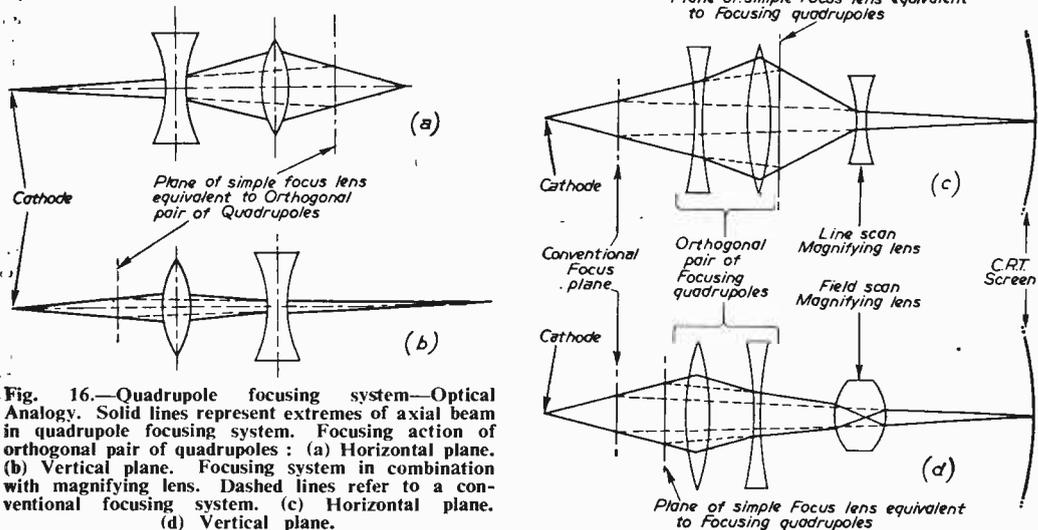
Fig. 16.—Quadrupole focusing system—Optical Analogy. Solid lines represent extremes of axial beam in quadrupole focusing system. Focusing action of orthogonal pair of quadrupoles: (a) Horizontal plane. (b) Vertical plane. Focusing system in combination with magnifying lens. Dashed lines refer to a conventional focusing system. (c) Horizontal plane. (d) Vertical plane.
