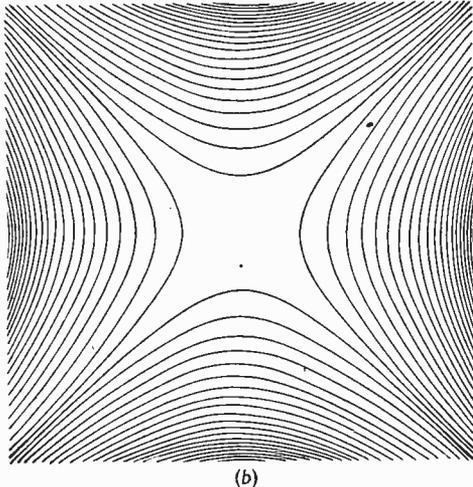
Fig. 18.—An adjustable quadrupole having pole shapes suggested by simple theory. (a) Isometric view. (b) Idealised field shape.
