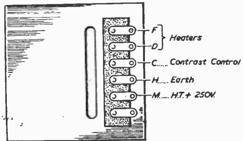
Fig. 3.—The terminal board at the rear of the tuner.
