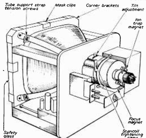
Fig. 12.—Details of the tube assembly on Models V14 and V14C. See notes above.
