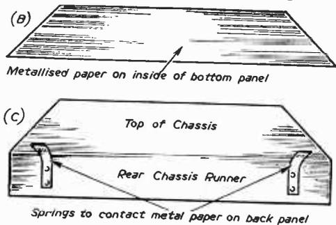
Fig. 2.—Lining the side of the cabinet with metallised paper or foil.
