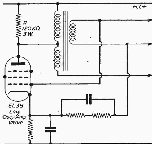
Fig. 3.—The basic line oscillator/output stage of Ferranti Model T1405S. If resistor R decreases in value, a critical line hold often results.
