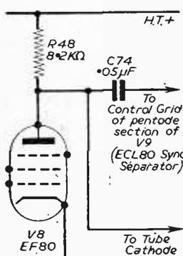
Fig. 2.—Part of the video amplifier stage of Ferranti Model 14T4. Loss of line and frame sync is caused if C74 goes open-circuit.
