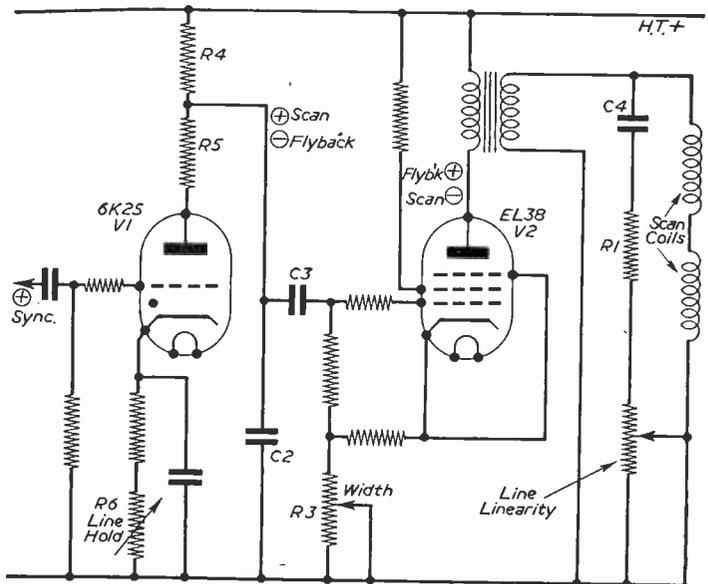
Fig. 24.—A thyratron timebase circuit.
