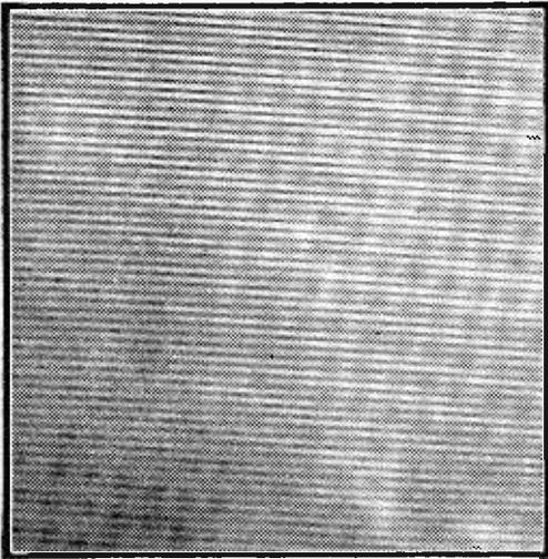
Patchett's Separator—a three-minute exposure of the camera indicates the high rigidity of scan which is obtained.
