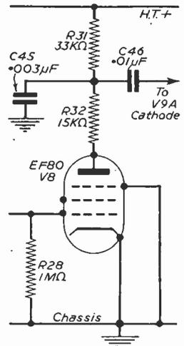
Fig. 1.—Basic circuit of the sync separator stage in Ferranti Model 14T3.
