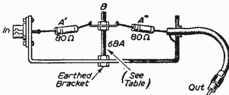
Fig. 5.—A length of screwed rod forms the  $B$  resistance in this arrangement. Note that the output lead screening is earthed.
