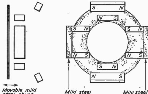
Fig. 22.—Adjustable magnifying lens having a field corrected to give good raster shape. Non-magnetic parts of the complete structure are not shown.
