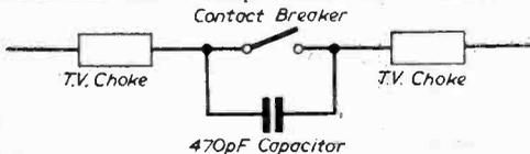
Fig. 2.—A suppressor system for thermostats.
