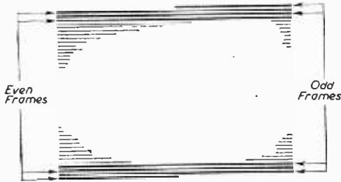
Fig. 3.—The lines of "odd" and "even" frames.
