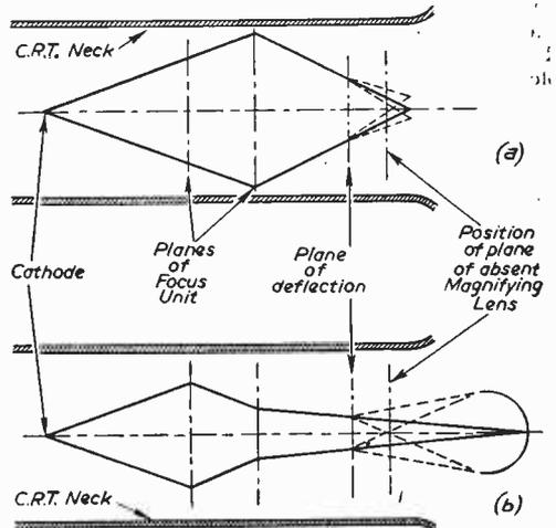
Fig. 19.—Action on electron beam of focusing and deflection systems without magnifying lens. (a) Horizontal plane—dotted lines show the effect of horizontal deflection. (b) Vertical plane—dotted lines show effect of vertical deflection.
