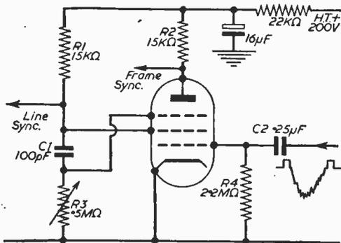
Fig. 6.—Flip-flop sync separator.
