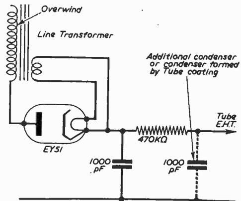
Fig. 1.—Additional smoothing provided by the tube coating.
