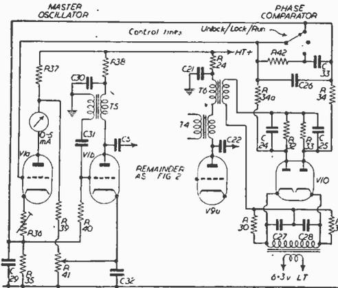
Fig. 3.—Mains locking circuit.
