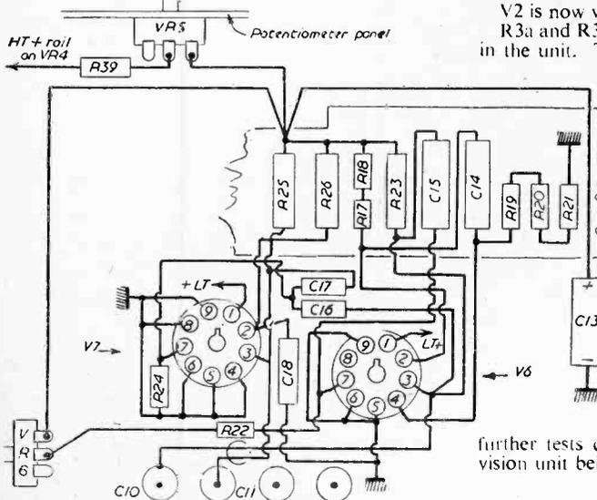
Fig. 10.—The frame circuit.
