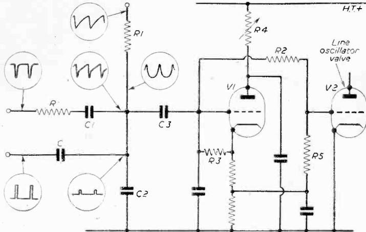
Fig. 3.—Basic circuit for the time-pulse system.
