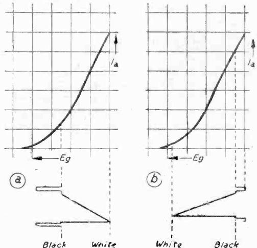
Fig. 1.—This illustration shows the picture content relative to the straight part of the valve curve.
