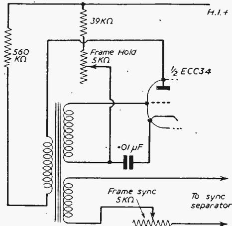
Fig. 18.—Method of sync coupling employed in the Pye D16T series.
