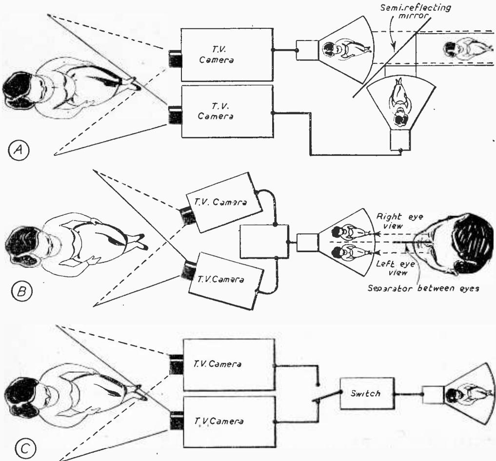
Three methods of producing television pictures in 3-D. A is the R.C.A. and Dumont system; B is the split image arrangement and C the synchronised shutter scheme.
