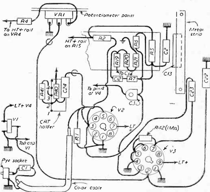
Fig. 11.—Sync separator and phase splitter.
