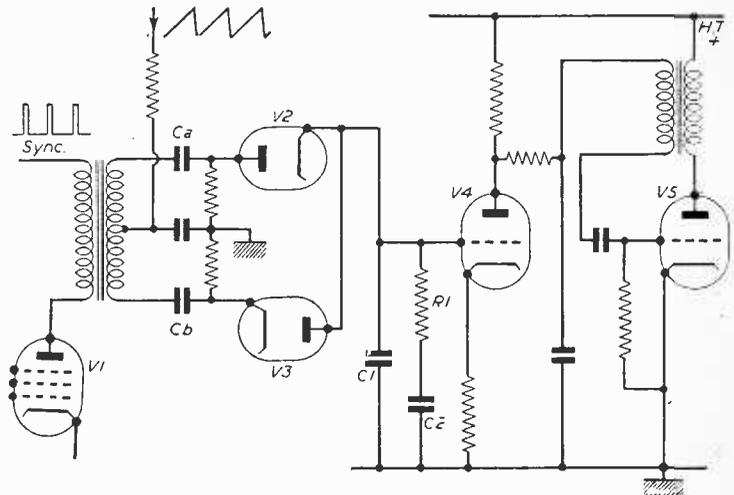
Fig. 1.—Basic circuit arrangement for auto sync control.
