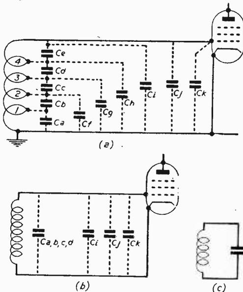
Fig. 1.—Diagram illustrating the stray capacities which exist in a circuit.
