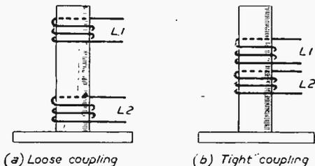
Fig. 3.—Loosely and tightly coupled coils.
