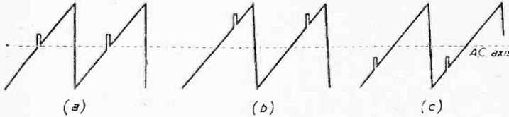
Fig. 2.—Position of sync pulse on the sawtooth waveform.
