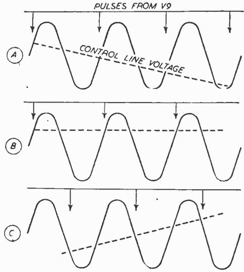
Fig. 4.—Action of phase comparator.
