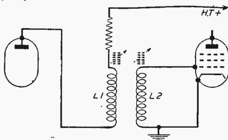
Fig. 2.—Stray couplings in a loose-coupled circuit.
