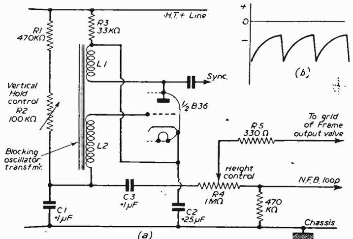
Fig. 16.—This frame generator section is used in the G.E.C. BT2147 series, and the voltage waveform across C1 is shown at (b).
