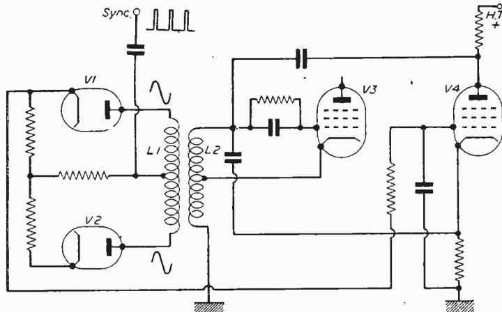
Fig. 5.—Basic circuit for the sine system.
