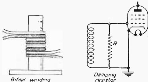
Figs. 4 and 5.—Bifilar winding and method of broadening tuning.
