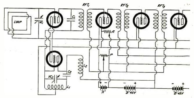
A SCHEMATIC DIAGRAM OF THE ULTRADYNE FIGURE 2: The detailed hook-up of the Ultradyne superheterodyne receiver which is described below. The lettering of the apparatus in the drawing corresponds with that in the printed list of parts.
