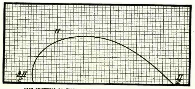
THE SECTION OF THE SPIRAL FOR BROADCAST FREQUENCIES FIGURE 6: This section of the curve gives the plate shape for obtaining a 3:1 frequency ratio. It would tune in stations having frequencies between 500 and 1,500 kilocycles, which is approximately the broadcast range.
