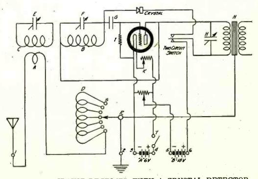
THE FOUR-CIRCUIT RECEIVER WITH A CRYSTAL DETECTOR FIGURE 1: This schematic diagram shows how the change from a vacuum tube to a crystal detector may be made in the Four-circuit receiver. All the lettering in the drawing is identical with that employed in the original diagram of the receiver.
