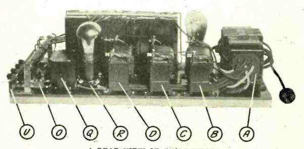
A REAR VIEW OF THE DEVICE FIGURE 2: This illustration shows the general location of the transformer, tubes, chokes. condensers and resistances.
