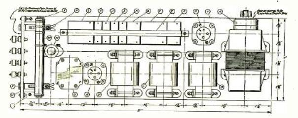
THE WORKING DRAWING FOR CONSTRUCTION FIGURE 4: This diagram gives the correct dimensions and spacing for mounting all of the component parts of the power-pack amplifier.
