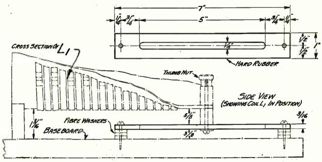
THE CONSTRUCTIONAL DETAILS OF COIL LI
