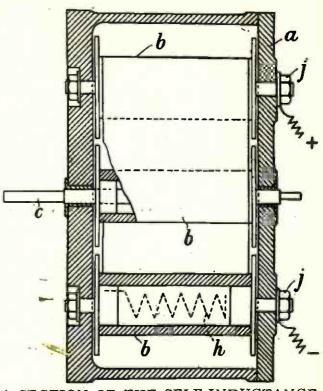
A SECTION OF THE SELF-INDUCTANCE FIGURE 2: This diagram shows how the convolutions of the coil wind about the three roller cores of this new variable self-inductance.
