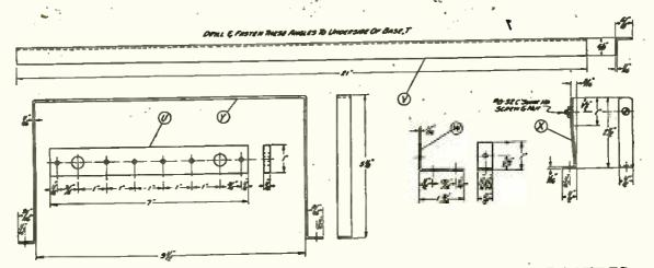
DETAILS OF THE CONNECTION BLOCK, BRASS STRIPS AND BRACKETS FIGURE 6: This drawing gives the necessary data for making the insulating strip on which the binding posts are mounted. It also gives the dimensions for the reinforcing angles and the small brass brackets which are used to fasten the condensers, the connection block and the resistance in place.
