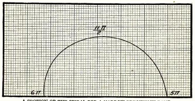
A SECTION OF THE SPIRAL FOR A NARROW FREQUENCY BAND FIGURE 8: This section of the curve shows the plate shape for covering a 6:5 frequency ratio. A condenser of this type would place stations between 500 and 600 kilocycles a uniform distance apart on the tuning dial.
