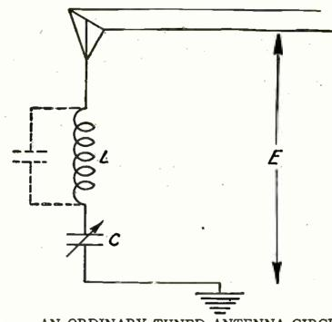
AN ORDINARY TUNED ANTENNA CIRCUIT • FIGURE 1: This is an example of a tuned circuit which has the voltage introduced in a part of the circuit exterior to the coil. Broadcast receivers generally make use of an untuned antenna circuit.
