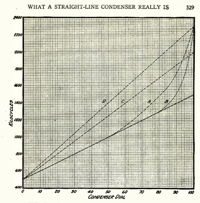
THE TUNING CURVES FOR THE CONDENSERS OF FIGURE 13 FIGURE 14: The curves A and B show that the capacity curves cover a much greater frequency ratio than 3:1 and that they are no longer straight-line-frequency curves when they are modified to obtain a low minimum capacity. Curve D is the only straight-line frequency variation between the maximum and the modified minimum.
