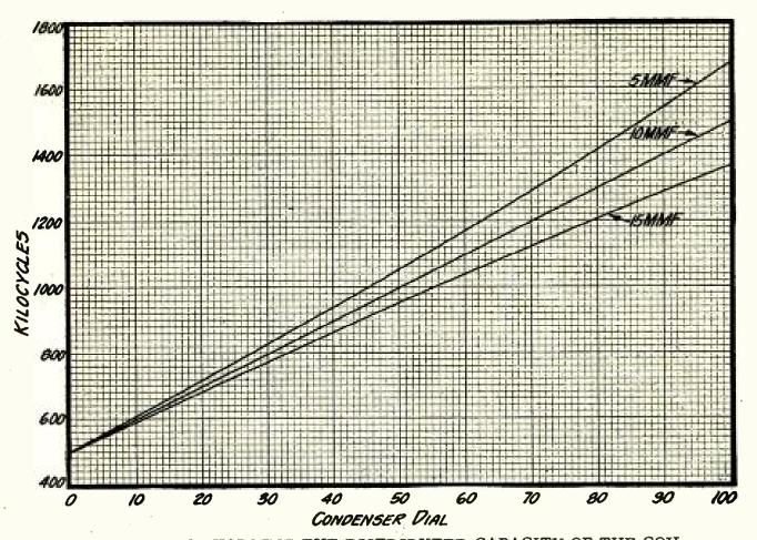
THE RESULT OF VARYING THE DISTRIBUTED CAPACITY OF THE COIL FIGURE 12: The central curve is for a condenser designed to give straight-line-frequency tuning when used with a coil having a distributed capacity of 10 micro-microfarads. A coil having 5 micro-microfarads capacity will extend the frequency range, while one having 15 micro-microfarads will limit it below the range desired.
