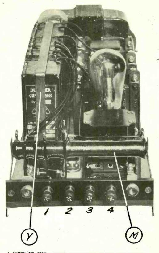
A VIEW OF THE POWER-PACK UNIT FROM THE RIGHT FIGURE 5: The unit with the Ward Leonard resistor in place. Notice the input and output jacks and the binding posts which supply the voltages for the set that the unit is used with.
