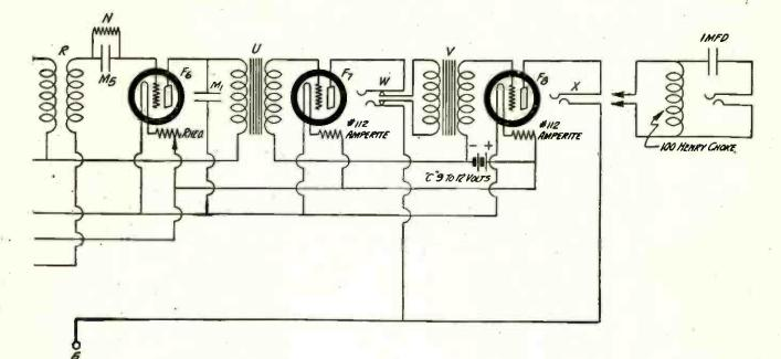
effected by connecting one side of a small midget condenser to the plate terminal of the detector tube, and the other side to the lower terminal of the loop.
