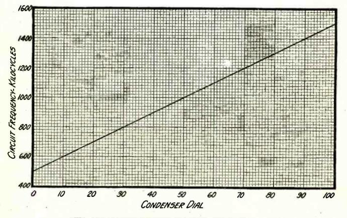
THE STRAIGHT-LINE-FREQUENCY TUNING CURVE FIGURE 9: This chart shows the curve for a tuned circuit which has the correct capacity to spread the frequency bands uniformly over the one hundred divisions of the condenser dial.
