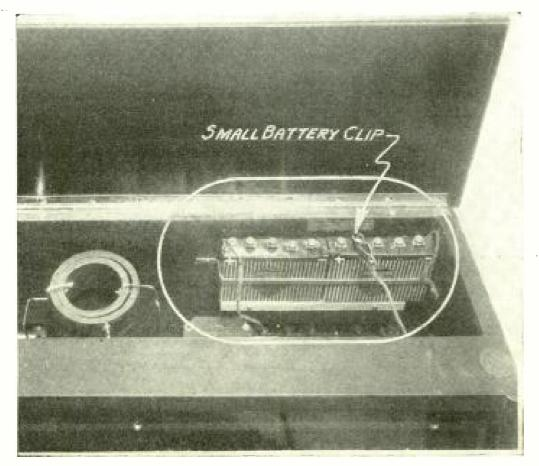
THE "C" BATTERIES INSTALLED IN THE CABINET FIGURE 3: A small wood shelf is mounted directly on the rear wall of the cabinet. The batteries are placed on this and are held in place by a piece of  $\frac{1}{16}$  by  $\frac{1}{2}$ -inch brass strip, bent to proper shape. A small battery clip may be used conveniently to make an easily adjustable negative connection.
