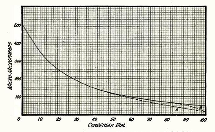
THE CAPACITY CURVES FOR A 500 MICRO-MICROFARAD CONDENSER FIGURE 13: The solid line is a curve for a straight-line-frequency condenser having a 3:1 frequency ratio. Note the relatively high minimum capacity. Curves A and B show methods of modifying the capacity curve to get a low minimum, but they only use 80 and 90 percent of the dial respectively.
