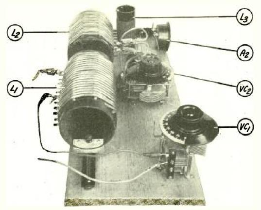
AN END VIEW THAT SHOWS THE COIL MOUNTING
