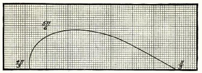
A SECTION FOR COVERING A WIDE FREQUENCY RANGE FIGURE 7: This section of the curve has been selected to cover a 4:1 frequency ratio. Plates of this shape would spread a band of stations between 500 and 2,000 kilocycles uniformly over the tuning dial.
