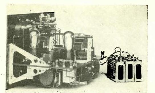
A VIEW OF THE SET WITH THE CABINET REMOVED FIGURE 4: The "C" batteries which are connected with the flexible leads have been added to accomplish a saving in total "B" battery drain and also to improve quality on strong signals.
