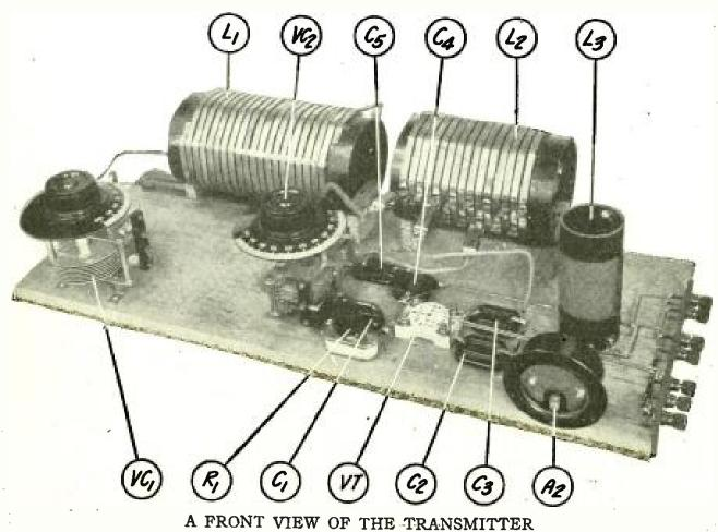
FIGURE 2: This illustration gives a good idea of the layout and spacing of the instruments. The designating symbols shown correspond exactly with those in the other figures and in the list of parts given above. The coil L2 is fastened to the baseboard by means of screws run through from the bottom of the baseboard into the coil mounting blocks.
