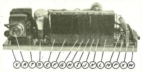
A FRONT VIEW OF THE UNIT FIGURE 3: The bank of condensers, the rectifier tube and the power transformer with its "on" and "off" switch that also gives three power ranges are shown here.
