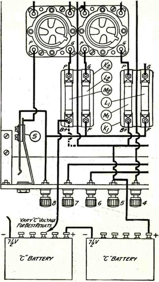
A PICTURIZATION OF THE CHANGE SHOWN IN FIGURE 2 FIGURE 4: A section of the original diagram which was printed on page 505 of the December, 1925, issue of POPULAR RADIO, showing the changes which must be made in connecting the "C" battery into the circuit.
