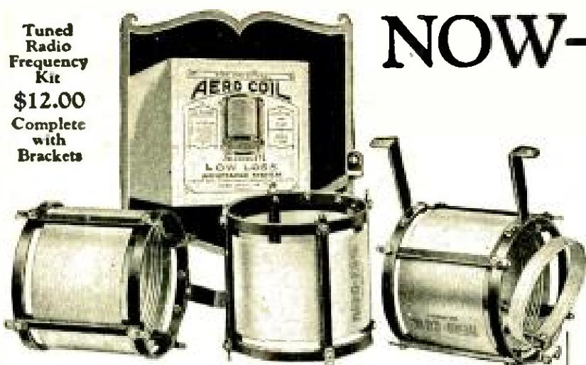
The complete Low Loss Inductance System, comprising two tuned circuit transformers and an antennae coupler with a uniquely constructed variable primary for governing the selectivity of the antennae circuit.
