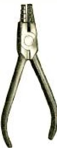
A complete and handy tool for electricians, radio set builders and mechanics. It will accurately form loops or eyes for No. 4, 6, 8 and 10 screws, make easy radius and sharp right angle bends, has flat jaws and wire cutters. This tool is made of the best quality steel, dropped forged and carefully tempered in oil.
