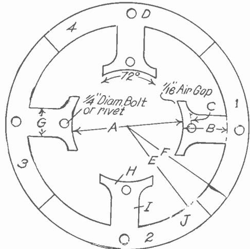
FIG. 9. FRAME OF FOUR-POLE DYNAMO OR MOTOR
