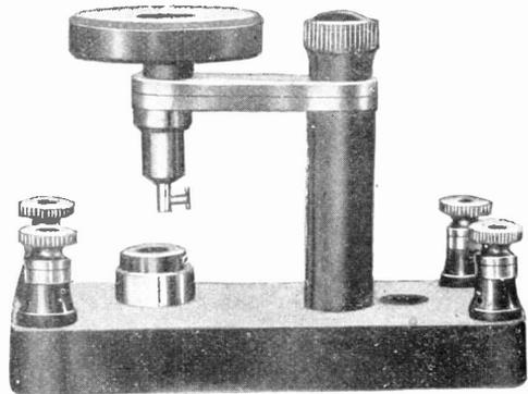
FIG. 115. ELECTROLYTIC DETECTOR
