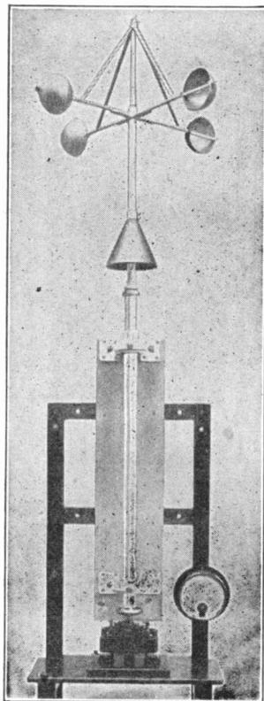
ELECTRICAL WIND MEASURING INSTRUMENT
