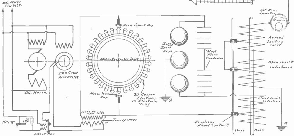
FIG. 5. DIAGRAM OF SECONDARY CONNECTIONS
