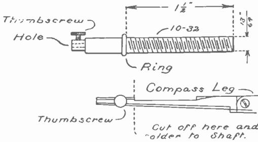
FIG. 122. SHAFT FOR HOLDING WIRE
