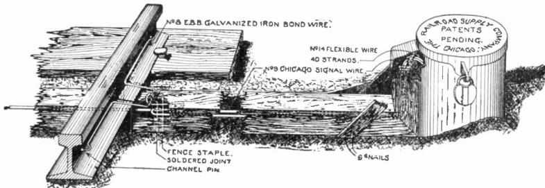
FIG. 11. CONNECTIONS BETWEEN TRACK CIRCUIT AND BATTERY CHUTE
