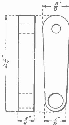
FIG. 120. BRASS ARM, SIDE VIEW AND PLAN
