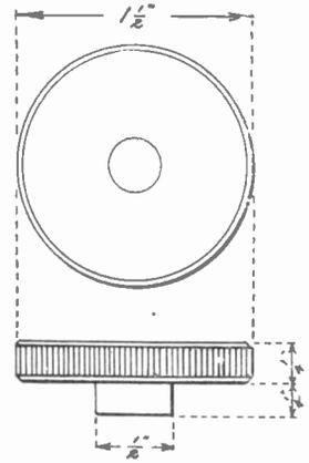
FIG. 118. ADJUSTING SCREW HEAD
