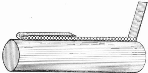
METHOD OF WINDING MAGNET COIL
