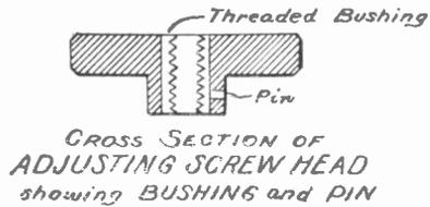
FIG. 119. DETAILS OF SCREW HEAD AND BUSHING
