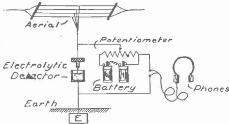
FIG. 114. CONNECTIONS FOR ELECTROLYTIC DETECTOR
