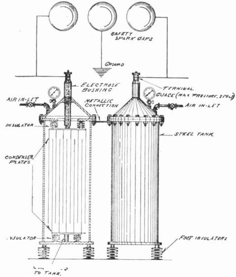
FIG. 4. SIDE VIEW AND CROSS SECTION OF CONDENSER
