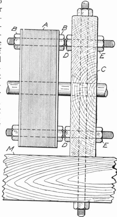
FIG. 7. BEARING BLOCK AND WORK HOLDER
