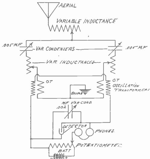
FIG. 6. RECEIVER CONNECTIONS
