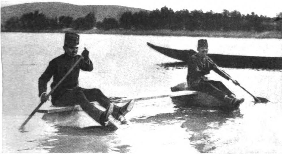
Air bags connected with a beam used as substitutes for boats by soldiers of a Vienna regiment.
