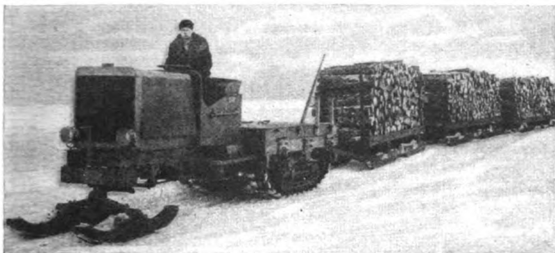
The auto log hauler is being used extensively by Maine lumbermen. The machine weighs ten tons and each car carries about four horse loads.
