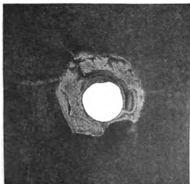
What the Vicious, Steel Jacketed Bullet of the New .22 Caliber Will Do to a Steel Plate 1/4 Inch Thick
