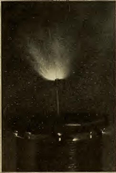
FIG. 2. DISCHARGE OF A TESLA COIL.
