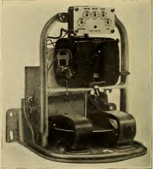
FIG. 30. RECORDING WATTMETER.
