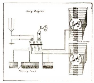
Wiring Diagram for the Inductive Tuner.
