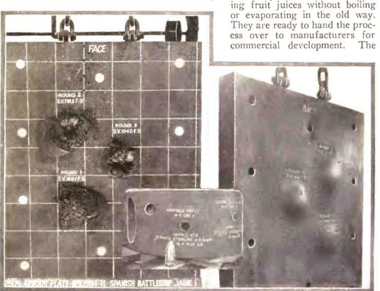
The Effect of Modern Shells on Steel Armor Plates: At the Left is an Armor Plate of the Spanish Battleship "Jaime I," Which Was Damaged by Fourteen-Inch Shells.
