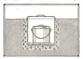
pail and the earth surrounding it a thick layer of coal ashes should be poured and tamped. The smaller pail is placed within the larger one, as shown, upon a layer of tamped ashes. The cover of the large pail is elevated a short distance.
