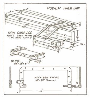
pitman wheel is ten inches in diameter. An eight-inch stroke is about the proper length for ordinary work with a 12" blade in the frame. A shorter or longer stroke is easily obtained by varying the location of the 5/16" x 1½" lag screw which is used to fasten the end of the pitman rod to the wheel.
