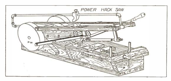
maple or other hard wood. The metal parts are mostly of mild steel, excepting, of course, the cold rolled shaft and the vise screw. Inasmuch as there are no hard joints to make, the wood parts may be very quickly gotten out and fastened together.
