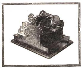
A Partial Rear View of the Set: The Black Inductive Tuner Spools may be Seen, as well as the White Spool of the Loading Coils.
