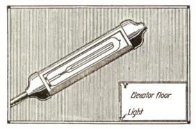
as shown in the accompanying drawing. The lamp should be attached to the floor of the car by means of a crow-foot, and connected so that it will light when the elevator is stopped. This can be accomplished by making an extra connection or two at the starting switch.
