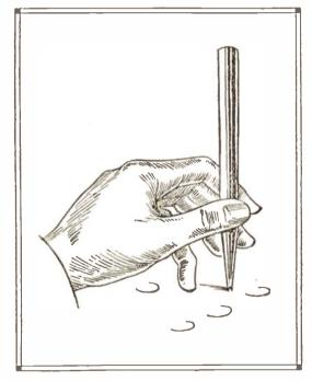
the centering of flange or shear lines which are usually centered with two marks close together for the purpose of distinguishing between the center marks for holes and those of the shear or flange lines. The idea is made clear by the illustration.
