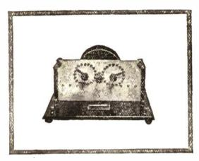
Especially Intended for Amateur Use, this Inductive Tuner is Designed along the Same General Lines as the Automatic Receiving Set. It is, However, Manually Operated
