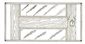
can be made "tamper-proof" by screwing two springs above the bolt, so that when the bolt is withdrawn from them they are separated. If the springs are placed in an electric circuit composed of dry cells and a doorbell, when the lock is tampered with, the bell will sound an alarm.
