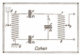
Wiring Plan of the Cohen Circuit for a Multiple Tuner,
