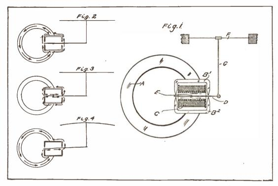
A Schematic Drawing of a Telephone Receiver of New Design, as well as Diagrams of the Magnetic Circuits and their Effects on the Diaphragm at Different Periods in its Operation.
