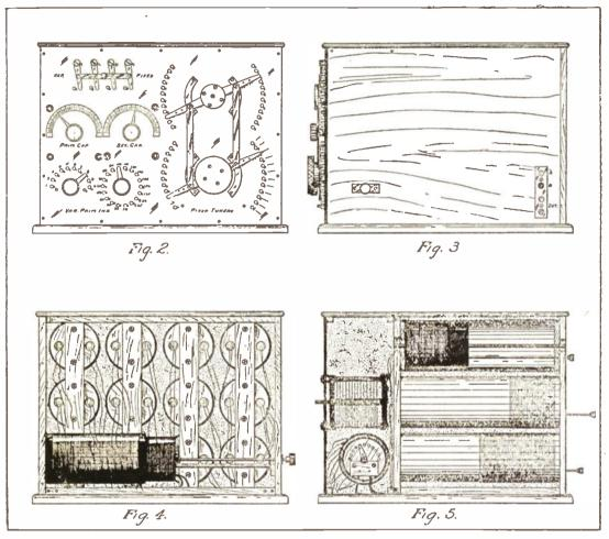
Views of the Exterior and Interior of the Inductive Tuner, showing the Location of the Different Parts.
