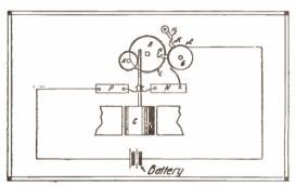
Diagram of the Working Parts of an Electric Clock that will Run for Three Years without Attention.
