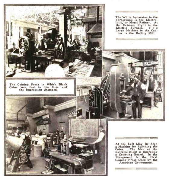
catching the blank between the two dies as they come together. The pressure exerted amounts to 160 tons, which stamps at the same time the impressions the number of pieces is instantly known. Much time is thus saved, since it is unnecessary to count each coin individually. This completes the process, for the
