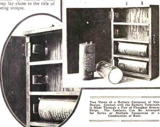
The contact device in this container consists of a pair of phosphor bronze spring strips, one of which makes congraphic plate and allowing a perfectly vertical beam of the rays to fall from the bulb above, through a special tube so as to properly direct the rays on to the object.
