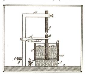
hole in the end of the arm, L, which is locked to the standard. This arm should be insulated, as shown, by a fibre joint. The self-operating device consists of a glass vessel, f, around the upper part of which a layer of heavy magnet wire (No. 14 is large enough) is wound. The vessel is nearly filled with mercury. The carbon, B, fits in a heavy iron sleeve which sinks into the mercury until its weight and that of the carbon and holder are displaced.
