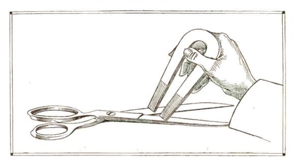
shoe magnet can be employed for magnetizing any pair of scissors. To magnetize the scissors the two poles of the magnet are placed in contact with the scissors near the pivot, and drawn to the end of the blades. This operation is repeated several times, care being exercised that the same poles of the magnet touch the same blades of the scissors.
