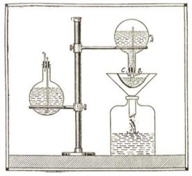
the top of the funnel. The solution runs out of tube C until the rising liquid closes the end B, thus automatically checking the flow. This goes on continually until the whole of the solution has been filtered.
