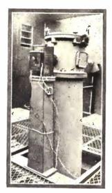
The "Wabble" of the North Pole is Detected and Recorded by This Instrument.
