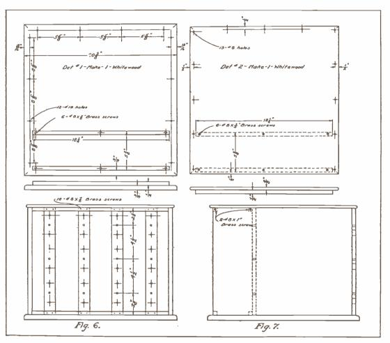
Details of the Case for the Inductive Tuner. It is Best to Use Mahogany or Oak, although a Good Grade of Whitewood can be Substituted.
