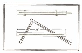
tions given. This pitch board and template may be used on other work than building stairs—laying out trusses, rafters, braces, etc.
