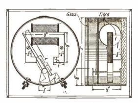
coil in the right hand, so that the fingers encircle it in the direction of the north pole. The dial may be divided in any way, to indicate the direction of the current.
