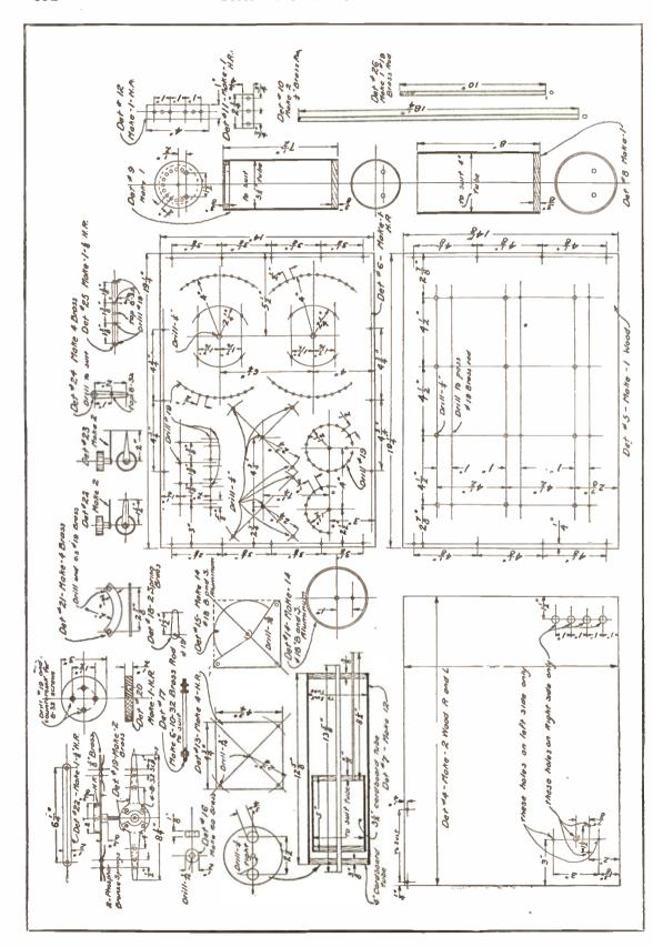
Detail No. 21 shows the contact strips for the switch levers in detail No. 19.
