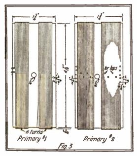
The Two Primary Coils, Showing the Method of Winding.
