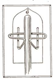
p a n y i n g drawing a n d fastened with b r a d s to a small w o o d block which may be suspended from a screw-eye driven in the wall. The wood can be p a i n t e d to m a t c h surroundings.
