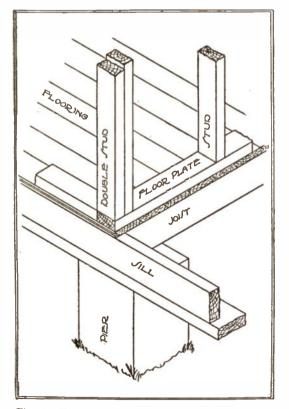
Fig. 12-Showing the Construction of the Framing at Floor.
