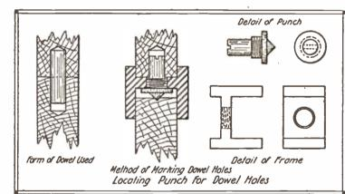
The device is inv a l u a ble for marking off dowel holes in the edges of boards used for table tops and in other places where it is e ssential that accu-
