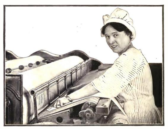
A Little Steel Fence Along the Entire Length of the Roller Prevents the Worker's Fingers from Being Caught in the Mangle or Ironing Machine.
