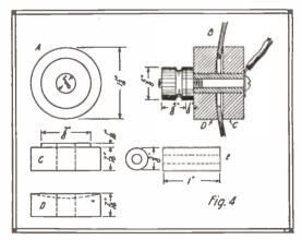
Details of the Binding Posts and Insulated Bushings.
