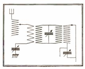
Wiring Diagram of a Simple Marconi Multiple Tuner, Showing Relation of Different Windings and Condensers.
