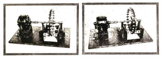
Figs. 3 and 3a.—Two Views of the New Rotary Spark Gap Which Has a Total of Eight Separate Gaps Connected in Series.
