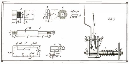
Different Members of the Hot Wire Ammeter Movement, as Well as a Side View of the Movement When Assembled.
