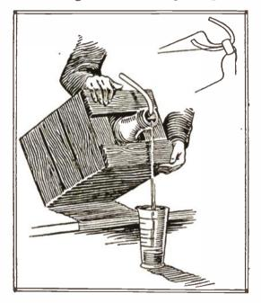
phuric acid from a carboy can be avoided if a bent glass tube is inserted into the neck of the bottle so that the partial vacuum caused by the liquid gushing out is equalized.
