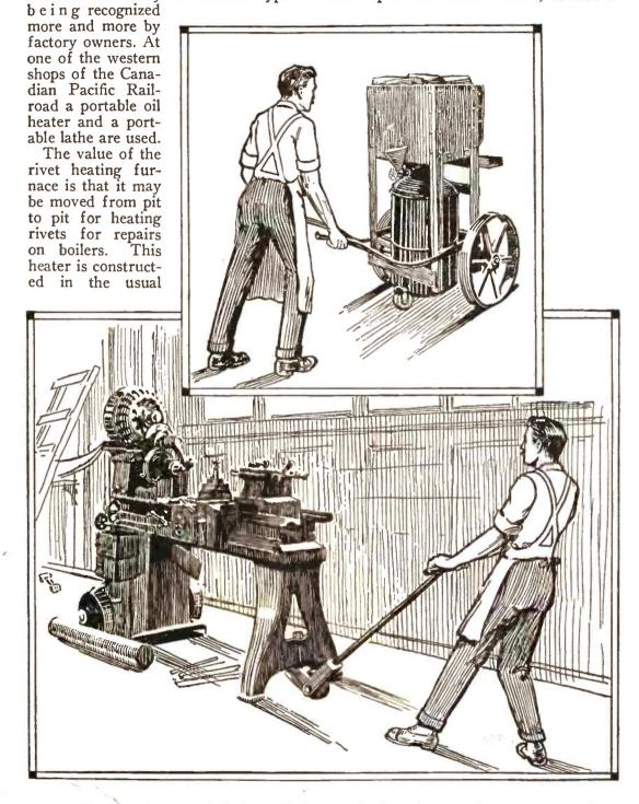
way, with the oil reservoir below. It is can be hurriedly pushed to a convenient carried from place to place in wheel spot in case of an emergency. barrow fashion, being provided with Contributed by P. W.
