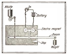
the armature is drawn down, a catch at its lower end releases the weighted beam, and the whistle blows until the beam is put back in place.
