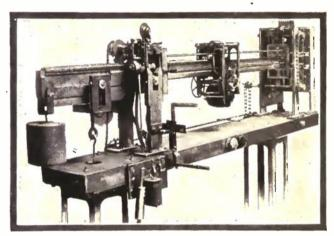
A Scale in which Electricity Does all the Work, Both Automatically Weighing Truck Loads and Keeping a Permanent Record.
