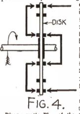
of *n* short gaps is practically the same (in some cases less than) that required to bridge a single gap n times as long. Thus, subdivisions of the total discharge favors the suppression of an arc, yet requires no additional potential to produce
