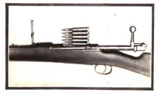
A Mauser Rifle and a Clip of Ammunition Ready to be Inserted into the Magazine. The Clip Method of Loading is Used in Most Military Weapons of Today.
