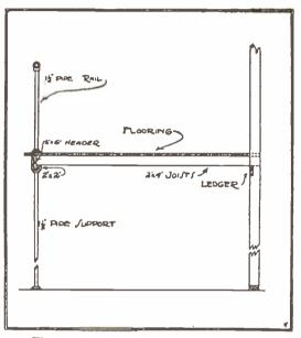
Fig. 19-Detail of Balcony Construction.
