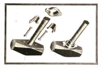
A New Type of Sledge Hammer in which the Danger of a Loosened Head is Entirely Eliminated.
