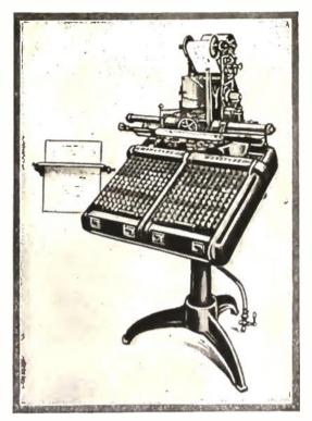
A Monotype Keyboard which Perforates a Paper Ribbon that is Afterwards Placed on the Casting Machine.
