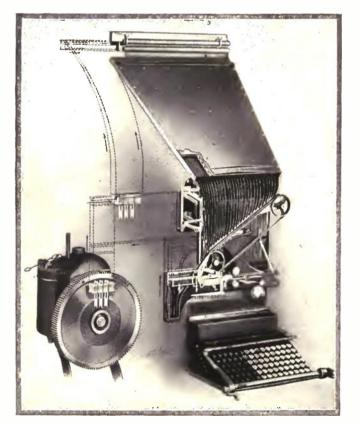
A Diagrammatic View of the Main Parts of the Linotype Machine, Showing the Various Steps in One Complete Cycle of its Operation.
