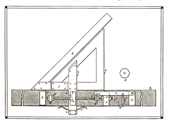
screw, J, which passes through the block H, and is held in position by the nuts, K. The rachet, W, is held in place by the hexagonal nuts, L.
