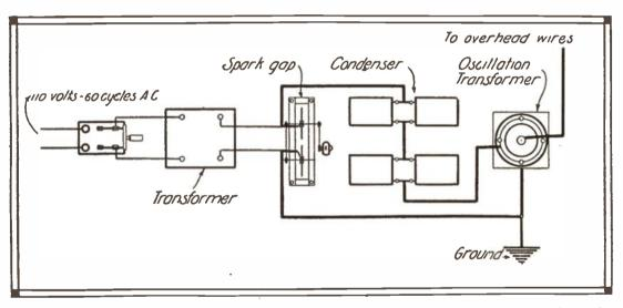
Wiring Diagram for the Connecting of the Various Pieces of Apparatus to be Used in Electrical Plant Culture.
