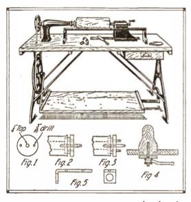
about 4 in. wide and as long as the This tail stock. should be hinged at the back to the bottom of the tail stock and provided with a bolt having a handle passing through at the front into an imbedded nut in the tail stock. The dead center can be made of a bolt. pointed at the end, turning through two imbedded nuts. with a small wheel or handle of some
