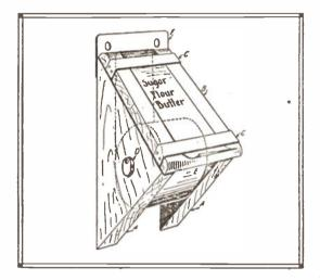
wooden or metal rod to hold a roll of paper, such as is used in adding machines, or any other roll of paper that may be obtainable—the roll determining the size of the parts for the holder.
