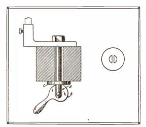
have a slot at one end to admit the cam, B. The washer, C, should be cut at the center to fit loosely over the slotted bolt. Contributed by M. A. PIPER.
