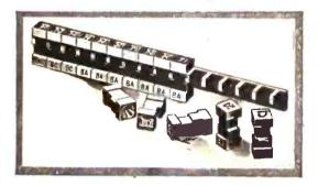
Matrices or Moulds of the Monotype Caster, Showing the Method of Holding Them in a Frame.
