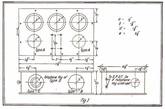
Dimensioned Plan of the Cabinet in Which is Placed the Different Apparatus Comprising the Multiple Receiving Tuner.
