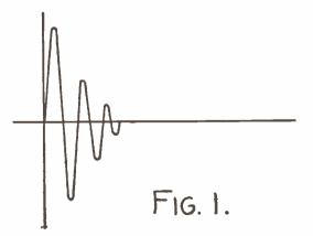
Highly Damped Oscillations Produced by a Parallel Plate Quenched Gap. ther experience led to the utilization of resonance in the transformer circuits, the inductance in the circuit preventing the heavy rushes of current necessary for maintaining the arc.
