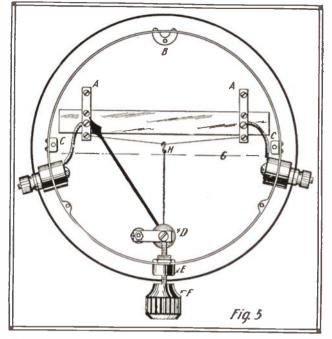
Front View of the Working Parts of the Hot Wire Meter as It Appears When Finished.
