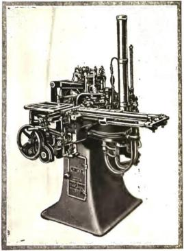
A Monotype Caster which Sets Up the Type According to the Arrangement of the Perforations in a Paper Ribbon.
