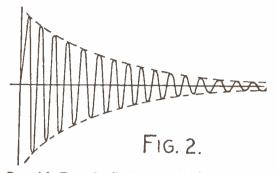
Powerful Free Oscillations of Single Frequency Induced in the Aerial by a Highly Damped Oscillation Circuit.
