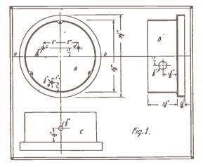
The Details of the Case for the Hot Wire Meter.
