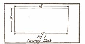
Forming Block on Which the Cardboard or Sheet Fibre is Placed.
