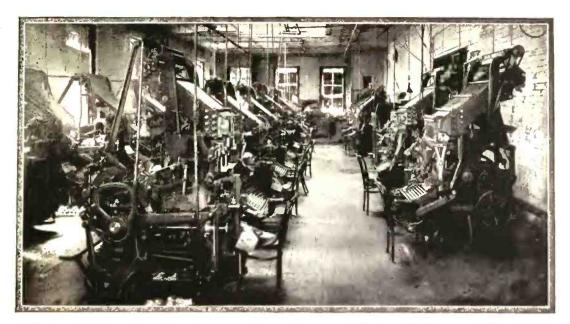
A Typical Newspaper Composing Room, in which a Number of Linotype Machines are being Used to Set up the Reading Matter. Many Linotypes are required by Every Daily Newspaper, Because of the Vast Amount of Type Matter that Must be set up within a Limited Time.
