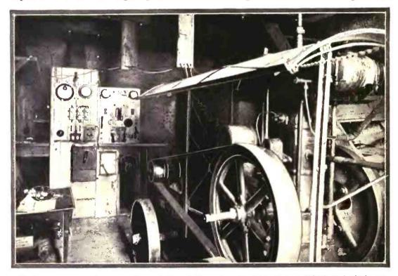
The German Army is Using this Type of Electric Generating Plant Mounted on Wheels and which can be Immediately Installed at Any Desired Point for Supplying Current for Illumination and Other Purposes.
