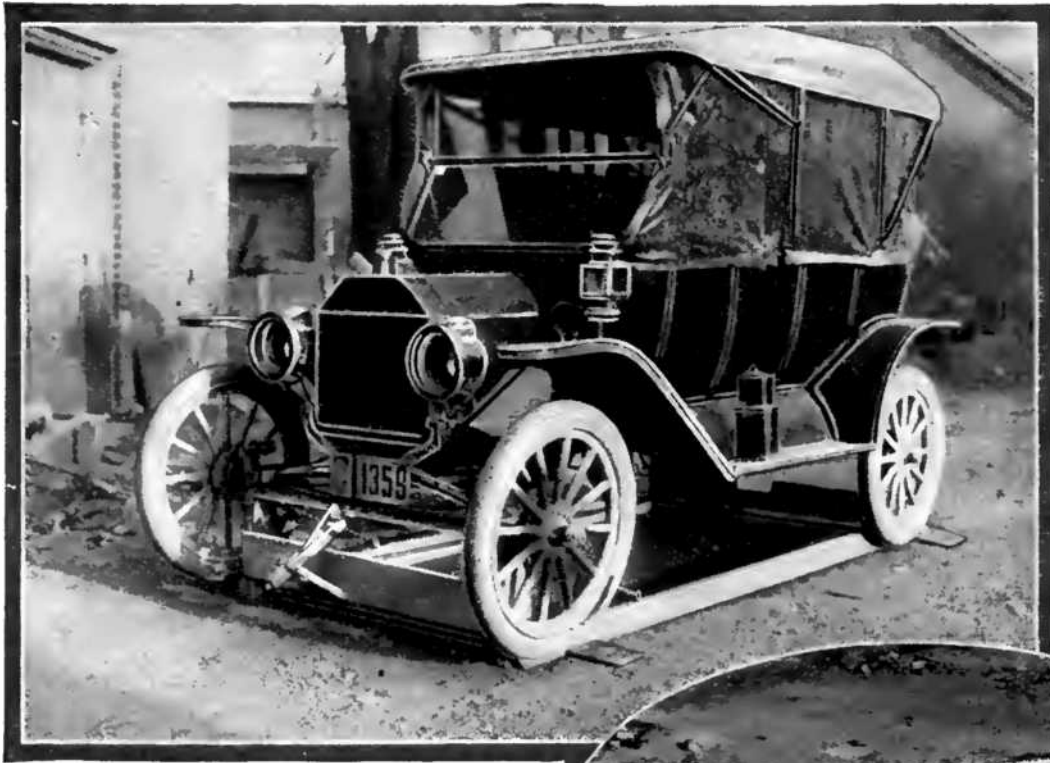
An Automatic Automobile Jack Invented by an American. As the Car Rides Over the Mechanism, It Is Lifted Off the Ground by Arms Pressing Against the Axles.
