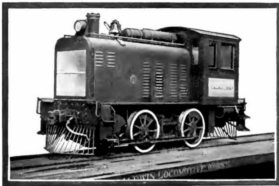
A Type of Locomotive That Is Designed Along the Same Lines As an Automobile. Its Tractive Power Is Developed by a Four-cylinder Engine That Uses Either Gasoline or Kerosene for Fuel.
