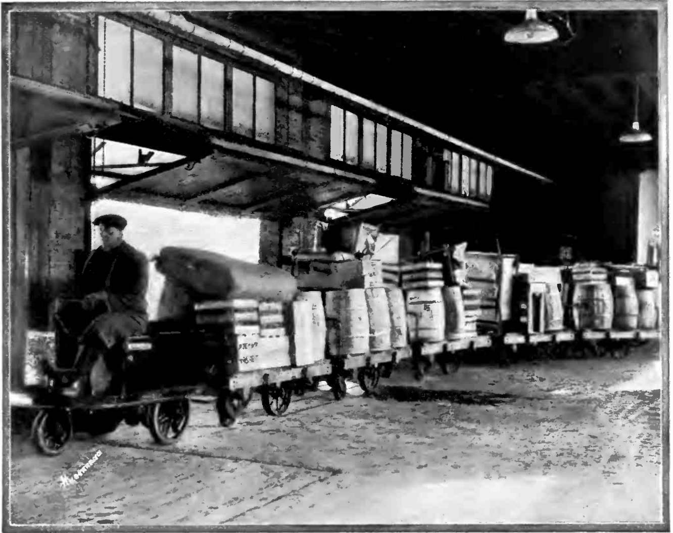
A Storage Battery Tractor Being Employed to Haul Loaded Trailers About a Dock.
