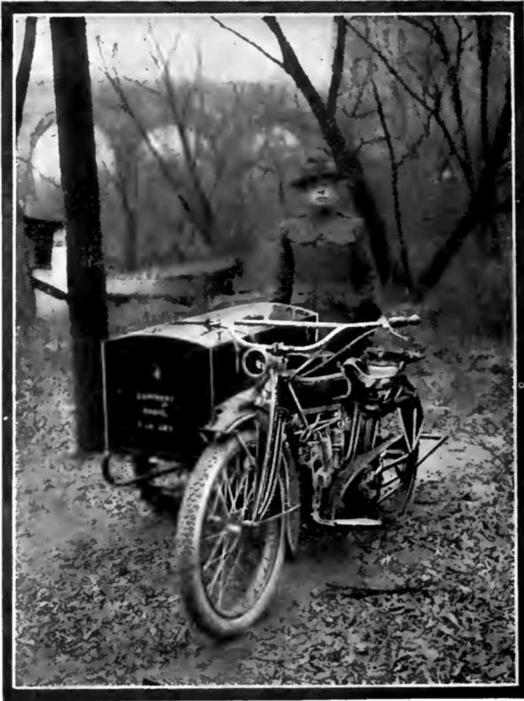
A Wireless Telephone Set That May Be Carried About in a Motorcycle Side Car Bids Fair to Become an Important Factor in Military Operations.
