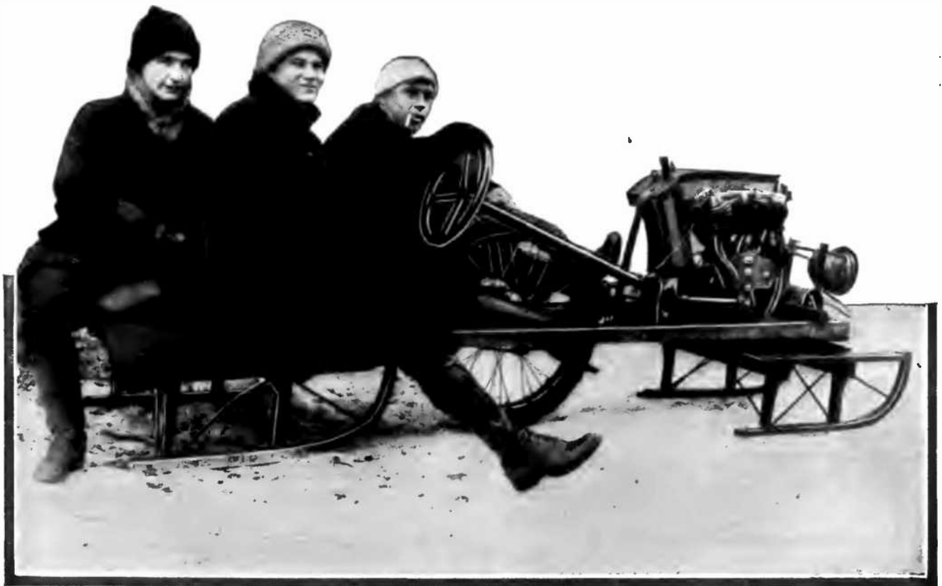
The Engine of a Motorcycle Being Put to Good Use During the Wintertime When the Roads Are Not Favorable to Motorcycling.
