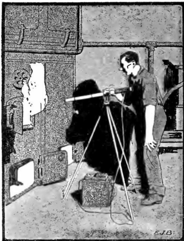
The Heat of a Flame Cannot Be Determined by the Human Eye; a Pyrometer is Essential for Accurate Work.
