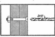
head until the shank is reached, a fter which the bolt can be driven
