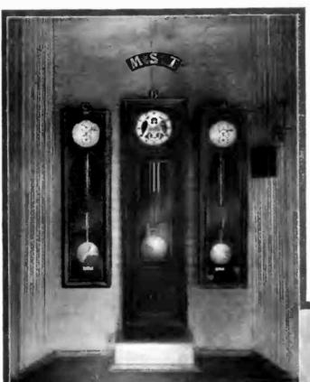
Above: Clocks Governing the Seismographs at Georgetown University. At the Right: The Seismographs that Stand on Concrete Piers that Reach Downward to Bed Rock,
