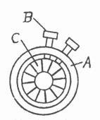
up against the shoulder on the sliaft, wrap a 3/8-inch wide piece of mica around the shaft up against the ring, and put the commutator in place. put the second ring on and turn on the nut, 12.—Ring for tightening the commu-Holding Commutator, tator in place. Direct the flame of a blow pot
