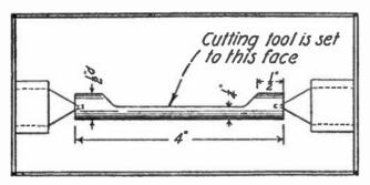
either end and milled down to exactly half its diameter as shown in the drawing. The rod is placed between lathe centers and the tool set to the height of the milled portion.
