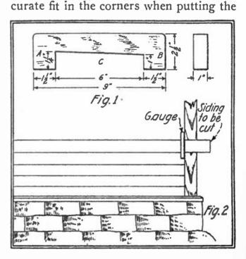
siding on a house, is readily made by the carpenter. A piece of wood is cut as shown in Fig. 1, which shows the utter simplicity of the device. In use, the parts marked A and B rest against the upright corner board of the house, allowing the piece of siding to be cut to pass through the open part C, as in Fig. 2. The piece is then marked with pencil or knife.
