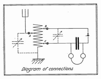
Wiring Diagram for the Tapped Three-Slide Tuner.
