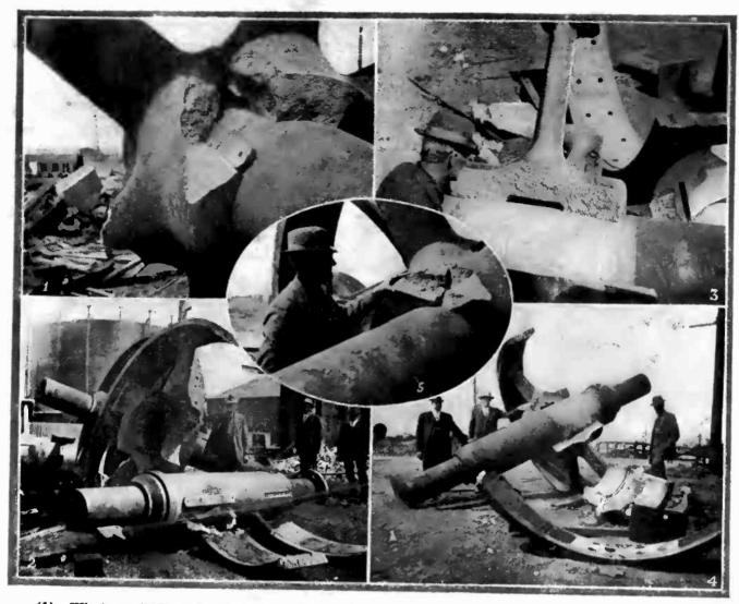
(1)—What an ineffectual discharge of dynamite dld to the hub of a big steel wheel. (2)—Another view of the same wheel after being shattered by the dynamite discharge placed at the hub. (3)—Remarkable straight fracture of the cast steel wheel at the hub, caused on the opposite side to where the dynamite was inserted. (4)—Another view of the steel wheel and its shaft. (5)—An unsuccessful attempt to shatter the wheel by a dynamite blast.
