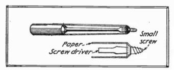
tion. After the screw is started, tear the paper away.
