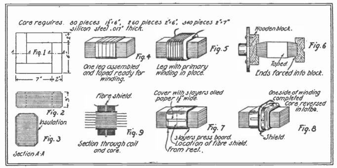
each and these strips are assembled alternately with the ends overlapping two inches. The 1½ by 6 inch strips are next divided into four piles of twenty each and these are assembled alternately also. These packs are then to be placed above and below the assembled piles as shown in Fig. 3 to break the sharp corners. The piles are then wound tightly with tape and finally covered with several layers of pressboard, preparatory to winding the primary and secondary.
