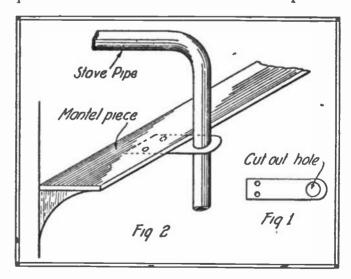
its place a holder that is neater and stronger. The holder is merely a piece of stove pipe iron cut to the shape indicated in Fig. 1 and having the holes as shown in the drawing. Fig. 2 shows the method of fastening the holder to a mantelpiece; obviously, by bending over the end containing the nail holes, the support may be fastened directly to the wall.
