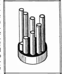
Place a rubber band around the disc and then drill a row of 3% inch holes around the edge as shown in the illustration. In each hole insert a piece of brass tubing, starting with a piece one inch long and making each succeeding piece ½ inch longer until five pieces are in place. Then start with another one inch piece in the opposite half of the disc and continue as before. When finished, the device is pushed down inside the horn, the rubber band on the edge of the disc holding it in place.
