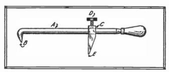
steel  $\frac{1}{4}$  inch thick,  $\frac{3}{8}$  inch wide and one inch long, sharpened to a cutting edge at E. A hole is drilled to pass the  $\frac{1}{4}$  inch rod and in the top of the cutter another hole is drilled and tapped for the set screw D. A handle fitted to
