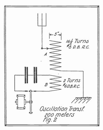
Connections for an Oscillation Transformer, Condenser and Rotary Gap.
