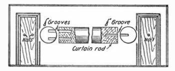
grooves cut into the end grain, as shown. The rod is prepared by cutting it to a length that will make it a snug fit between the door jambs. The slots are then cut, two being placed in one end and one in the other end of the rod. Headless nails are driven in the door jamb on either side to take the slots and the support is finished.
