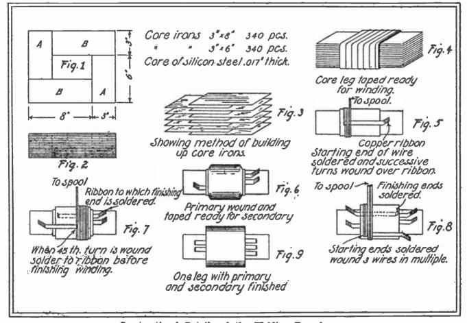
In order to make the description clearer, the various parts of the transformer will be described separately, each under its proper head-The transformer is designed for operation on a 110-volt, 60-cycle alternating current circuit and when the load is applied, the current in the primary is approximately 26 amperes. The secondary current at 11 volts is in the neighborhood of 250 amperes and this is sufficiently large to make quite a display.
