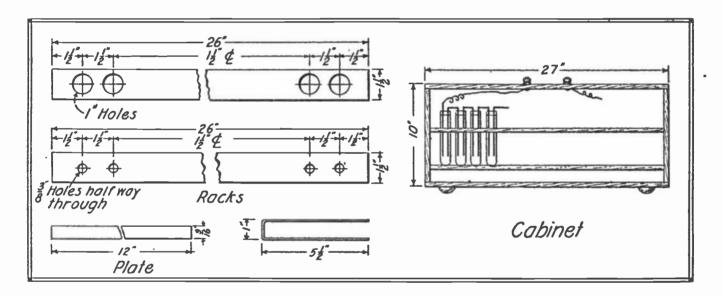
A containing cabinet is now constructed from ½ inch oak measuring overall 27 inches in length, 10 inches in height and 9½ inches in width. Brass screws should be used throughout the work to avoid the corrosive effect of the battery solution. The interior of the cabinet should be coated with lampblack or a similar acid resistant.
