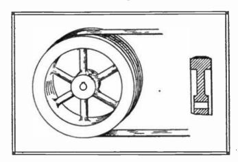
oughly shellacked and when the varnish had dried, the wheel was given a test which quickly proved the scheme to be practicable. At the end of the season the tape was found to be but slightly worn. During the entire run the belt did not once leave the fly wheel.
