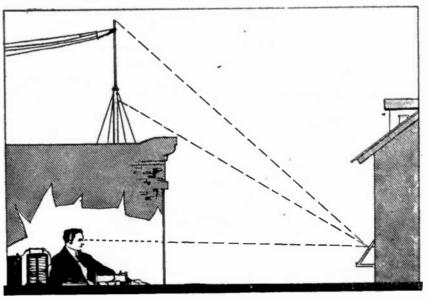
Without Leaving His Seat, an Amateur Operator Can See His Aerial by Means of a Simple Mirror Device.
