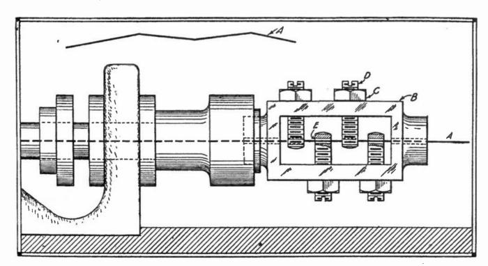
the end of the rod completes the can opener. In use, the pointed end of the rod is inserted through the top of the can, while the cutter, which has been set to the desired radius, is carried around with some pressure on the handle.
