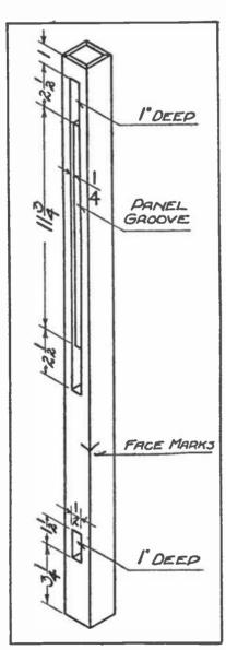
Fig. 1.—Detail of Inside Corner of Leg.
