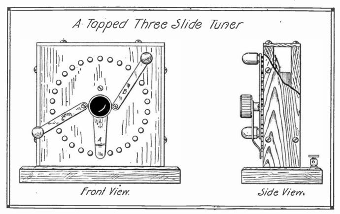
Front and Side Views of a Tapped Three-Slide Tuner as it Appears When Completed.
