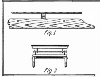
occasioned where the sleigh is fastened to the plank. Very often the bobs are broken at this point because it cannot give enough.
