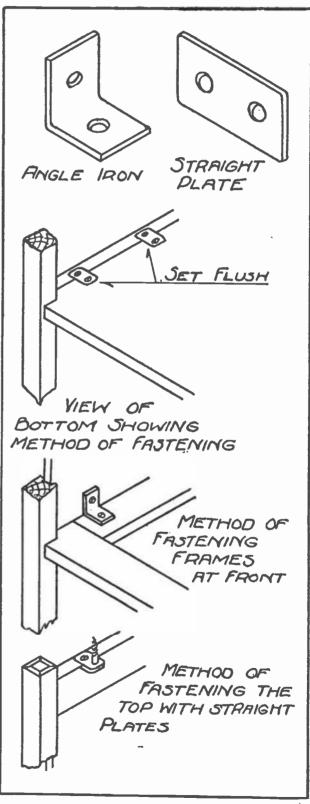
Fig. 3.—Methods of Fastening the Different Members,
