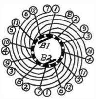
Fig. 15.—Scheme for Connecting Armature Windings to
