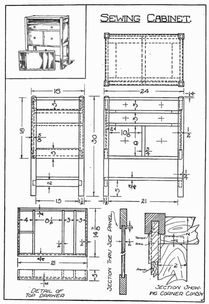
General Details of the Sewing Cabinet as Well as a View of this Piece of Furniture When Completed, with One of the Drawers Removed.
