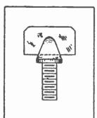
placing the lost set screw of a binding post, etc., may be made from the zinc terminal of a dry cell. The terminal is removed from the cell and a piece of brass, cut to the s h a p e shown in the illustra-
