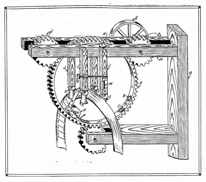
wood. On the inner rim of the large gear is fastened a spool carrying the cloth wrapper. The tire is supported between rollers, K, K, K and L, placed at the extremities of four wooden pieces, J. The roller, L, turns on a shaft, M, which passes through the wooden sup-
