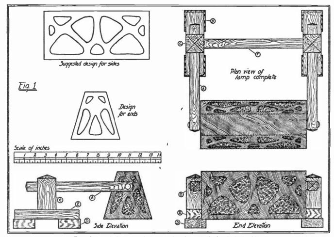
Drawings of Completed Lamp showing Method of Assembling.
