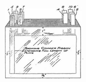
Fig. 1.—View of Glass Condenser Plates Assembled.
