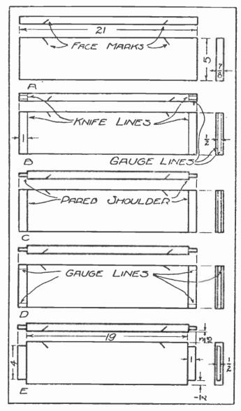
Fig. 1.—Methods of Cutting the Tenons on Chair Ratle.
