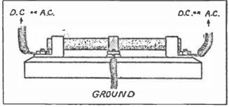
Graphite Rod and Connections for Protecting Power Lines.
