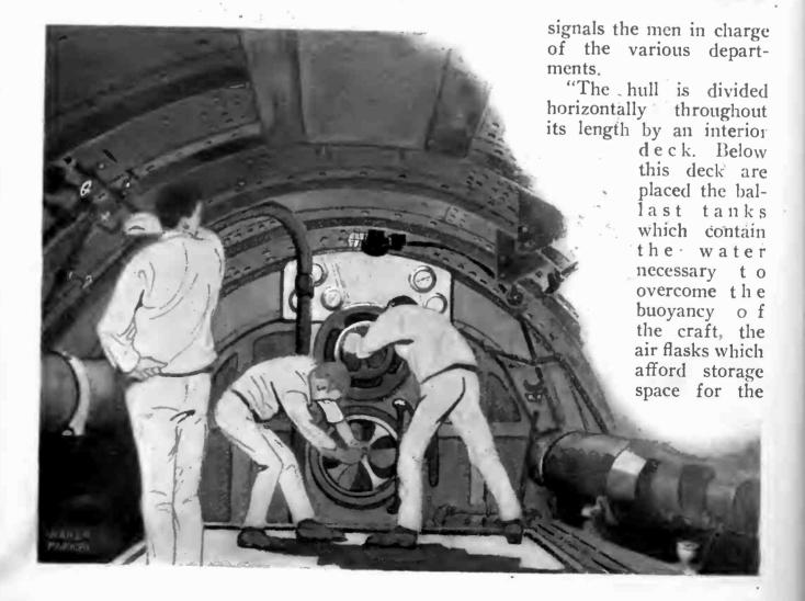
air used in emptying the ballast tanks, firing the torpedoes, and in maintaining a constant supply of fresh air for breathing purposes; the storage battery, which furnishes the electric current used in propelling the craft under water; and the oil tanks for the storage of the crude oil fuel for the Diesel engines used for surface propulsion.
