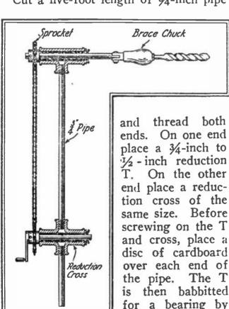
on a paper pad and standing a ½-inch diameter steel shaft upright in it. The babbitt cannot escape as it is poured in around the shaft because of the disc closing the end of the pipe. A two-foot length of pipe is in-
