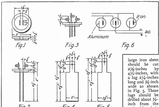
Fig. 2 Fig. 4 Fig. 5 ance, thereby greatly increasing the efficiency. It will furnish 80 to 90 volts D. C. and will carry as high as 5 amperes on intermittent service. By doubling the
