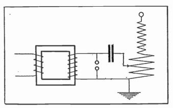
Fig. 15.—Diagram of an Oscillatory Circuit.
