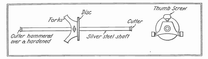
ters being also provided on the shaft. A pattern is required for the head—a useful lesson in small pattern making—and if the cutters are properly hardened the gauge may be used for marking metal as well as wood.
