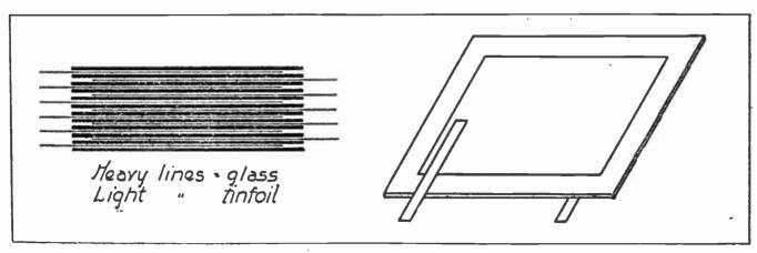
Showing Method of Assembling Plates of Condenser with Lugs Projecting. Also View of Single Plate of Glass with Tinfoil in Position.
