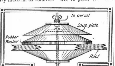
Diagram of Inexpensive Roof Insulator.
