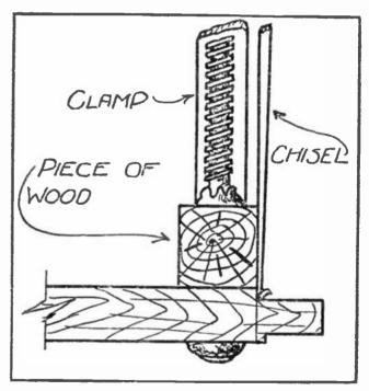
Fig 8.—Suggestion for Chiseling Sharp Corner on
