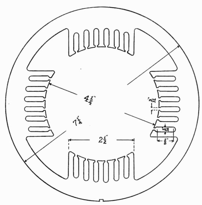
Fig. 45.-Field Punching for Compensated Series Motor.
