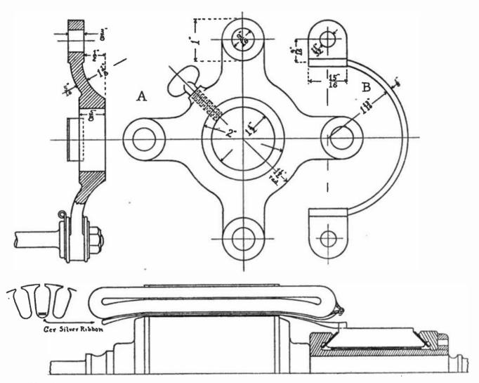
Fig. 47.—Details of Brush-holder Yoke, Cross Connector and Commutator Resistance Leads.
