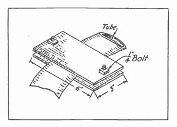
3 by 6 inch pieces of iron as shown in the accompanying sketch. The holes in the under piece should be a snug fit for the shoulder of the bolts, while those in the upper piece should be an easy clearance fit. It is preferable to employ wing buts on the ends of the bolts in order that no wrench may be necessary for tightening.
