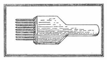
corners with a knife or file. Drive a row of ten penny finishing nails into the end of the broad part near enough together to let the shank of a six or eight penny nail enter, but not far enough apart to permit the heads to pass through. File the heads of the nails down to points.
