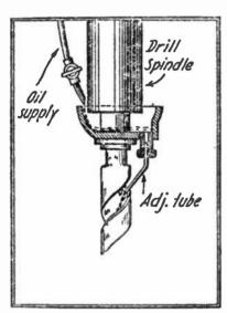
found around the shop. The main part is the oil cup. In this case the steam chamber from an old 11/4 - inch steam whistle wasemployed. threads were bored out and the hole tapered to slide
