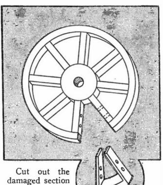
Cut out the damaged section between spokes with a hack saw and drill two holes in each
