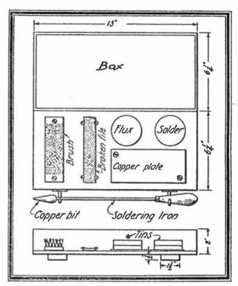
dinary fire or gas flame. Do not buy a very small iron, for it will not retain the heat. When soldering in awkward places the solder should be cut up in small pieces with shears, or scissors if no one is looking, and after fluxing the place to be soldered, putting several bits of solder in position ready for running with the heated iron.
