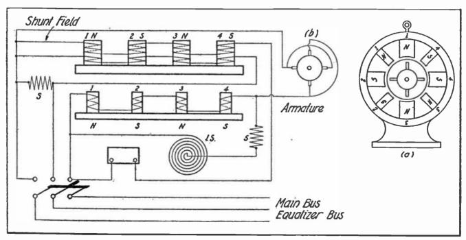
Wiring Scheme for an Interpole Dynamo.
