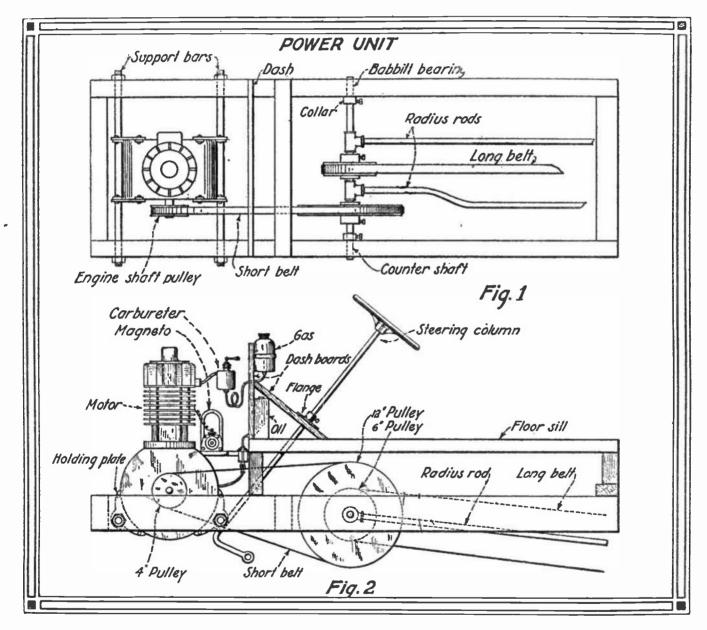
cters are based upon the assumption that the motor is capable of developing between four and five horsepower, which is the average performance of motors of this type. The belt pulley on the engine crankshaft is four inches in diameter and it drives to a pulley 12 inches in diameter; the ratio is obviously 3 to
