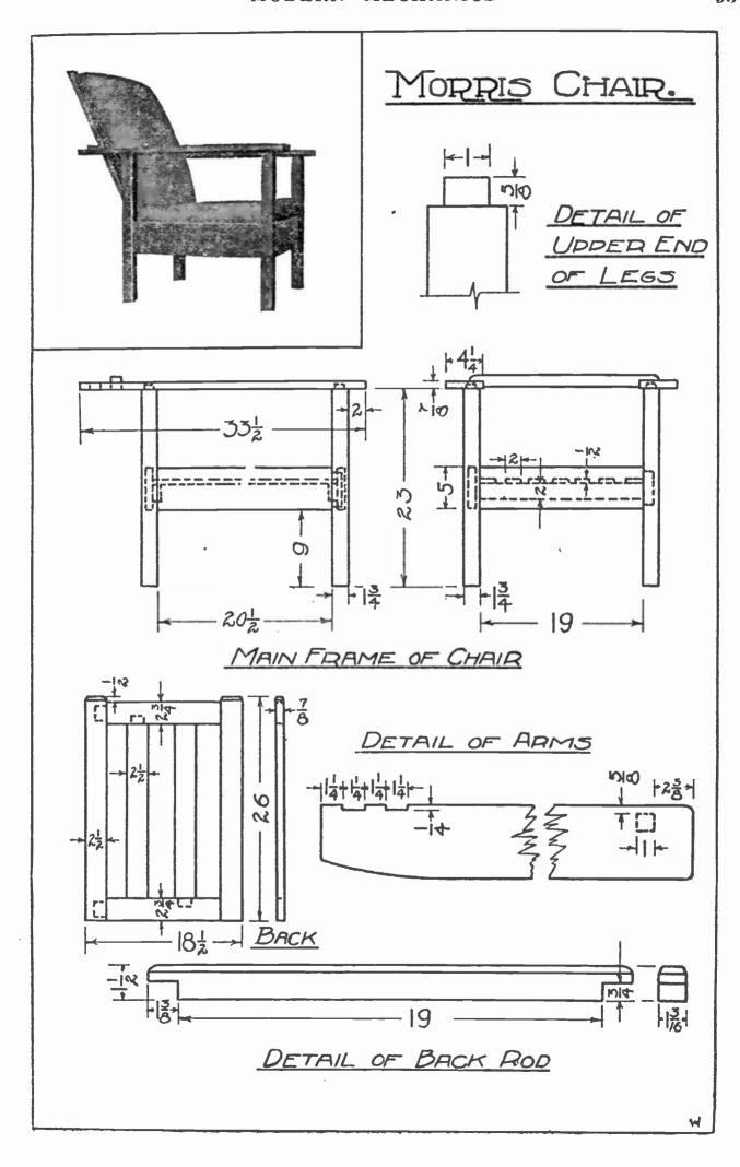
per ends of the legs. Notice the detail on the drawing. To do this, be very sure that you measure up 23" from the bottom ends of the legs, rather than 5%" down from the top. Cut these tenons
