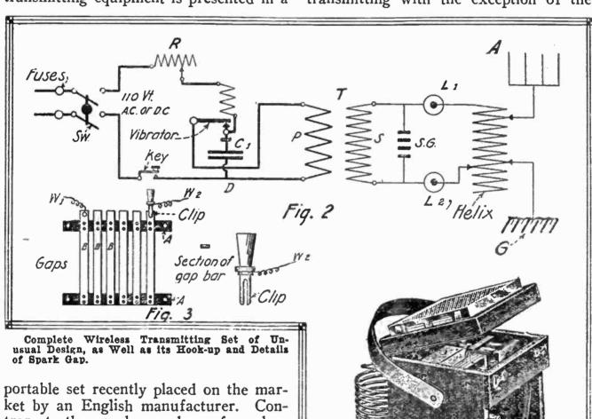
portable set recently placed on the market by an English manufacturer. Contrary to the usual procedure of employing a transformer or some form of electrolytic or motor interrupter for operating on either alternating or direct current circuits, this set has adopted an ingenious principle that enables it to be employed on either kind of current and on frequencies varying from 40 to 100.
