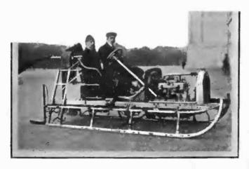
Sled Driven by Aerial Propeller, Capable of Developing High Speed.
