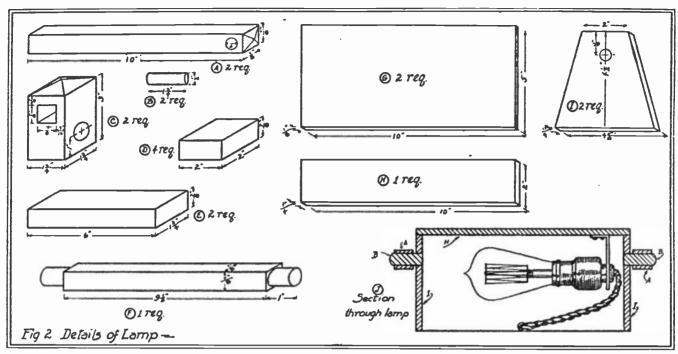
Details of Parts of Piano Lamp.
