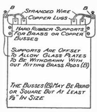
Fig. 8.—Method of Making Connections with Lugs.
