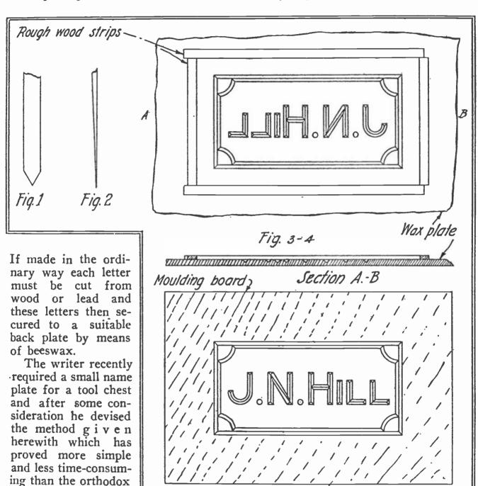
means it requires no special tools. A little thought will show the reader that if letters were cut backwards and deeply into a flat surface of wax and a plaster cast of this then made, the lettering will be raised and in the right direction. Care is of course needed
