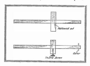
ture of a little time and trouble. The improvement consists simply in cutting a hollow out of the face of the head as shown in the drawing. The gauge may
