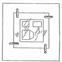
with a piece of the thin wood used on the backs of picture frames and the two held together by means of four clothespins. The negative or tracing and the blue-print paper are placed face to face and held in close contact between the glass and the wood. When it is desired to examine the print in order to determine when correct exposure has been given, one clothespin may be removed and a corner of the wood lifted up without fear of getting the paper and tracing out of register.
