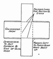
Fig. 2.-Pattern for Condenser Tank.
