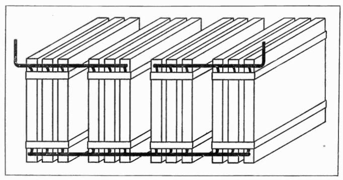
Complete Condenser, Showing Method of Connecting.
