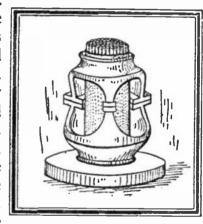
from a disc of wood and the various parts assembled with glue. The wooden roller is of course removed in order that matches may be placed inside the tube of sandpaper. When the glue is dry the holder may be filled with matches and it is obvious that they are to be scratched on the wall of the sandpaper tube through the openings between the legs of the gas mantle holders.
