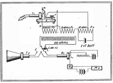
Wiring Diagram of New Wireless Recording Apparatus.
