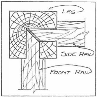
Fig. 4 .- Mortises in Legs of Chair to Hold Tenons.
