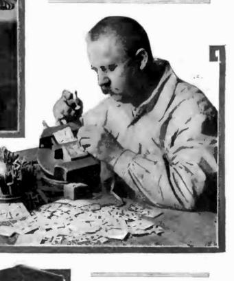
Using a scroll saw in order to cut out from a silver sheet the silver edge of the Iron Cross. Previously, the silver squares have been punched to shape.
