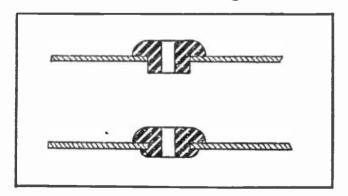
into hole in the canopy. Heat the threaded end with a match or candle, which will quickly soften the rubber. Before it hardens press out edges with the thumb, thus forming a shoulder and locking the bushing.
