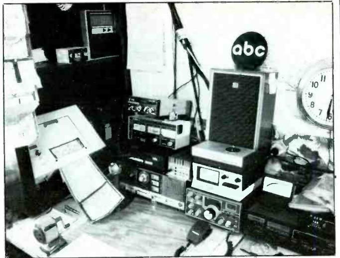
*Weather FAX (left) is ideal for Tropo checking and tracking.*
