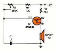
Fig. 9. This audio oscillator is another R/C-type circuit that gets the work done with a UJT (uni-junction transistor).
