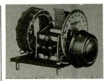
One of the three tuned circuits in a Freshman Masterpiece five-tuber. The coil was deliberately mounted on a variable capacitor frame to create losses (see text).
