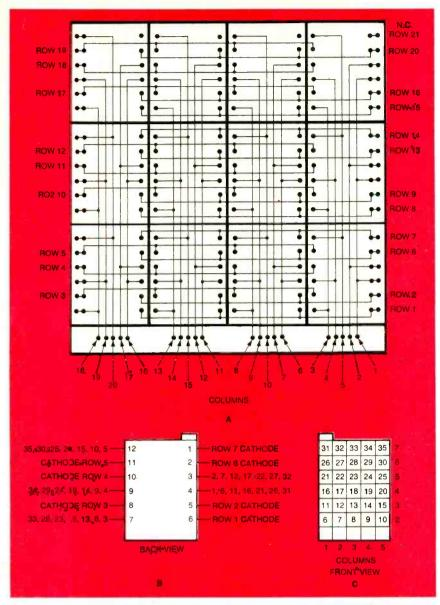
Fig. 5. Once you've etched your board, install the parts guided by this parts-placement diagram. Install the jumper connections first, as at least four of them must run beneath the IC sockets for U3 and U4.
