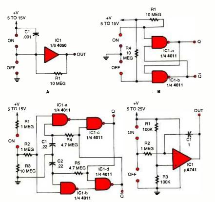
Fig. 7. Author's first touch circuit is shown in A. Next one (B) is a configured flip-flop using a 4011 chip. In C, the author uses one touch-off/touch-on pushbutton. In D, the circuit uses an opamp for switching action.
