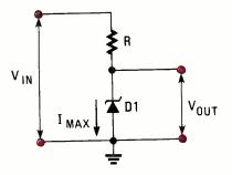
Fig. 3. Zener diodes make excellent voltage regulators.
