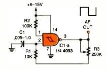
Fig. 8. Here's another square-wave oscillator that uses a CMOS IC with input hysteresis. In this R/C oscillator circuit, a single gate of a quad 2-input NAND Schmitt trigger IC is the active element.
