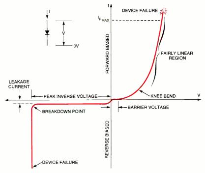
Fig. 2. Here's the characteristic curve of current through a standard diode vs. the voltage applied across it.
