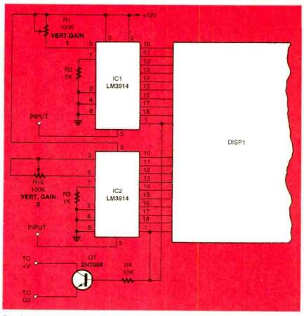
Fig. 2. By altering the input of the Solid-State LED Oscilloscope, as shown here, the singe-trace circuit illustrated in Fig. 1 can be converted to a dual-trace unit. Other modifications are possible as well (see text for details).
