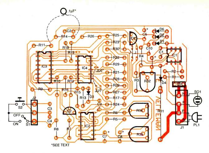
Fig. 4. Assemble the Soft Switch's printed-circuit board according the this parts-placement diagram. Note the components marked with an asterisk. Those components are either included in or left out of the circuit depending on the mode of operation that you are configuring your circuit for.
