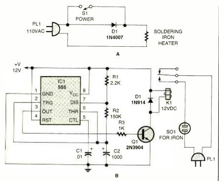
Fig. 9. A budget diode dimmer circuit (A) can be used to protect the tip of a soldering iron when not is constant use. The circuit in B builds in a timing sequence that may be more useful to the person who solders.
