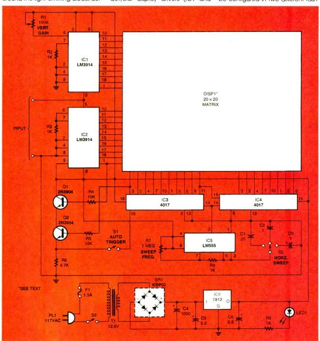
Fig. I. The Solid-State LED Oscilloscope is built around six IC's and twelve 5×7 LED arrays that are arranged to form a 20 × 20 LED display matrix. Two of the the chips, IC1 and IC2, form the vertical circuit, while the horizontal circuit is formed by two more
