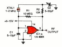
Fig. 6. This single CMOS 2-input NOR gate crystal oscillator circuit has one major limitation; it lacks high frequency performance, otherwise, it is a solid performer.
