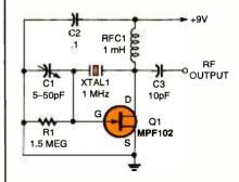
Fig. 3. A simple Pierce crystal-controlled oscillator circuit can be used as a marker generator for receiver tuning alignment.
