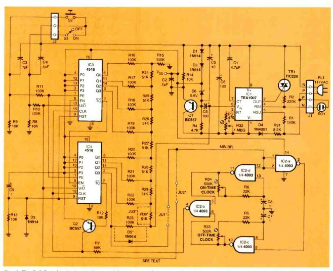
Fig. 1. The Soft Switch, which is built around four integrated circuits, a few diodes, and a Triac, uses two simple oscillator circuits to provide independently adjustable gradual on and gradual off times.
