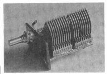
Fig. 6. The Jackson Brothers LAIIxxx dual airdielectric variable capacitor is used in lowpower (QRP) and receiver antenna-tuning units and elsewhere.
