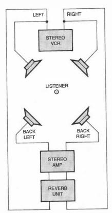
Fig. 4. If you would like to set the unit up for surround effects, feed it a stereo signal and amplify the resulting output with a stereo amplifier.
