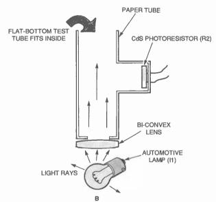
Fig. 4. This turbidimeter circuit (A) will let you measure or monitor the clarity of water. A simple optical assembly (B) lets light reflected by particles in a water sample hit a photoresistor, varying its resistance.
