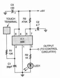
Fig. 4. Simply touching the "touch terminal" will activate the switch and keep it on for a duration set by R3 and C2.
