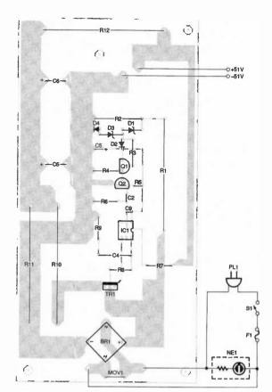
Fig. 6. Here's the parts-placement diagram for the power-supply board.
