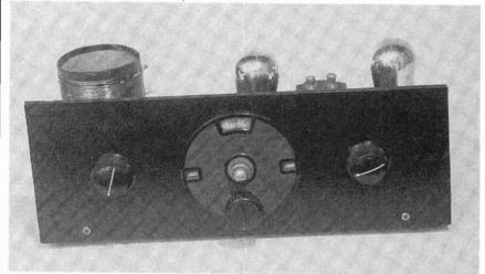
Here's the front of 1930's ham receiver complete and ready for testing. Note the Marco three-window dial (see text).
