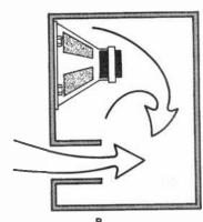
Fig. 1. Here's how the vent works in a bass-reflex speaker. The situation above the resonance frequency is shown in A, while B shows the situation below resonance.
