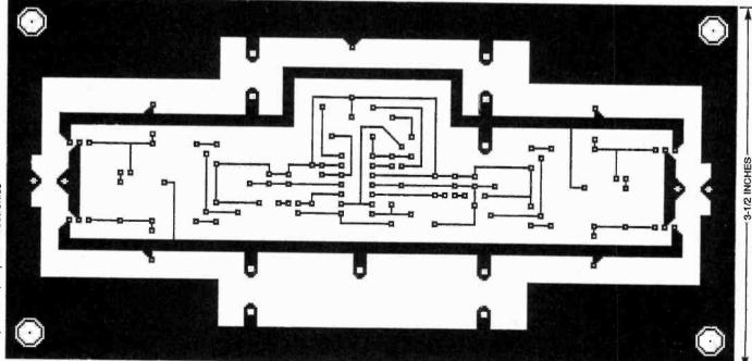
Fig. 3. Here's the full-size foil pattern for the Amplifier circuit board.
