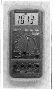
The Rangemaster II features 45 ranges and 11 functions that include voltage, current, resistance, frequency, capacitance, and logic, with very wide ranges and high resolution. The range for DC voltage is 200 mV to 1000 volts (0.6% basic accuracy); AC voltage is 200 mV · to 750 volts (1.2%); DC/AC current is 20 μA to 20 amps (0.8% and 1.2%, respectively); resistance is 200 ohms to 200 megohms (0.8%); capacitance is 2 nF to 200 µF (3%); and frequency counter is 2 kHz to 20 MHz (1%).
