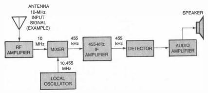
Fig. 1. The basic, single-conversion receiver, shown here, combines the incoming signal with the local-oscillator (LO) signal to produce the intermediate frequency (IF) signal. The resultant IF signal then is converted to audio by the set's detector stage.
