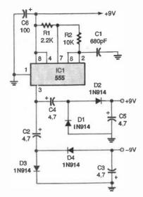
Fig. 5. This dual-polarity power supply is ideal for use with op-amps and in many other applications
