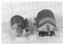
Fig. 5. The capacitor on the left in this photo is called a straight-line frequency model, while the one on the right is a straight-line capacitance model.
