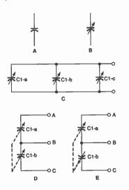
Fig. 1. These symbols are commonly used to designate a variety of fixed and variable capacitors.
